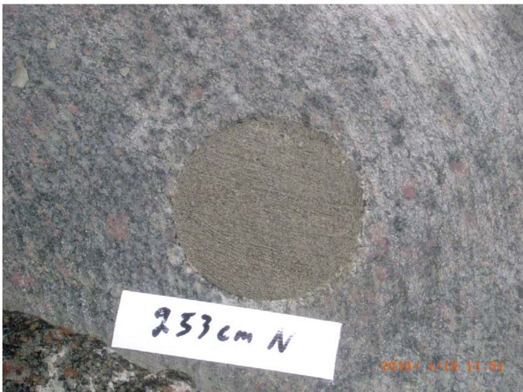
Figure 5-3. Examples of sections. Upper: Clay plug (base of Disc 5). Lower: The CBI-concrete seal (base of Disc 7). Both the clay and the concrete had completely filled the hole.
