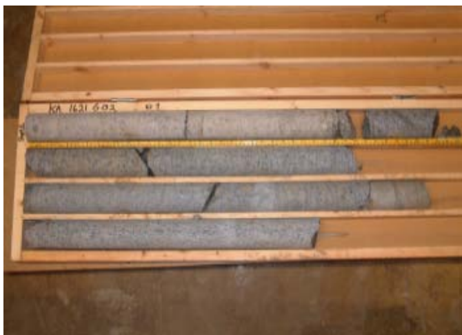
Figure 2-1. Hole KA 1621 G02. The core from the 80 mm-diameter hole represents the uppermost 3 meters of the hole having at least five water-bearing fractures.
