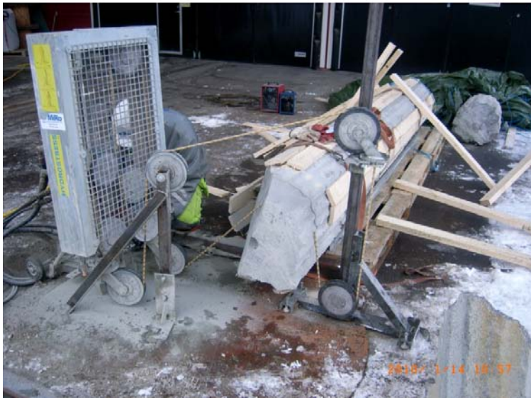
Figure 5-1. The rock column containing the plugged borehole KA 1621 G02. Upper: Slot drilling. Lower: Wire sawing of discs with about 100 mm thickness.
