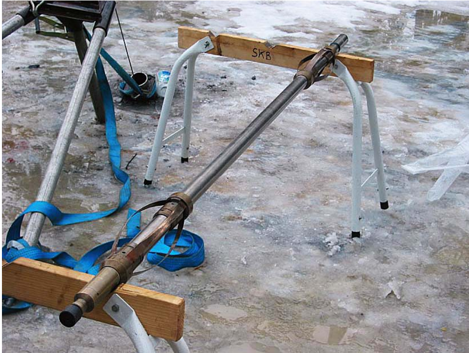
Figure 3-14. The HiRAT probe used for acoustic televiewer logging. The probe is centralized in the borehole with two bow spring centralizers (Ringgaard 2007).
