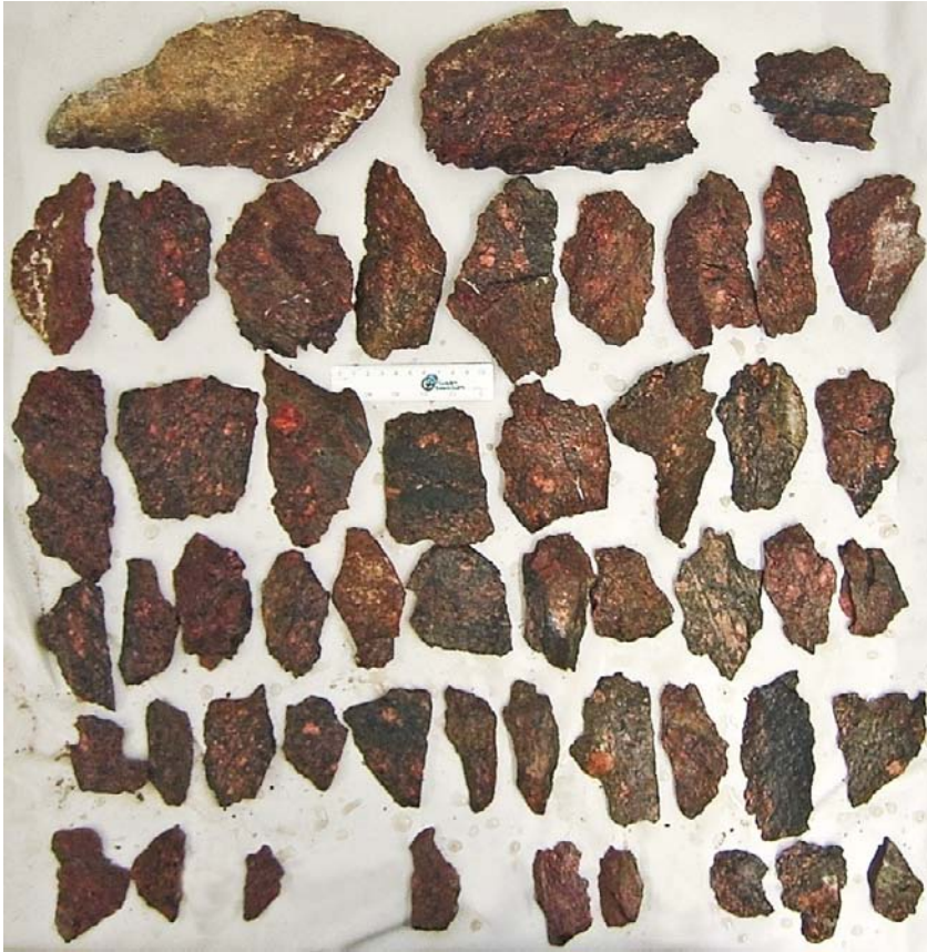
Figure 3-30. The larger fragments collected from a heated borehole (450 mm) CAPS Test 1, shown here for comparison of the shape to the fragments collected in the slim borehole (75 mm) of SLITS (Figure 3-28). The scale in the centre of the image is 10 cm long (Glamheden et al. 2010).
