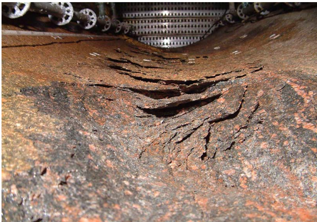
Figure 1-3. Photograph taken from below of chips forming at 3.7 m depth in the 1.75 m diameter vertical borehole of the Äspö Pillar Stability Experiment (APSE) site. Note the fairly consistent orientation of the centre, deepest points, of the wedge shaped spalls in the borehole periphery. This spalling was induced by heating in the pillar next to the large diameter borehole. From Andersson (2007).
