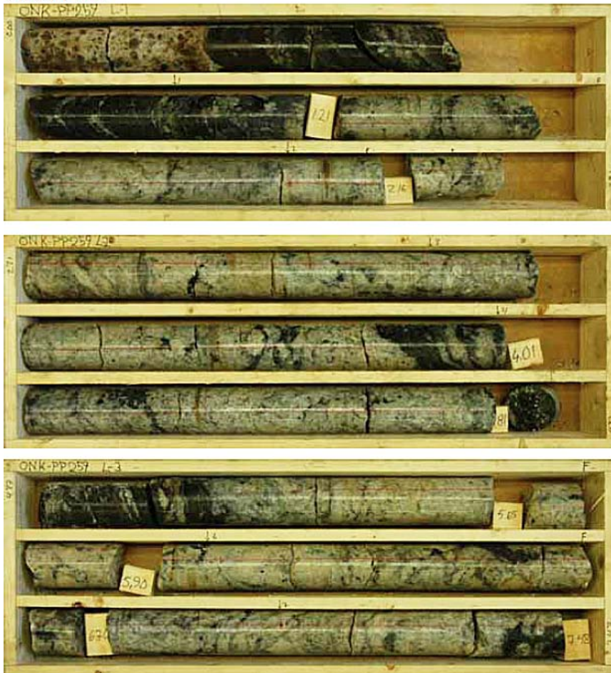
Figure 4-3. Drill core from the borehole (ONK-PP259) used for the pilot SLITS test at ONKALO. The diameter of the core is 83.7 mm (while the diameter of the borehole is 101.3 mm). The upper box includes cores down to 2.31 m depth, the middle box to 4.87 m and the lower box down to the end of hole at 7.48 m depth. The first 0.34 m is concrete in the tunnel floor. (Toropainen 2010).
