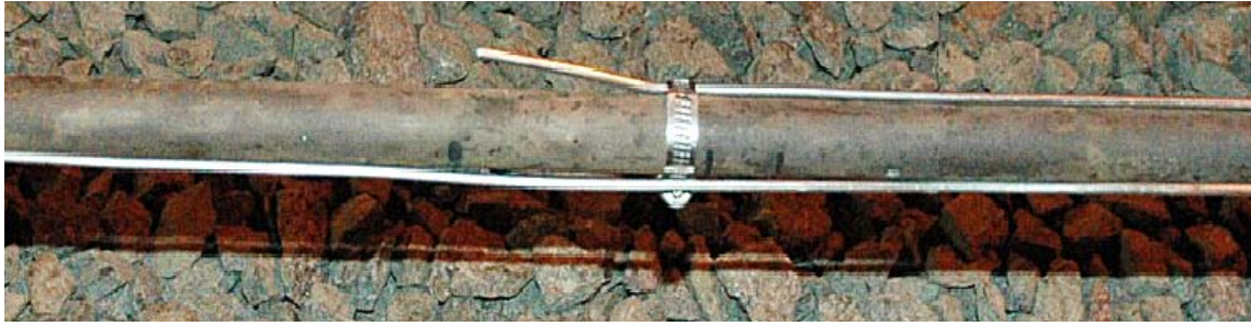
Figure 3-12. Close-up of the heater at the temperature gauge. This gauge is located at a distance of about 1 cm from the heater; i.e. in the gap between the heater and the borehole wall not leaning against the wall. This gauge was located at the bottom of the heated section (T01).
