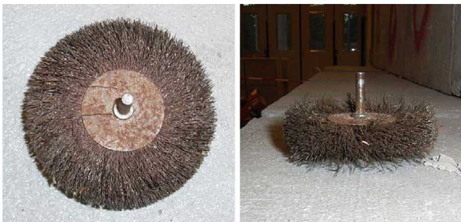
Figure 3-16. Brush used after heating periods to loosen any thermally spalled rock in the borehole wall.
