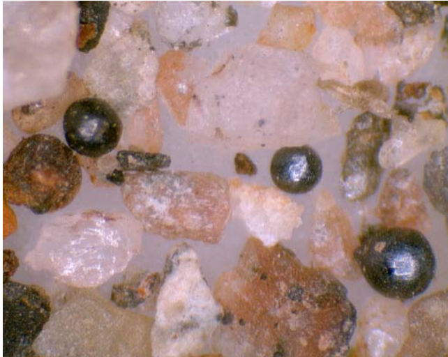
Figure 3-32. Close-up image of typical small fragments collected. Three spheres of asphaltite. The image is about 1.5 mm wide.
