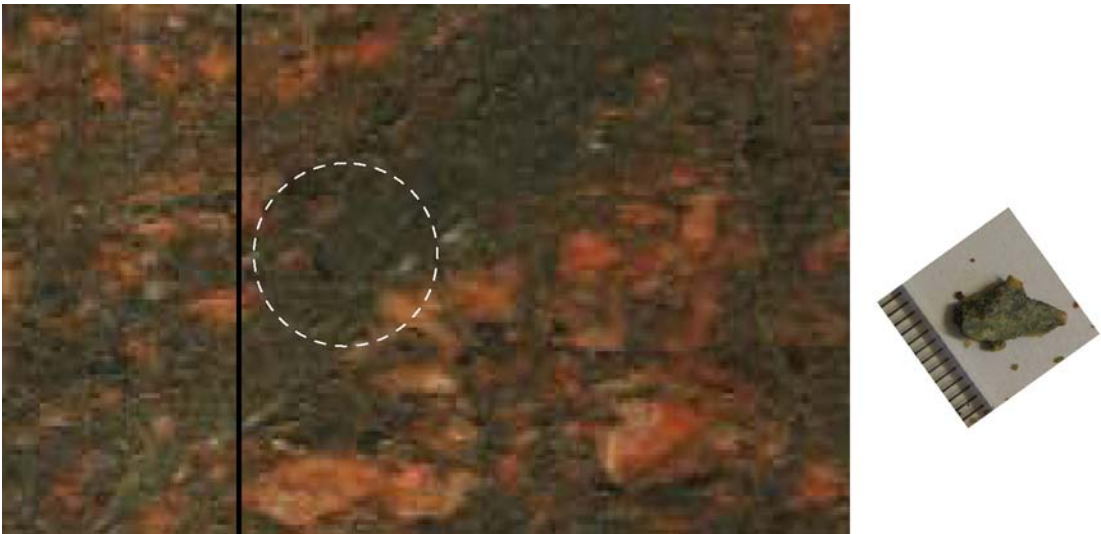
Figure 3-29. For one of the fragments collected it seems that the shape and size fits with the place where we found a missing piece in the logging results. The left image is the optical logger result from after the third heating and the right image is the mirror image of the fragment, for comparison.
