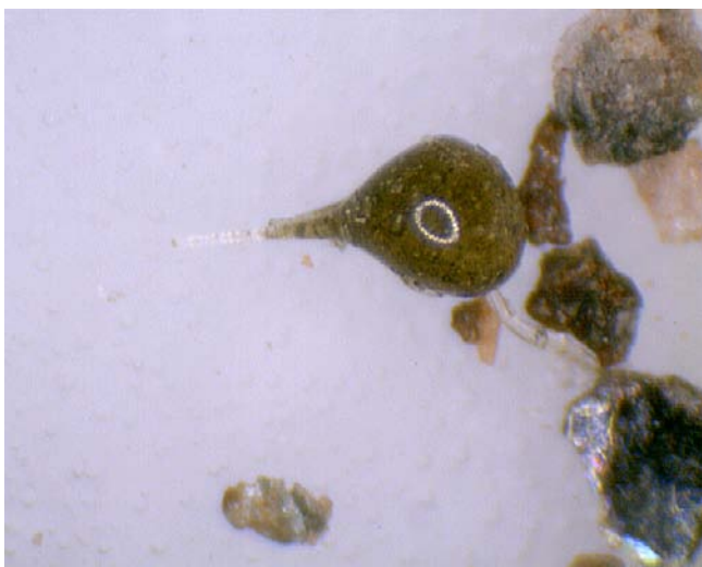
Figure 3-34. Example of asphaltite collected among the fragments after the last heating. The particle is transparent and having drop shape. The image is ca 1.5 mm wide.
