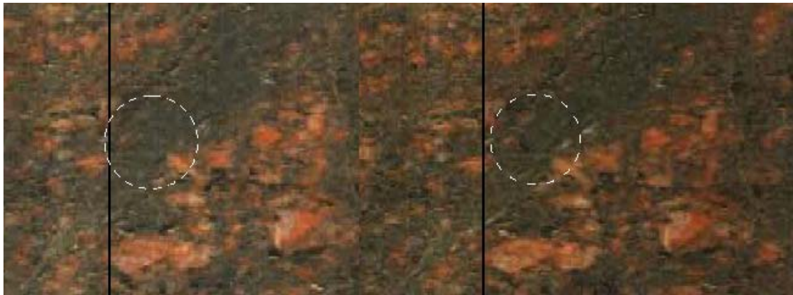
Figure 3-27. The same location as shown in Figure 3-25 and Figure 3-26. The left image is the optical logger result from 30/8 after the second heating and the right image is from 9/9, after the third heating.
