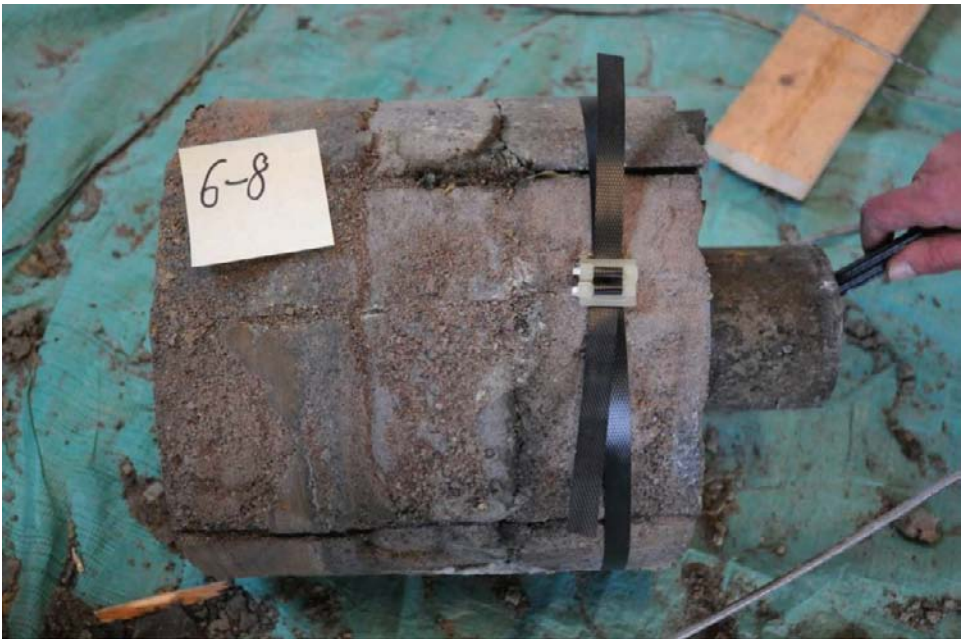
Figure 5-9. Some blocks were very fragile and in order to keep them together during the cutting, they were supported by plastic straps.
