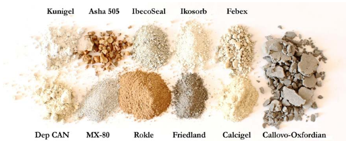
Figure 3-1. Photo showing the different materials in the ABM test.
