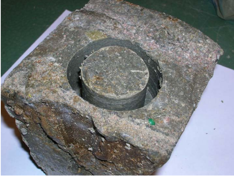
Figure 6-13. Preparation of samples for measuring the swelling pressure and the hydraulic conductivity. The samples were drilled out and then sawn out from the block pieces.
