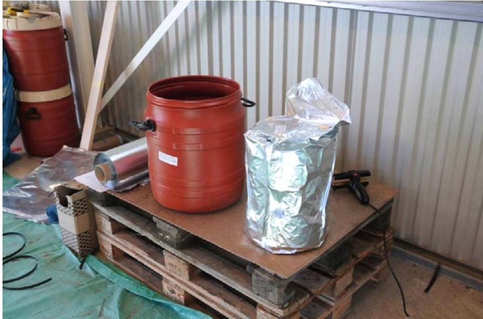
Figure 5-10. The parcels containing bentonite blocks were placed in sacks of alumina laminate which were evacuated welded together and then placed in air tight barrels.
