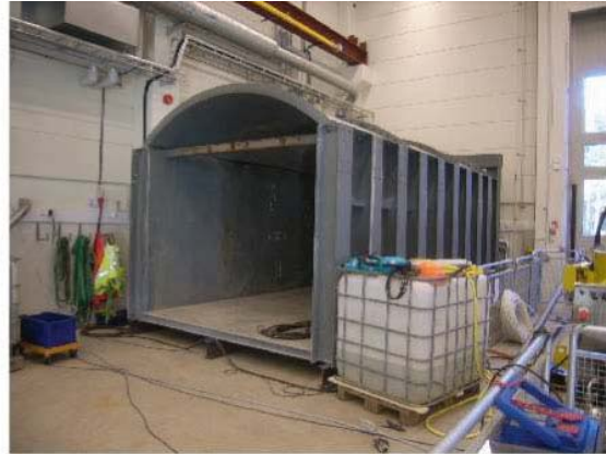
Figure 2-1. 1/2-scale tunnel simulator located in bentonite laboratory at Äspö (Dixon et al. 2008b).
