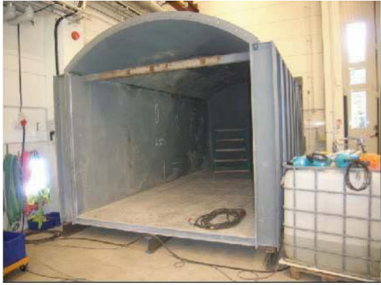
Figure 2-1. 1/2-scale tunnel simulator located in bentonite laboratory at Äspö (Dixon et al. 2008b).
