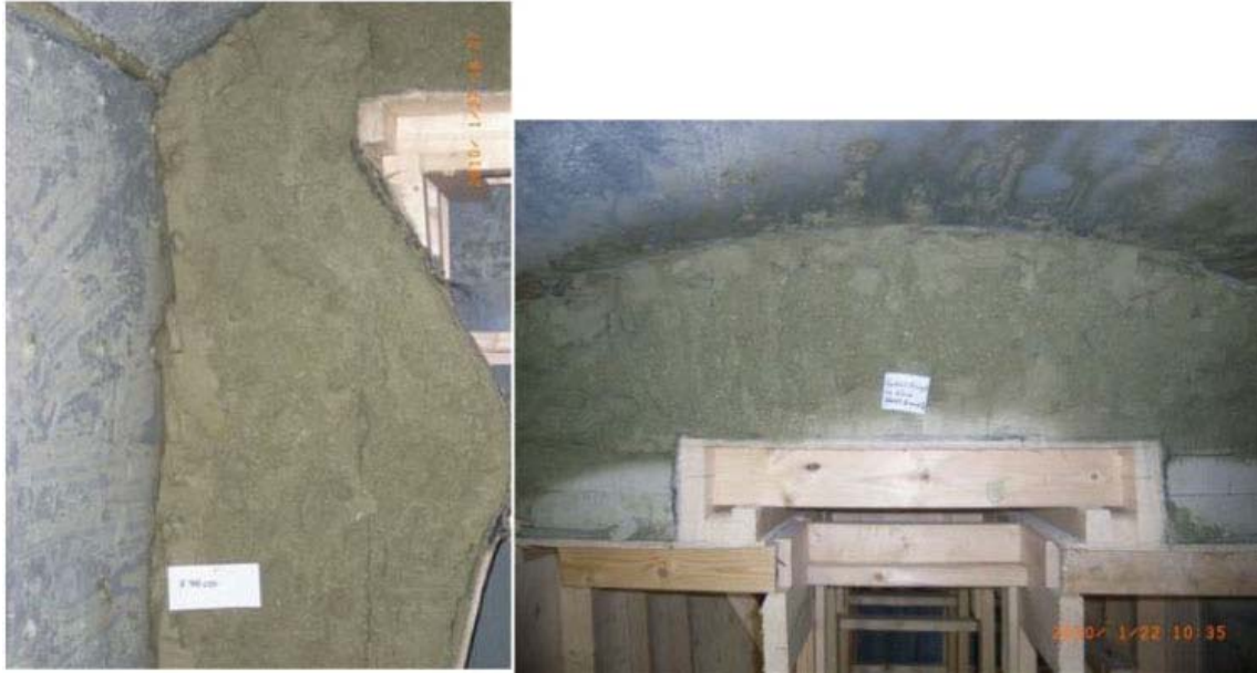
Figure 3-15. Homogenisation of clay blocks and pellets in Test 4. Left: location of formwork failure. Right: crown region behind fracture. The block-block and block-pellet contacts are not visible and considerable progress has been made towards homogenisation in these regions.
