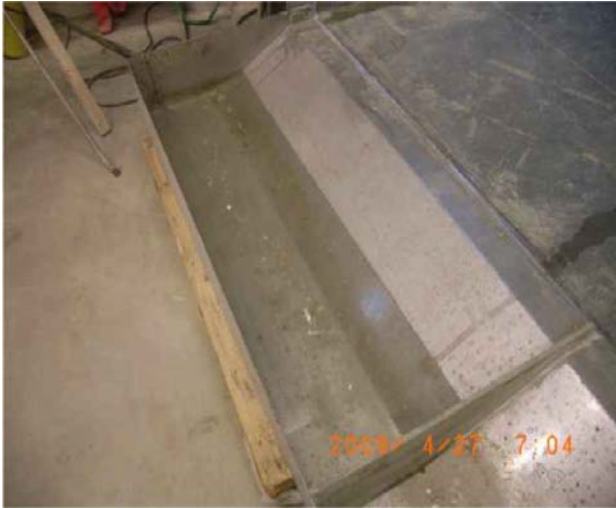
Figure 3-4. Water that exited Test 1. Water was clear and lacked discernible sediment.
