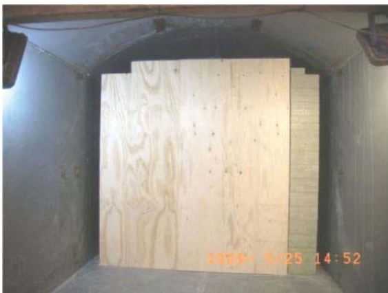
Figure 2-2. 1/2-scale simulation showing downstream face before and after pellet installation. Note the presence of blocks along right side only. Left side contains only 0.15 m thickness of pellet fill between geotextile inner liner and chamber wall.
