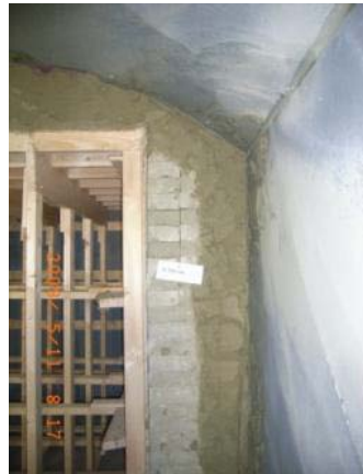
Wetting at location of artificial fracture resulted in gasket-like seal extending through first row of blocks.
