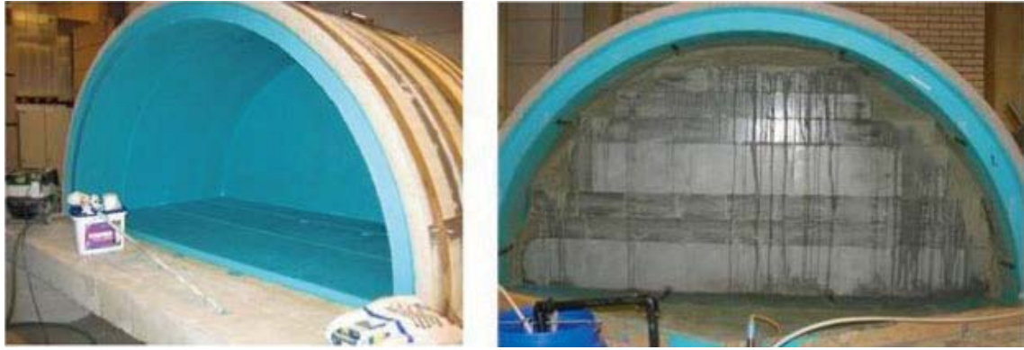
Figure 2-4. 1/4 Scale test cell and assembly at end-of-test (Ekokem tests in Finland (Riikonen 2009)). A similar setup was used for tests described by Dixon et al. (2008a).
