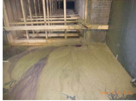
Pellet materials eroded from mock-up
