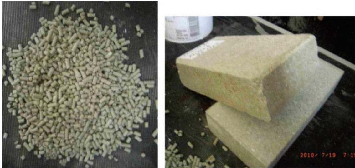
Figure 3-1. Photos showing pellets and blocks manufactured from Milos B bentonite.
