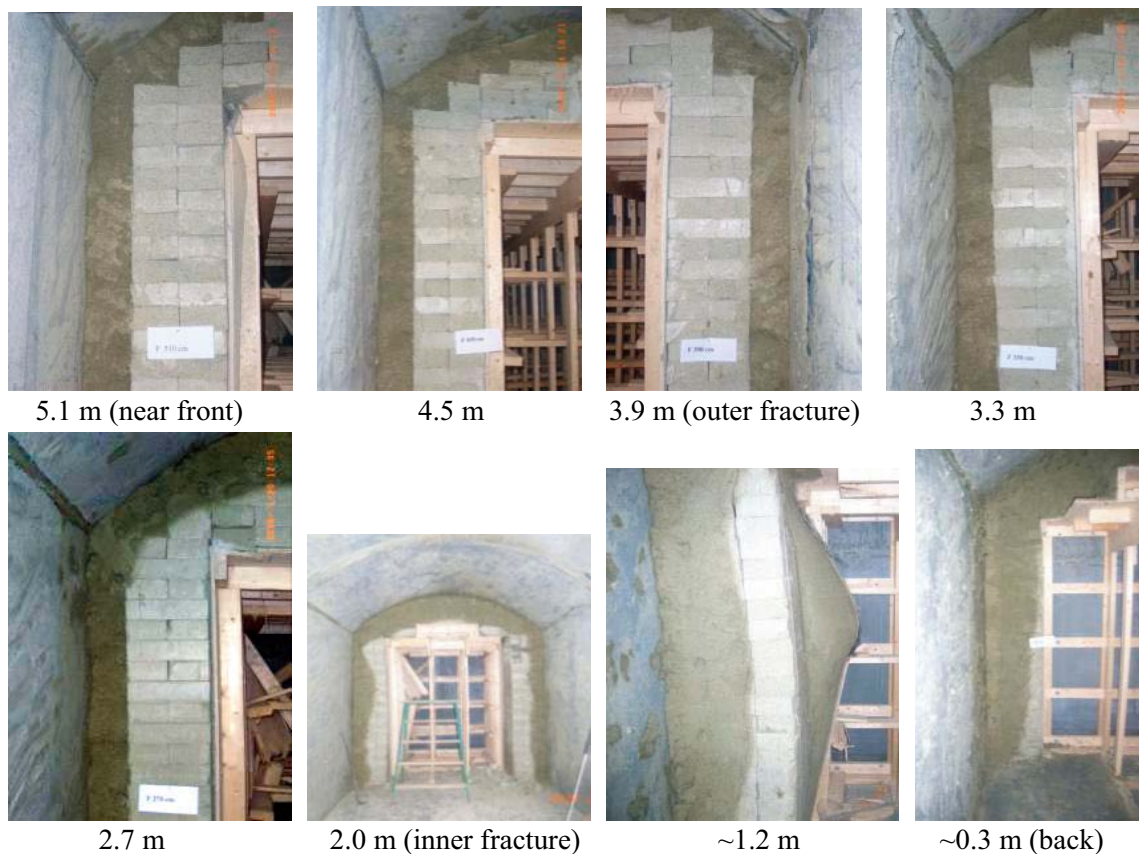
Figure 3-13. End-of-Test Water distribution within Test 4. Photos show extensive water retention and swelling in region behind inner fracture (~2 m), including mechanical failure of internal framework at ~1.2 m, limited wetting in region between fractures (2–4 m) and essentially unaltered regions downstream of outer fracture (excepting front face of assembly, wet by exiting water).
