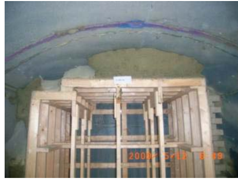
Artificial fracture at mid-point of Tests 1, 2 (coloured by dye)
