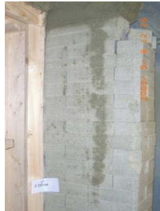
Wetting at location of artificial fracture resulted in gasket-like seal extending through first row of blocks.
