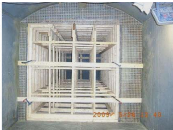
Figure 2-2. 1/2-scale simulation showing downstream face before and after pellet installation. Note the presence of blocks along right side only. Left side contains only 0.15 m thickness of pellet fill between geotextile inner liner and chamber wall.
