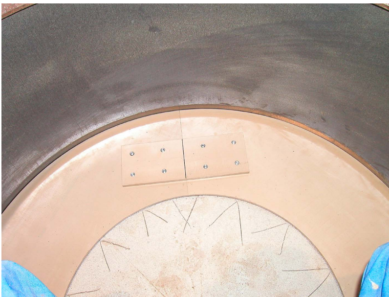
Figure 8-6. The PEEK ring placed on top of block C2.
