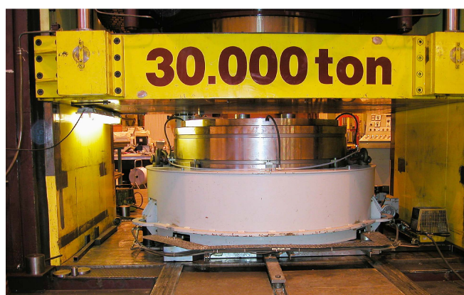
Figure 3-1. The mould placed in the press at Hydroweld AB in Ystad, Sweden.
