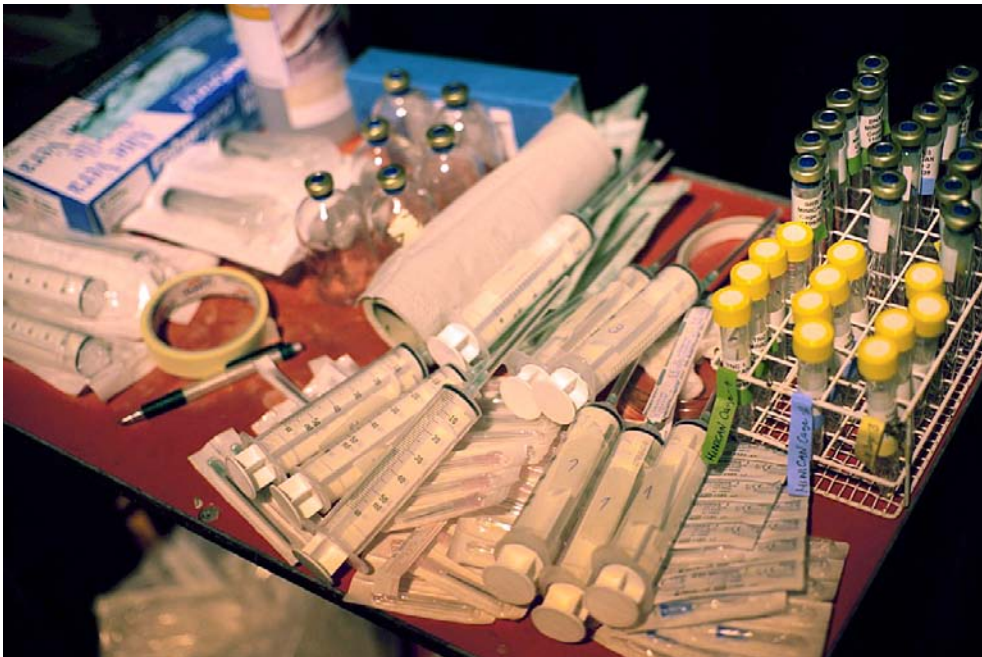
Figure 2-3. Material for sampling during the removal of the A04 canister in the MINICAN experiment.
