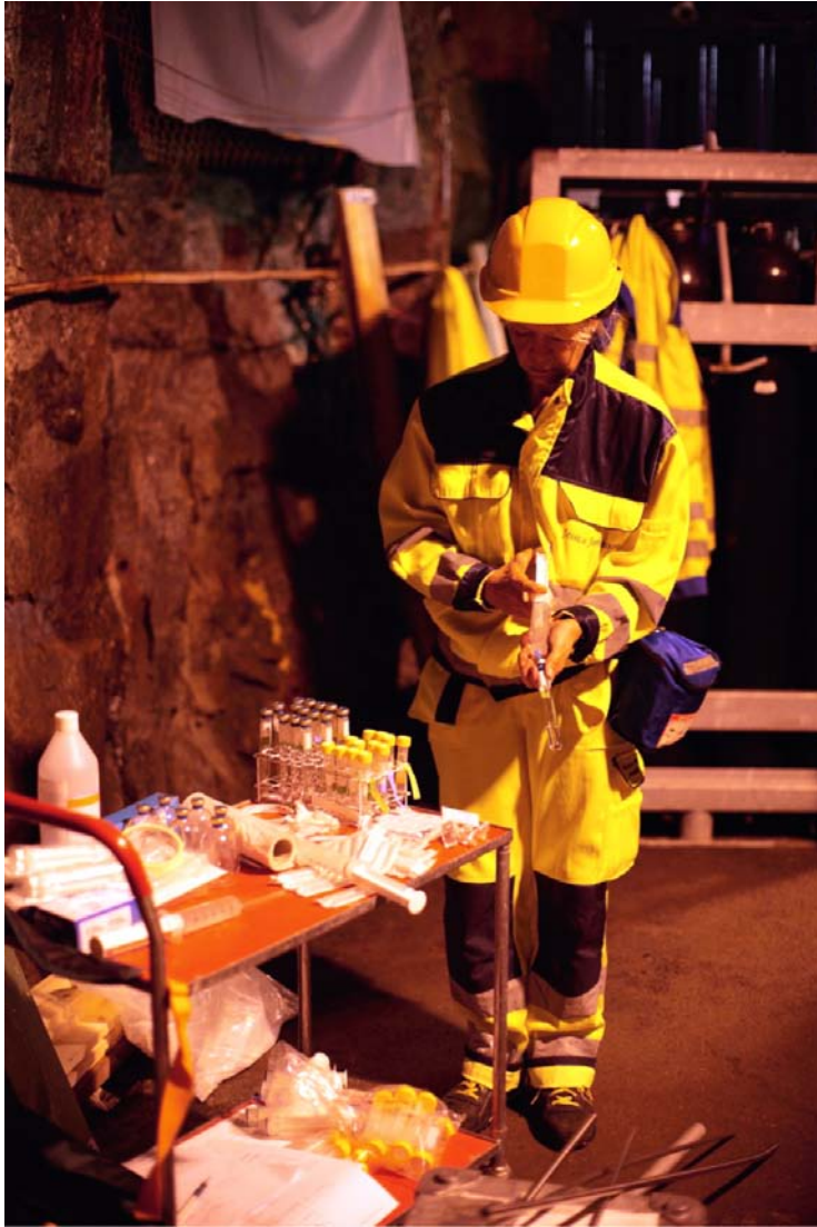
Figure 2-4. Sterile transfer of a water sample to an anaerobic, sterile test tube.
