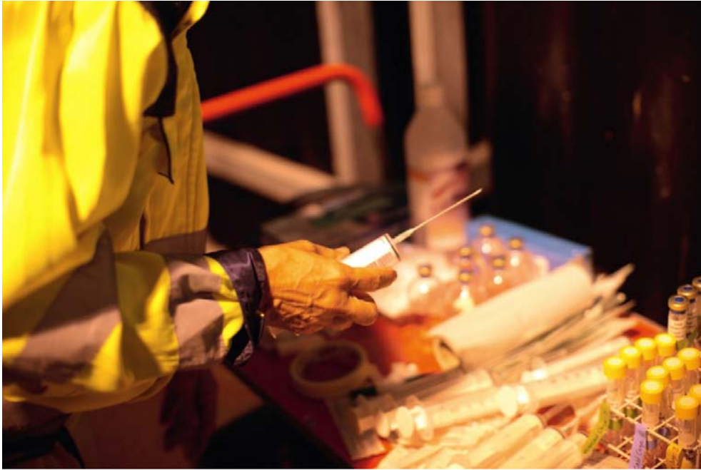
Figure 2-2. Samples from container water and support cage surfaces were taken with sterile syringes and needles.
