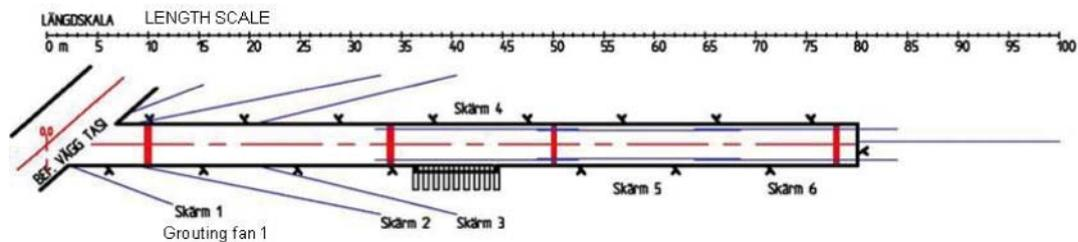
**Figure 3-47.** Principal drawing of the TASS-tunnel. The pre-grouting fans are marked with blue lines and the weirs with thick red lines across the tunnel (Skärm 1, Skärm 2 etc = Grouting Fan 1, Grouting Fan 2 etc.). Drawing modified from /Funehag 2008/.
