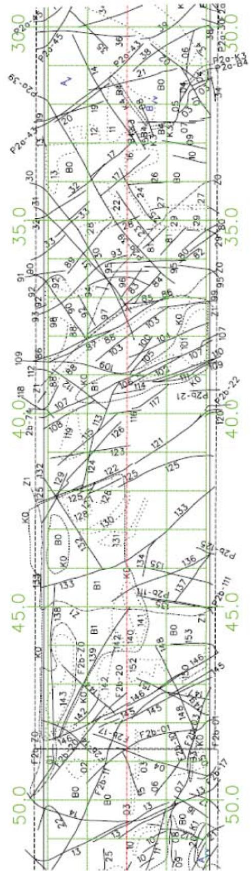
3D model with the geological mapping wrapped around a theoretical tunnel model
