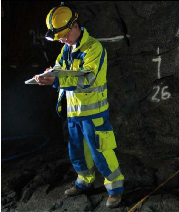
**Figure 2-2.** Tunnel floor mapping on plastic-coated paper (around section 24 m of the TASS-tunnel).
