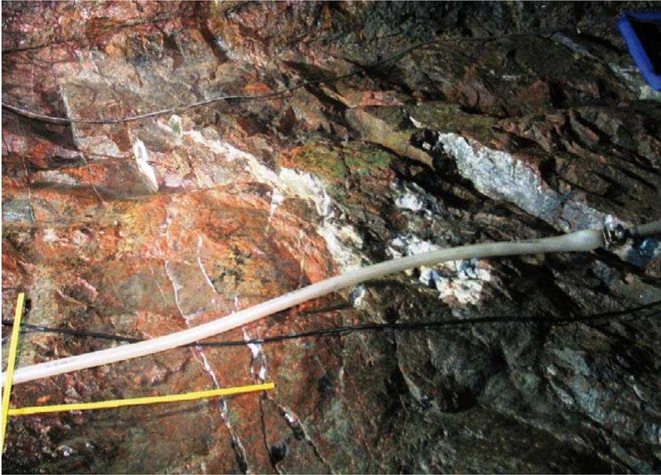
**Figure 3-31.** Floor, approximate section 19–20 m, fracture ID: G-42, 2 fractures, width: 5 mm, orientation: 287/90 (see Appendix II B). Calcite-filled fractures (white).
