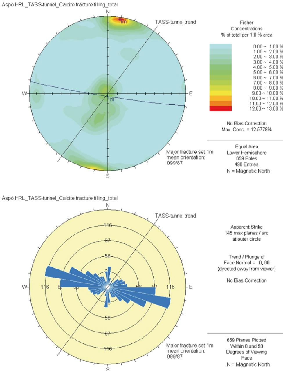
**Figure IX B.** Orientation of fractures that contain calcite as a fracture-filling mineral in the TASS-tunnel presented in Schmidt net and joint rosette diagrams. The 216° trend of the TASS-tunnel is marked as a black line. The main orientation set is 1 m: 099/87.
