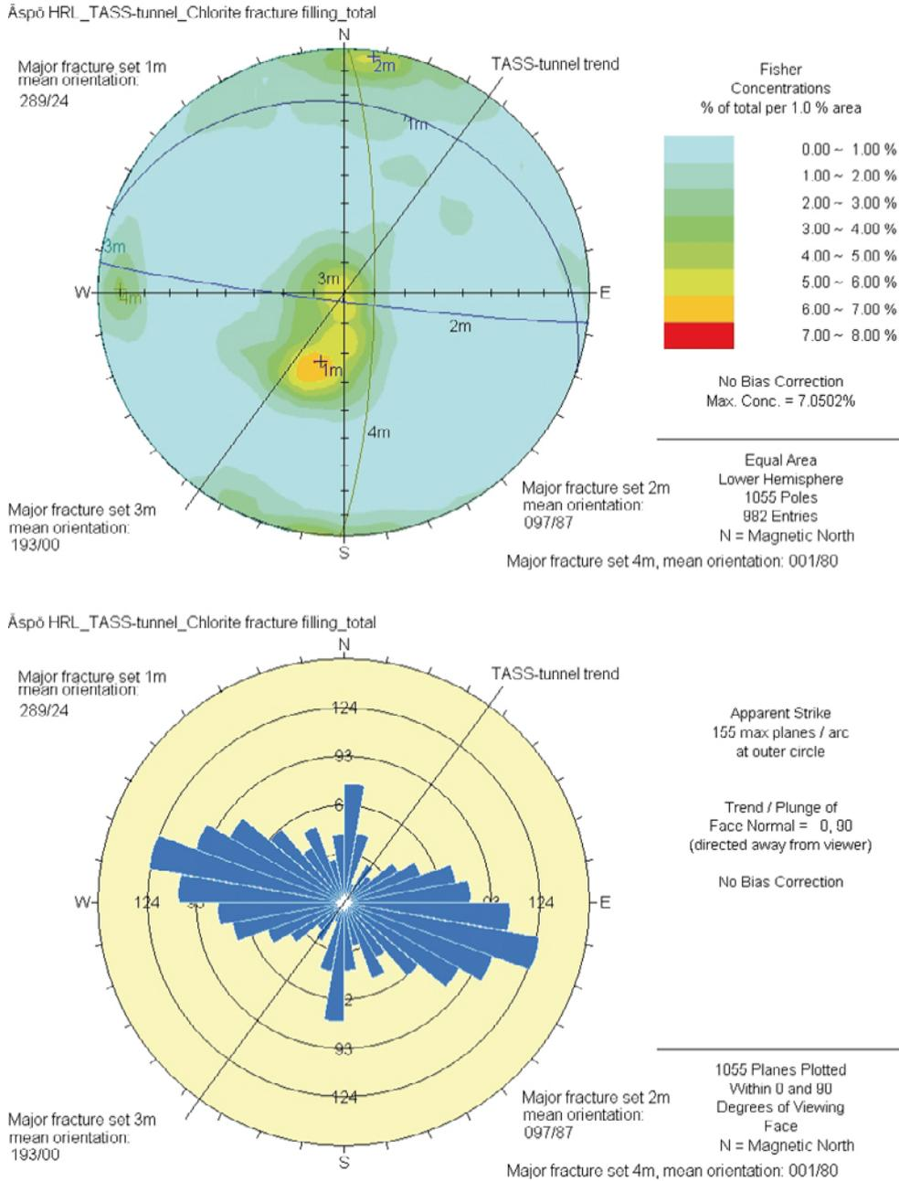
**Figure IX A.** Orientation of fractures that contain chlorite as a fracture-filling mineral in the TASS-tunnel presented in Schmidt net and joint rosette diagrams. The 216° trend of the TASS-tunnel is marked as a black line. The main orientation set is 1 m: 289/24. Three less prominent sets can also be seen, set 2 m: 097/87, set 3 m: 193/00 and set 4 m: 001/80.
