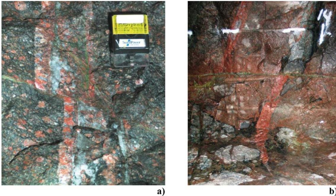
**Figure 3-39a–b.** Displacements. **a)** Floor, section around 26 m. Minor (about 0.1 m) displacement of a pegmatite dyke (P2a-B3) along an almost vertical fracture (fracture G2-45, orientation 260/80, see Appendix III A and III C). **b)** Left-hand wall, section 13–14 m. About 0.5 m displacement of a pegmatite dyke (P-B4) by a sub-horizontal, persistent fracture (fracture F-03, designated orientation: 000/00, see Appendix II A).
