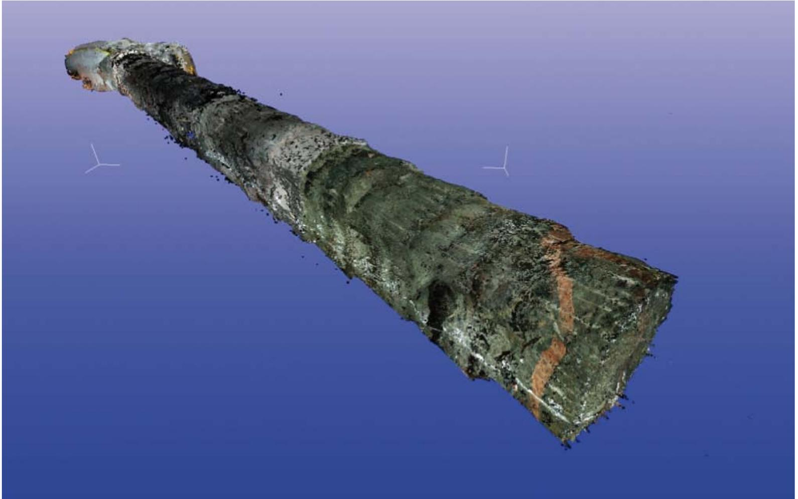
**Figure 5-6.** A model of the TASS-tunnel that is based on all the coloured laser scans and viewed from the outside. The scans have been partially cleaned from noise by using Pointools software. Part of the TASI-tunnel is visible in the upper left-hand corner and the final tunnel face in the lower right-hand corner.
