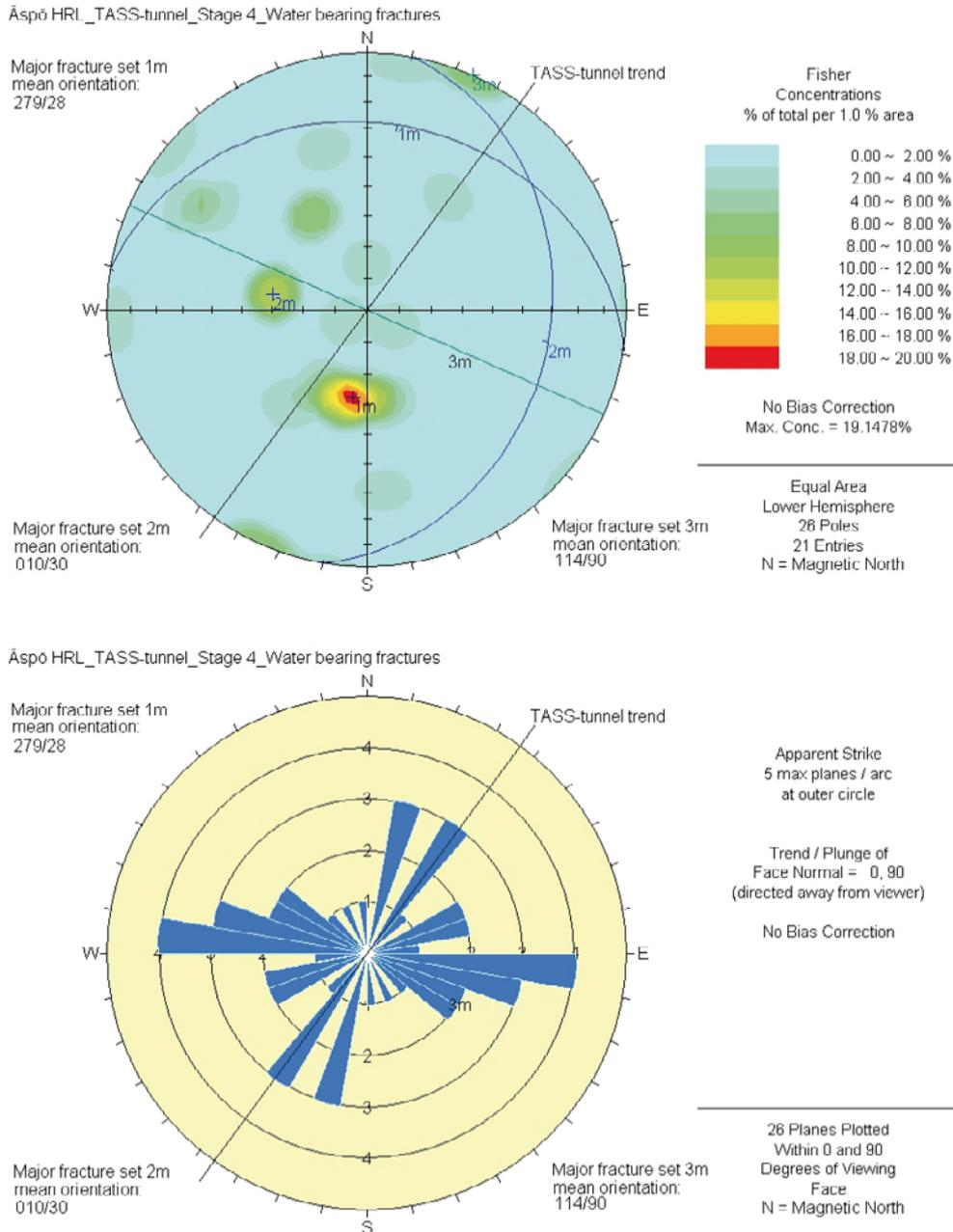
**Figure 3-62.** Orientation of all water-bearing fractures from the fourth stage mapping (64.6–80.7 m) of the TASS-tunnel presented in Schmidt net and joint rosette diagrams. The 216° trend of the TASS-tunnel is marked as a black line. One main orientation set can be seen, i.e. 1m: 279/28, as well as two less prominent sets, 2m: 010/30 and 3m: 114/90. N refers to magnetic north.
