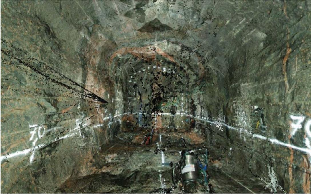
**Figure 5-4.** The TASS-tunnel, section 70–80.7 m. Colour scan (laser image with RGB from digital photos) still with some unwanted noise such as, for example, the black dots.
