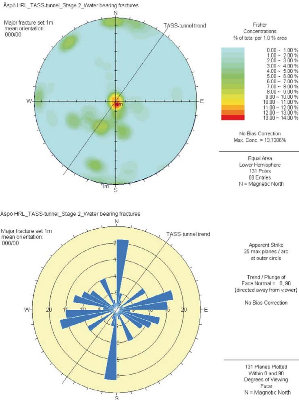
**Figure 3-56.** Orientation of all water-bearing fractures from the second stage mapping (20.7–48.7 m) of the TASS-tunnel presented in Schmidt net and joint rosette diagrams. The 216° trend of the TASS-tunnel is marked as a black line. One main orientation set can be seen, namely 1m: 000/00. The north-south striking trend on the rosette diagram is mainly caused by horizontal fractures that have the designated structural orientation 000/00. N refers to magnetic north.
