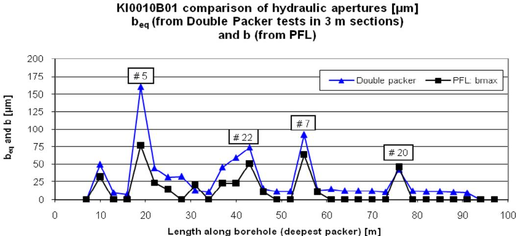
**Figure 4-2.** Comparison between the largest  $b$ -value (hydraulic aperture) from PFL (Posiva Flow Log) within each 3 m section and the  $b_{eq}$  (equivalent hydraulic aperture) from double packer from the same sections in borehole KI0010B01. Hydraulic measurements indicating structures #5, #7, #8, #20 and #22, from /Hardenby et al. 2008/.
