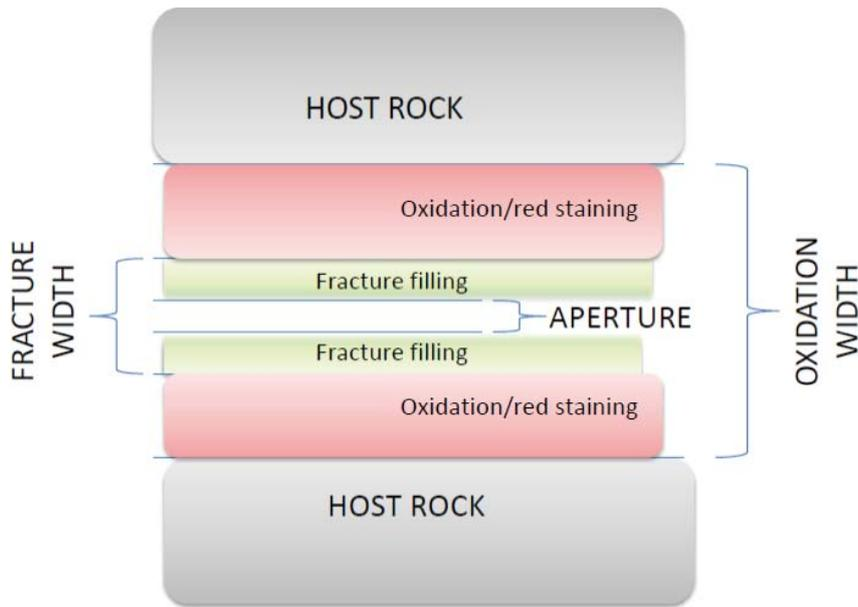
**Figure 2-1.** Principle drawing of the parts of a fracture. The fracture width is defined as possible aperture plus possible fracture filling measured across the fracture. Oxidation rims along fractures are measured in the same way and include the fracture width.
