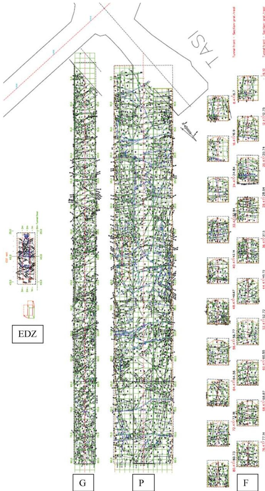
**Figure 3-1.** Summary of the geological mapping of the TASS-tunnel as it is presented on the TMS dgn-drawing. EDZ = EDZ-slot, G = floor, P = walls and roof, and F = tunnel face (see Figures 2-3 and 2-4 and, for a better resolution, Appendices I to VI).
