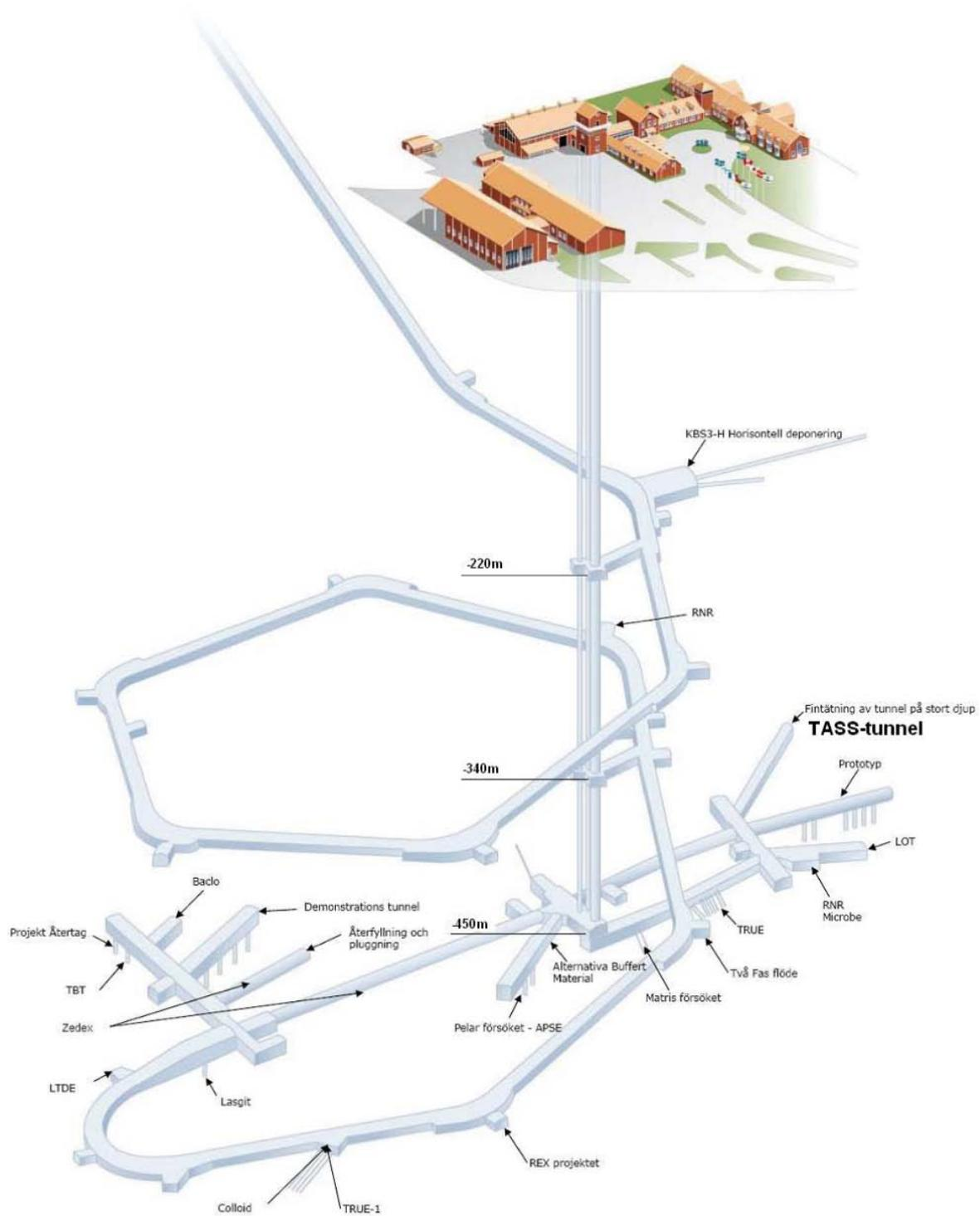
Figure 1-1. The Äspö HRL, including location of the TASS-tunnel.
