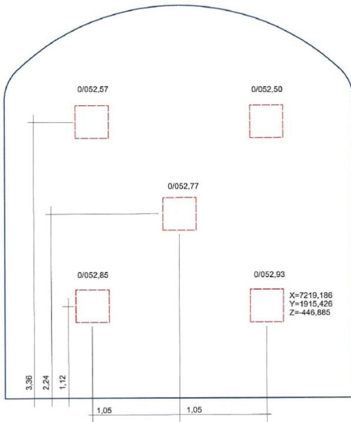
**Figure 2-8.** Five points measured by the surveyor G. Johansson at Geocon AB on the tunnel face of the theoretical section 52.47 m. In this example, the average of these points will be 52.72 and will define the true section 52.72 m.
