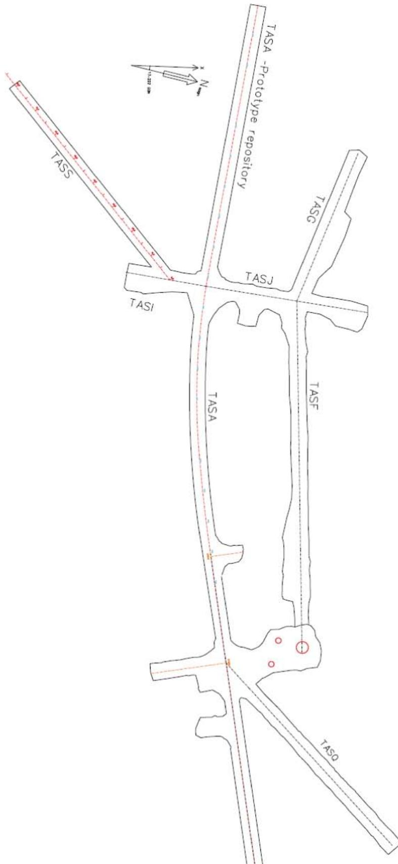
**Figure 1-2.** Äspö HRL, contours of the tunnels at the -450 m level including location of the TASS-tunnel. The orientation of the TASS-tunnel is  $230^\circ$  (Äspö 96) or  $215.8^\circ$  (magnetic north). North arrow: N magn = magnetic north, x = north Äspö 96.
