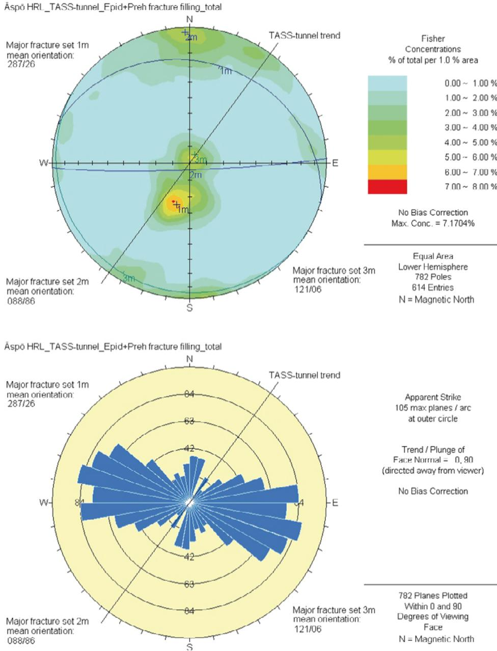
**Figure IX E.** Orientation of fractures that contain epidote and prehnite as fracture-filling minerals in the TASS-tunnel presented in Schmidt net and joint rosette diagrams. The 216° trend of the TASS-tunnel is marked as a black line. The main orientation set is 1 m: 287/26. Two less prominent sets can also be seen, set 2 m: 088/86 and set 3 m: 121/06.
