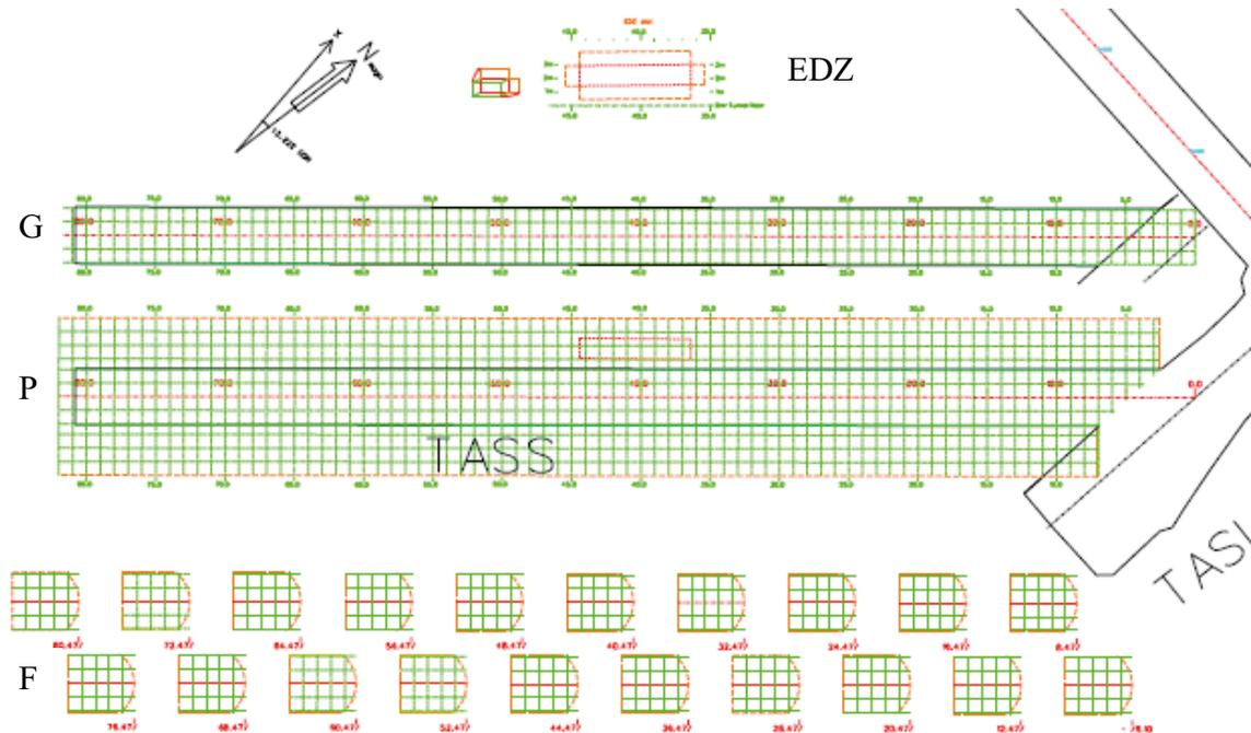
**Figure 2-4.** Layout of 2-D drawing on which the mapping results from the TASS-tunnel will be drawn (EDZ = EDZ-slot, G = floor, P = walls and roof, and F = tunnel face, see Figure 2-3).
