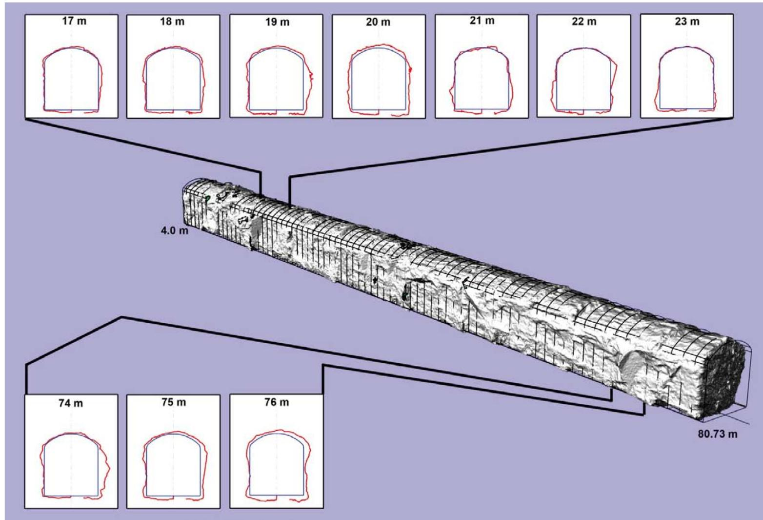
**Figure 5-8.** Triangulated model of the TASS-tunnel based on intensity laser scans. Topography of the tunnel surfaces and some theoretical cross sections (blue) compared to the real contour (red).
