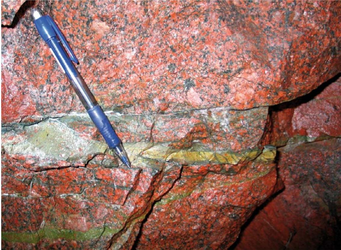
*Figure 3-44. Brecciated and oxidized Äspö diorite. Small fragments of Äspö diorite can be seen in an early epidote/prehnite filling. Note that some of this filling has in turn also been brecciated. Tunnel face 6.1 m, fractures 05 and 06 (see Appendix I B).*
