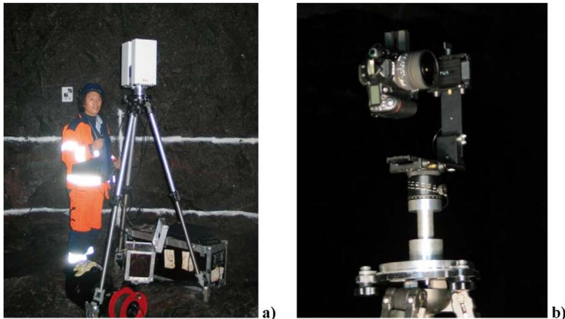
**Figure 5-1a–b.** TASS-tunnel equipment at approximately section 48 m. **a)** Laser scanner on a tripod, marker (paper tag with black and white chequered pattern on the wall) and operator. **b)** Digital Nikon D80 SLR camera on a tripod.
