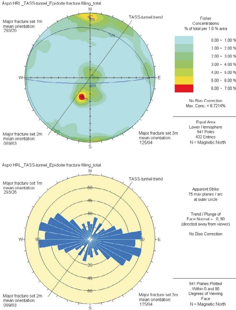
**Figure IX C.** Orientation of fractures that contain epidote as a fracture-filling mineral in the TASS-tunnel presented in Schmidt net and joint rosette diagrams. The 216° trend of the TASS-tunnel is marked as a black line. The main orientation set is 1 m: 293/26. Two less prominent sets can also be seen, set 2 m: 089/83 and set 3 m: 125/04.
