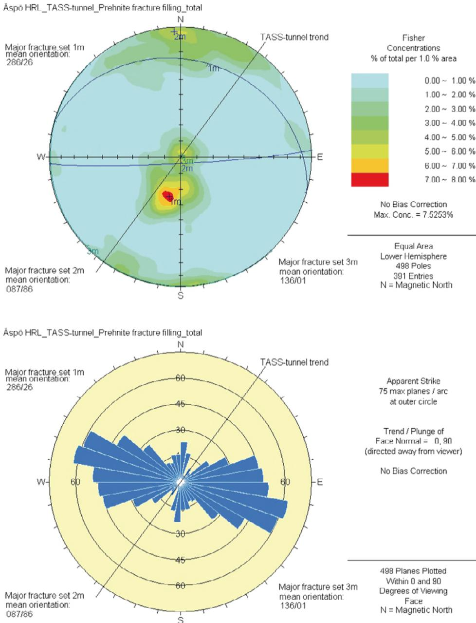
**Figure IX D.** Orientation of fractures that contain prehnite as a fracture-filling mineral in the TASS-tunnel presented in Schmidt net and joint rosette diagrams. The 216° trend of the TASS-tunnel is marked as a black line. The main orientation set is 1 m: 286/26. Two less prominent sets can also be seen, set 2 m: 087/86 and set 3 m: 136/01.
