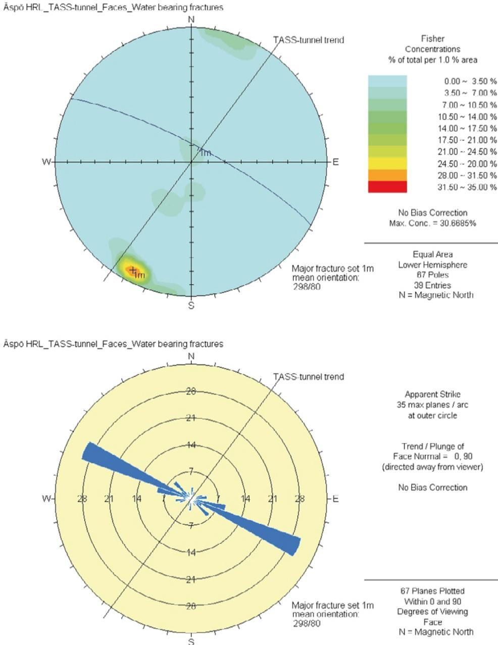
**Figure 3-50.** Orientation of all water-bearing fractures in the faces of the TASS-tunnel presented in Schmidt net and joint rosette diagrams. The 216° trend of the TASS-tunnel is marked as a black line. One main orientation set can be seen, namely 1m: 298/80. N refers to magnetic north.
