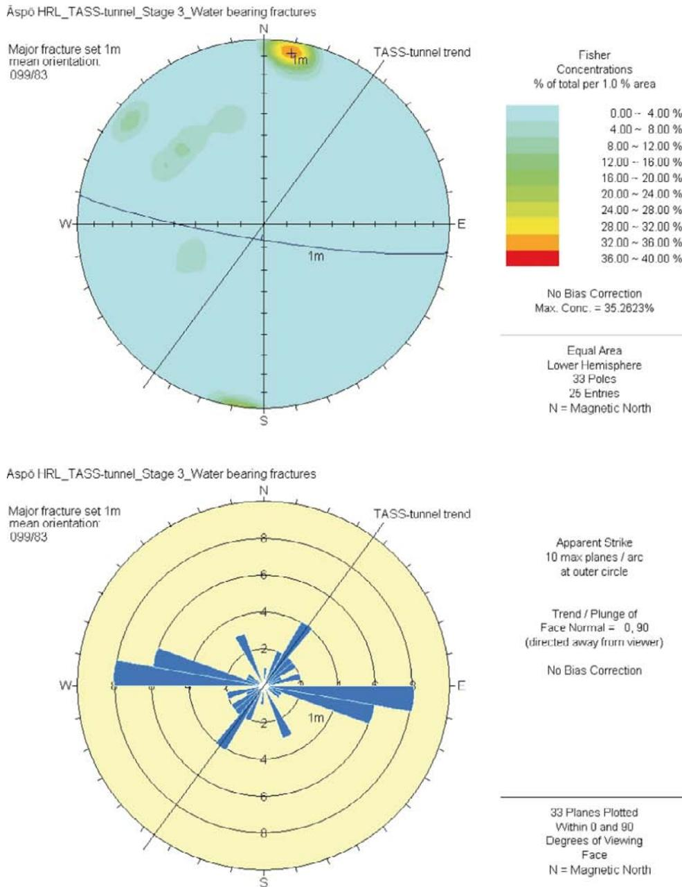
**Figure 3-59.** Orientation of all water-bearing fractures from the third stage mapping (48.7–64.6 m) of the TASS-tunnel presented in Schmidt net and joint rosette diagrams. The 216° trend of the TASS-tunnel is marked as a black line. One main orientation set can be seen, namely 1m: 099/83. N refers to magnetic north.
