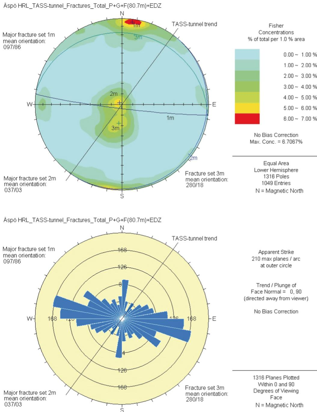
**Figure VIII A.** Fracture orientations from the whole TASS-tunnel presented in Schmidt net and joint rosette diagrams. The 216° trend of the TASS-tunnel is marked as a black line. One main orientation set can be seen, 1 m: 097/86, as well as two less prominent sets, 2 m: 037/03 and 3 m: 280/18.
