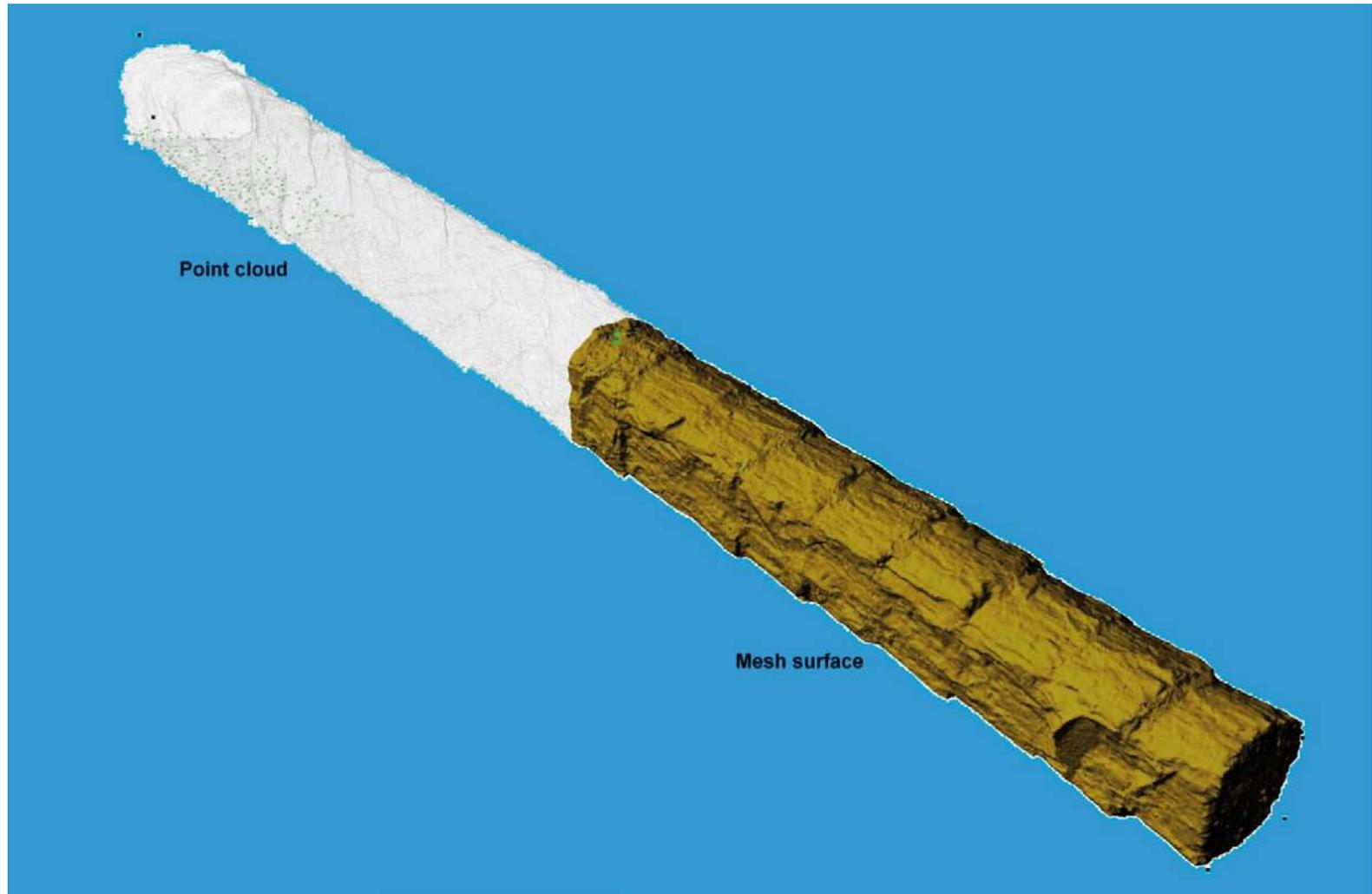
**Figure 5-5.** A model of the TASS-tunnel that is based on all the laser scans and viewed from the outside. One part of the tunnel is illustrated as point cloud and the other as mesh surface. The beginning of the tunnel is in the upper left-hand corner and the final tunnel face in the lower right-hand corner.
