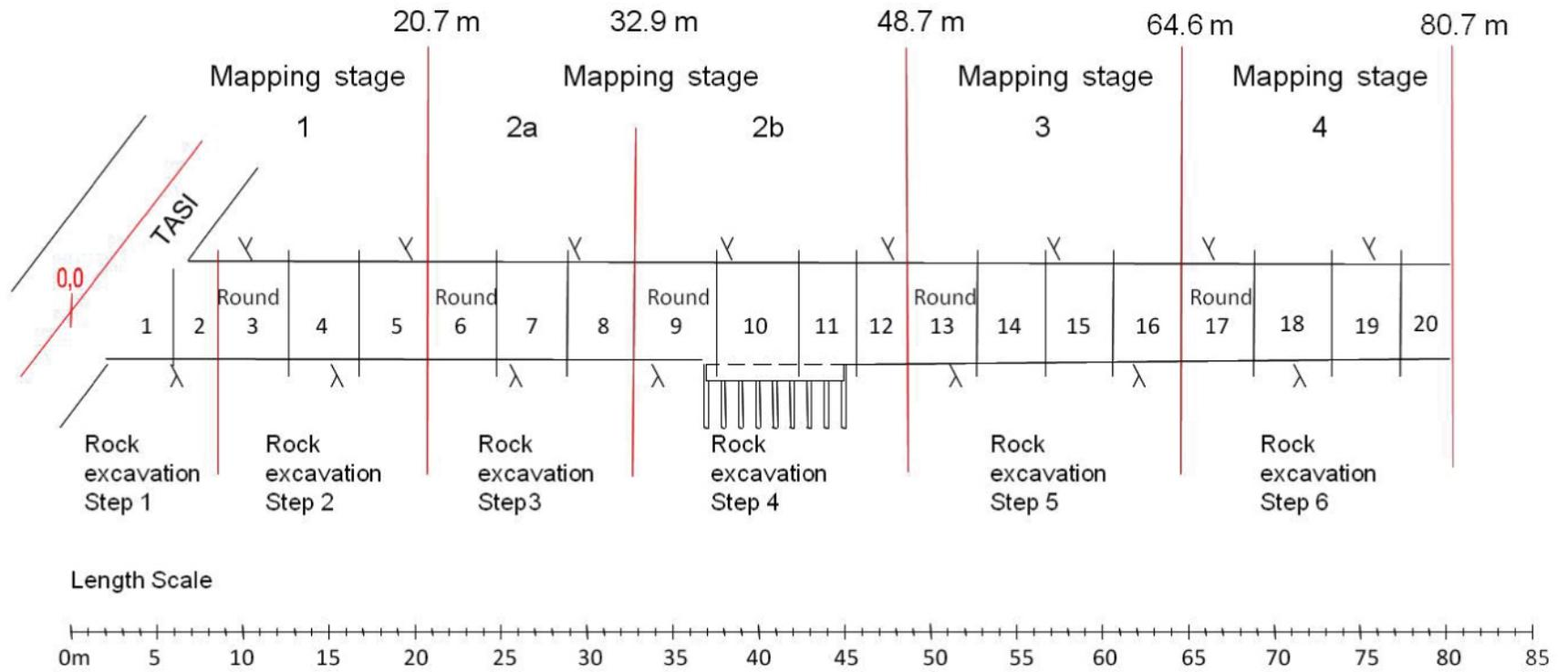
Figure 2-7. The figure shows how the mapping stages 1–4 are related to the rock excavation steps 1–6 (modified after /Karlzén and Johansson, 2010/).
