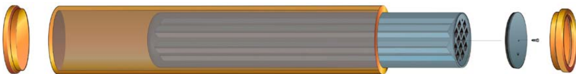
Figure 5-9. Exploded view of the canister components (from left: copper base, copper tube, insert, steel lid for insert and copper lid).
