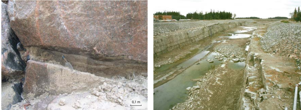
Figure 4-24. a) Laminated silt in an open fracture in the north-western part of the excavated area at drill site 5. The site was originally covered with till that has been removed. b) Horizontal fractures along the more than 1 km long canal between the Baltic Sea and the nuclear power reactors in Forsmark. These fractures are inferred to be sheet joints formed in connection with the release of stress in the bedrock (Figure 11-2 in the Site description Forsmark ).
