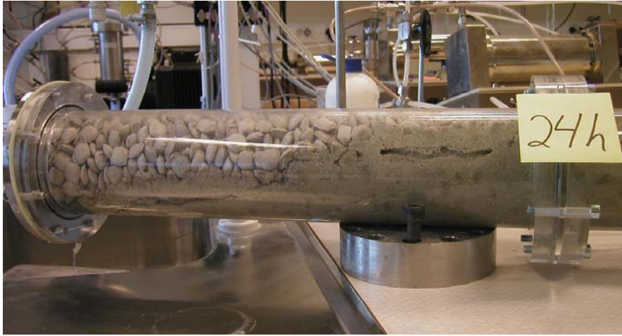
Figure 2-4. Photo of the test equipment used for piping/erosion measurements.
