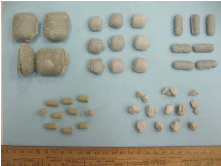
Figure 2-1. Examples of bentonite pellets used in repository sealing studies. (Upper row are pellets produced using roller compression (briquettes); Lower Left is example of typical extruded bentonite pellet; Lower Right are crushed HCB granules).
