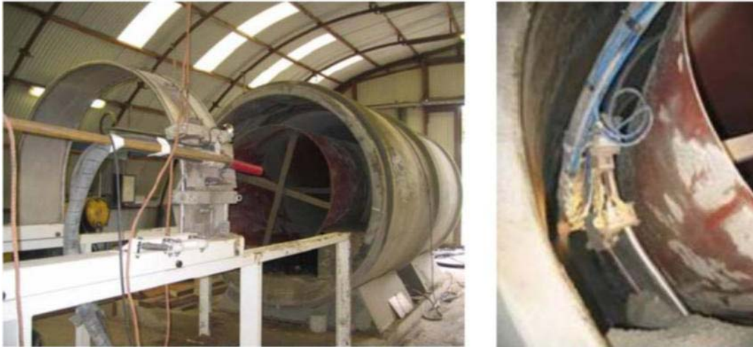
Figure 2-13. Placement trials for granular materials around supercontainer of type considered by ONDRAF/NIRAS, air-entrainment only (De Bock et al. 2008).
