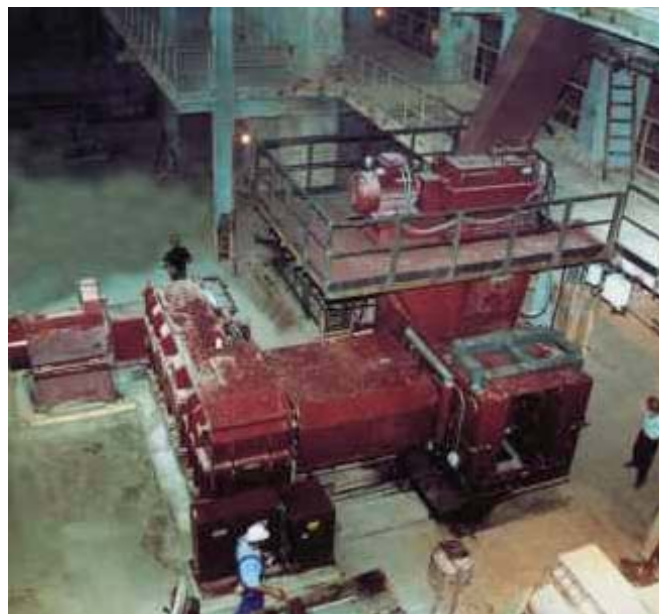
Industrial-scale roller compression machine (Hosokawa Bepex GmbH)
