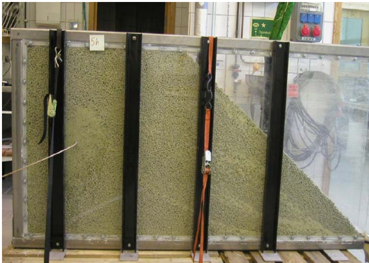
Figure 2-5. Photo of the test equipment used for studying the wetting behaviour.
