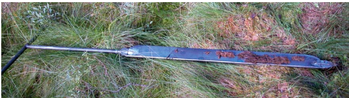
Figure 2-4. The Russian peat corer used for sampling of peat from the five wetland sites. One meter long peat samples can be obtained with this corer.
