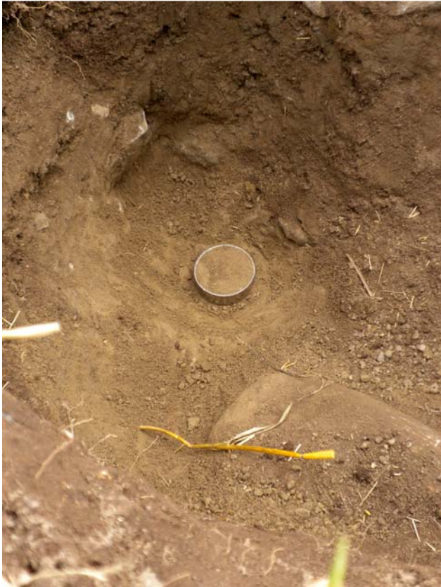
Figure 3-3. The clay till at sampling site AFM001359. The clay till is characterised by the abundance of stones and gravel. The cylinder has a diameter of 5 cm, and was used for taking samples to calculate density and porosity.
