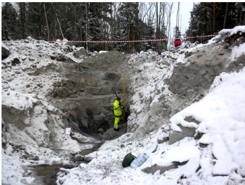
Figure 2-6. Trench 2 seen from the west towards the eastern side. The thickest layers of till were situated in the central part of the trench.
