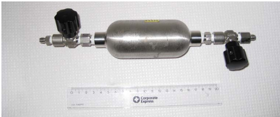
Figure 3-1. Vessel used for transport of gas samples from VTT. With courtesy of Ramboll Oy.
