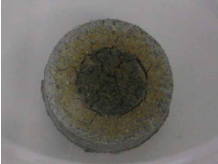
Figure 4-26. Bottom bentonite profile of Fe-bentonite sample after the 1 st swelling pressure and hydraulic conductivity measurements and drying in N 2 -atmosphere.
