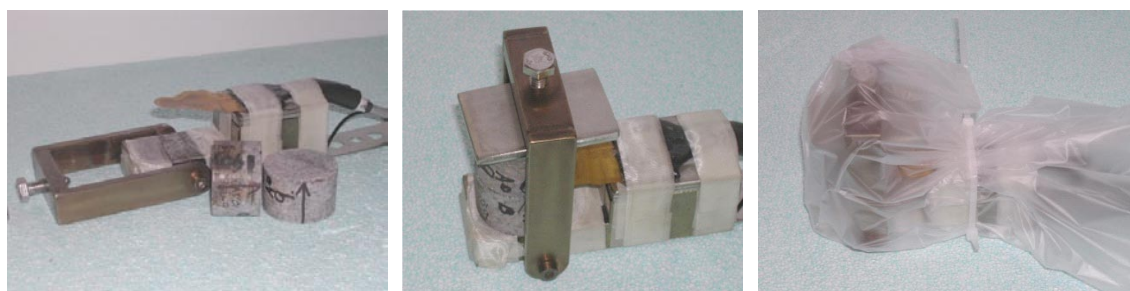
Figure 3-2. Specimens prior to mounting (left), mounted in stainless sample holder (middle), and sample holder with mounted specimens wrapped in plastic (right).
