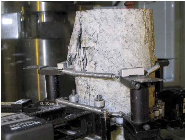
Figure 5-7. The specimen F01A-113-9 is scaling under the knife-edge.
