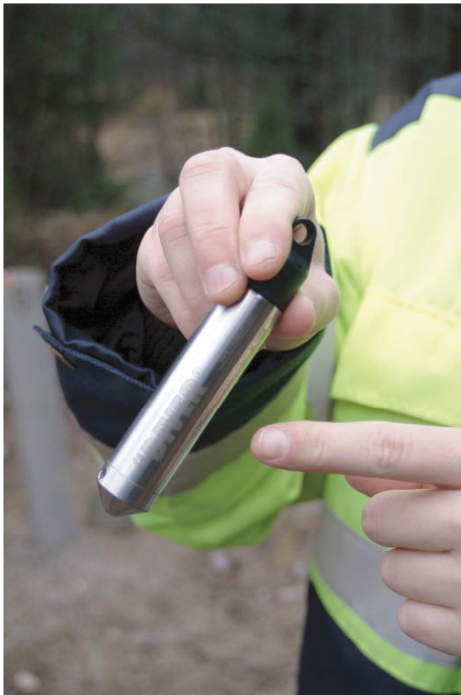
Figure 3-2. Close-up photograph of a Van Essen Instruments TD-Diver®, used for measurement of pressure and temperature in each well. Another Diver® model (CDT-Diver®), which was used in SFM0061, has an additional capability to measure the electrical conductivity.
