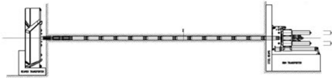
Figure 4-21. Design sketch for horizontal reaming of the deposition tunnels
