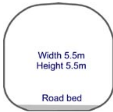
Figure 4-5. Suggested shape for the deposition tunnel. The tunnel section area is 27.4 m 2 .
