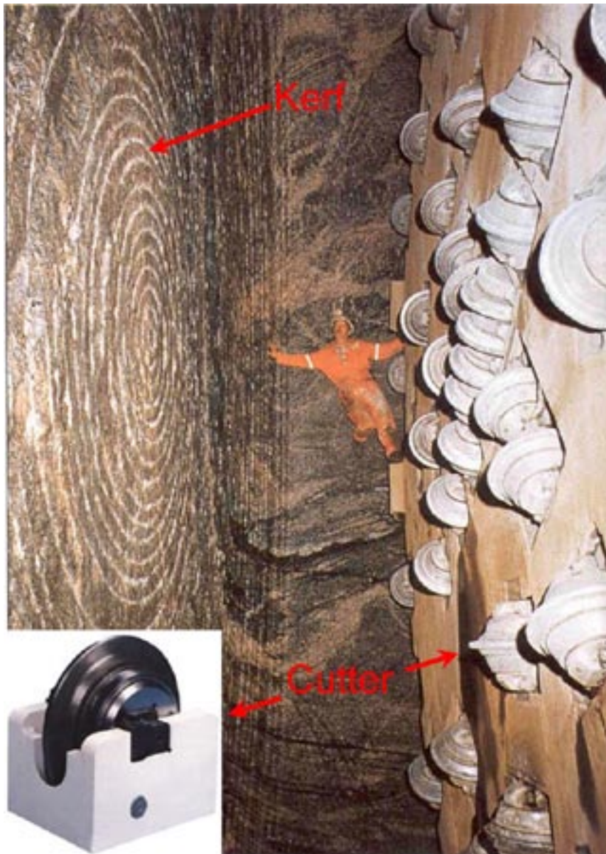
Figure 2-14. Kerfs (grooves) produced at a tunnel face by using disc cutters in a Tunnel Boring Machine (TBM) operation. Photos: Courtesy The Robbins Company.
