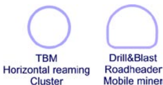
Figure 4-38. Tunnel shape will depend on choice of excavation method. Drill & Blast, roadheader and mobile miner may in principle excavate any shape.
