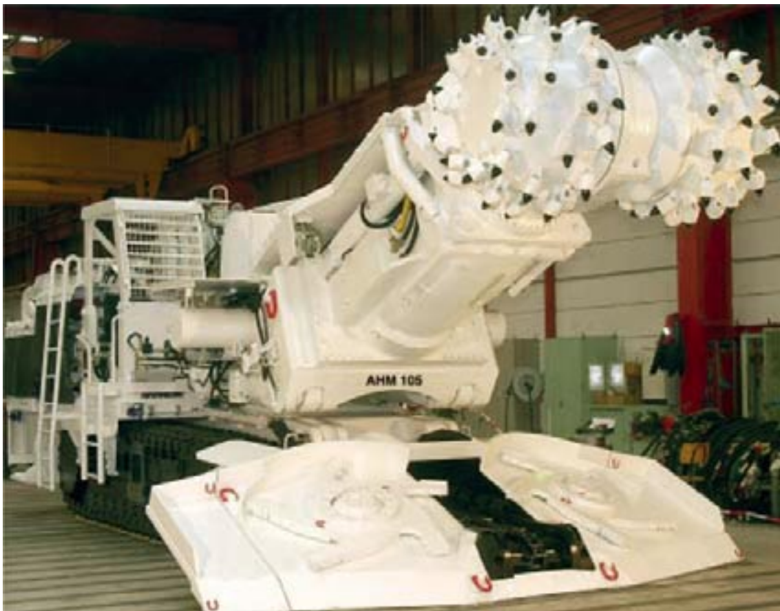
Figure 2-19. Example on equipment for mechanical excavation – roadheader. Courtesy Sandvik Voest Alpine.
