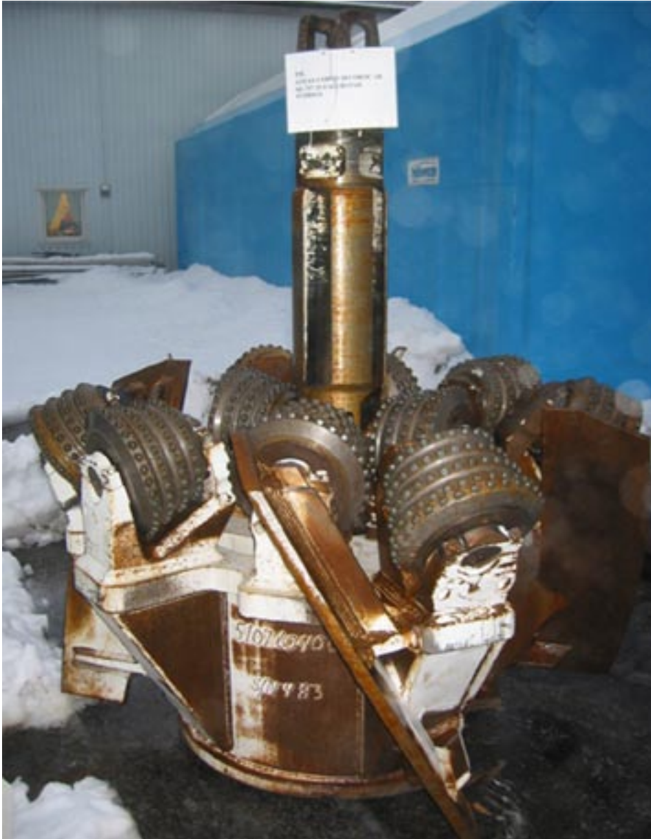
Figure 4-34. The reamer head used at the Sandvika project. The tunnel is 1.8 m in diameter and with length 285 m. Courtesy: Atlas Copco Construction & Mining.
