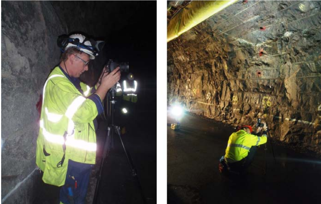
Figure 2-4. Photogrammetry course at Äspö HRL. Here how to handle the field equipment – digital camera, tripod, floodlights etc in the TASS-tunnel (to the left) and in the TASA-tunnel (to the right). Photo: C. Hardenby.
