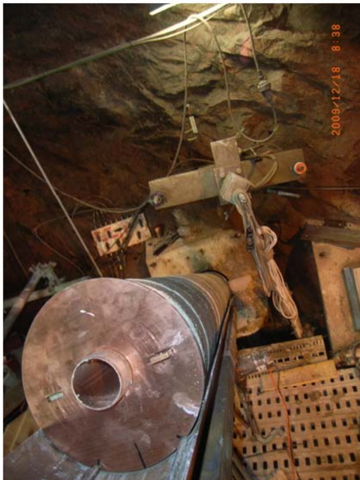
Figure 4-21. Placement of clay blocks. Upper: Funnel for letting the blocks slide down. Lower: Block column with copper plate and attached central tube passing through.
