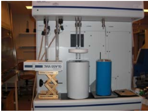
Figure 3-17. Instrument for making surface area and porosity determinations.
