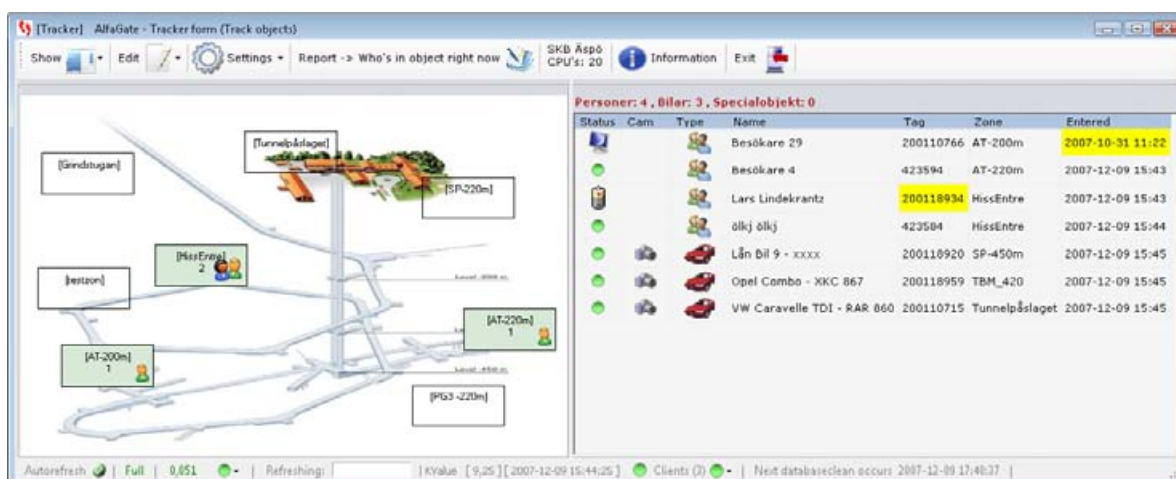
Figure 7-8. AlfaGate Tracker is the visualisation system which shows the locations of the persons in the Äspö HRL.
