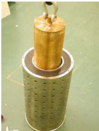
Figure 4-20. Model canister being lowered into support cage containing bentonite pellets in annulus.
