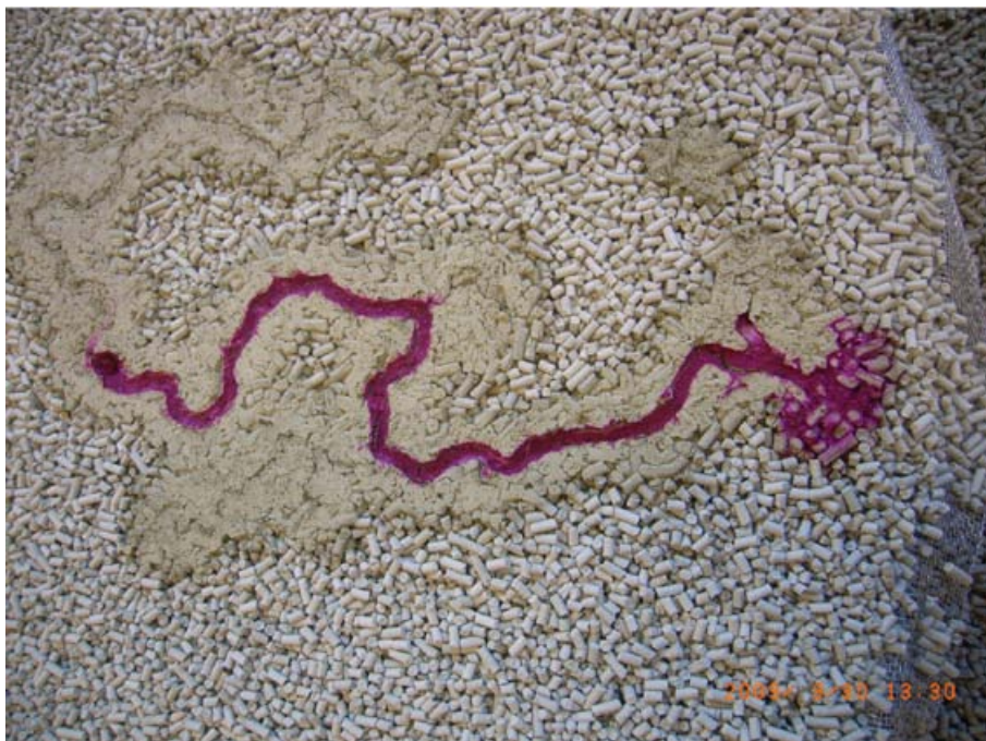
Figure 6-4. Appearance of water penetrating pellet filling contacting an initially water saturated rock slab.
