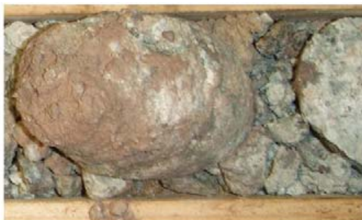
Samples from KAS17: 196,55-196,75. Fracture zone with gouge material
