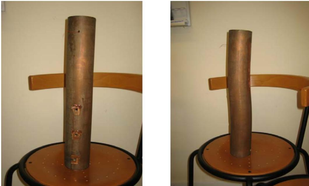
**Figure 3-12.** Copper rod used in one of the 1:10 scale rock shear tests just prior to sampling for stress-strain testing (photo taken April 30, 2010 at Clay Technology AB laboratory in Lund, Sweden).
