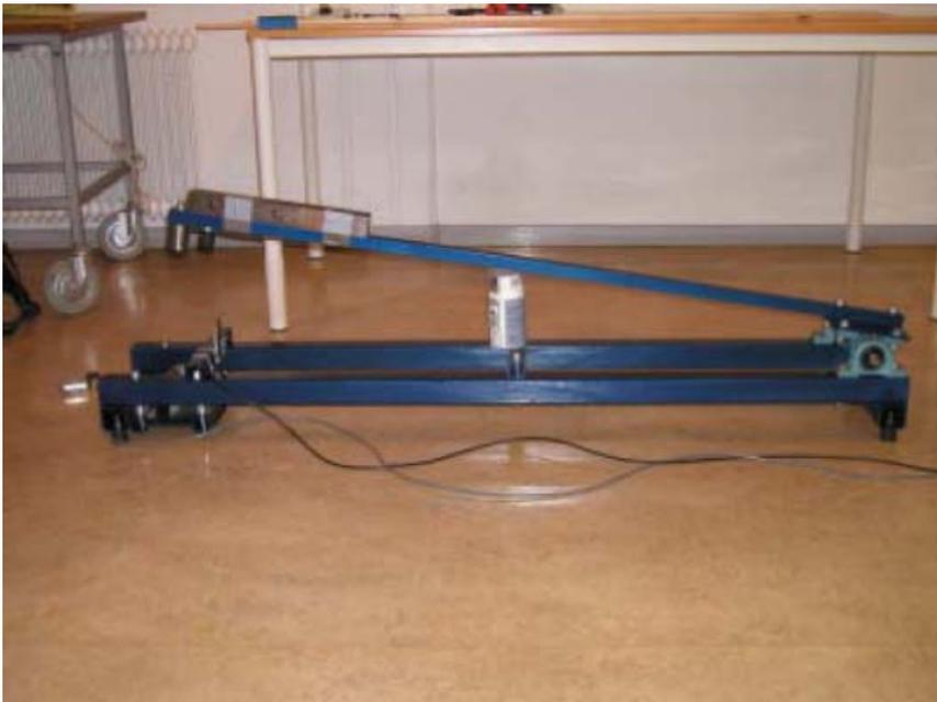
**Figure 3-3.** Fall hammer device for shearing samples at high shear rates (from /Börgesson et al. 2004/).
