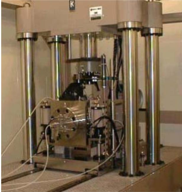
*Figure B-1. Photograph of the Japanese BORE-SHEAR apparatus for shear testing of composite EBS specimens.*
