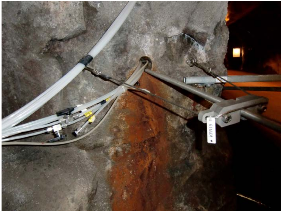
Figure 4-2. Connection between the borehole line used for pressure measurements and the surface Chemmac used in KFR19:1. Such a direct connection reduces the number of fittings and thereby minimizes the risk of external oxygen intrusion by diffusion or leakage. The line used is the one in the lower bundle marked with black tape.
