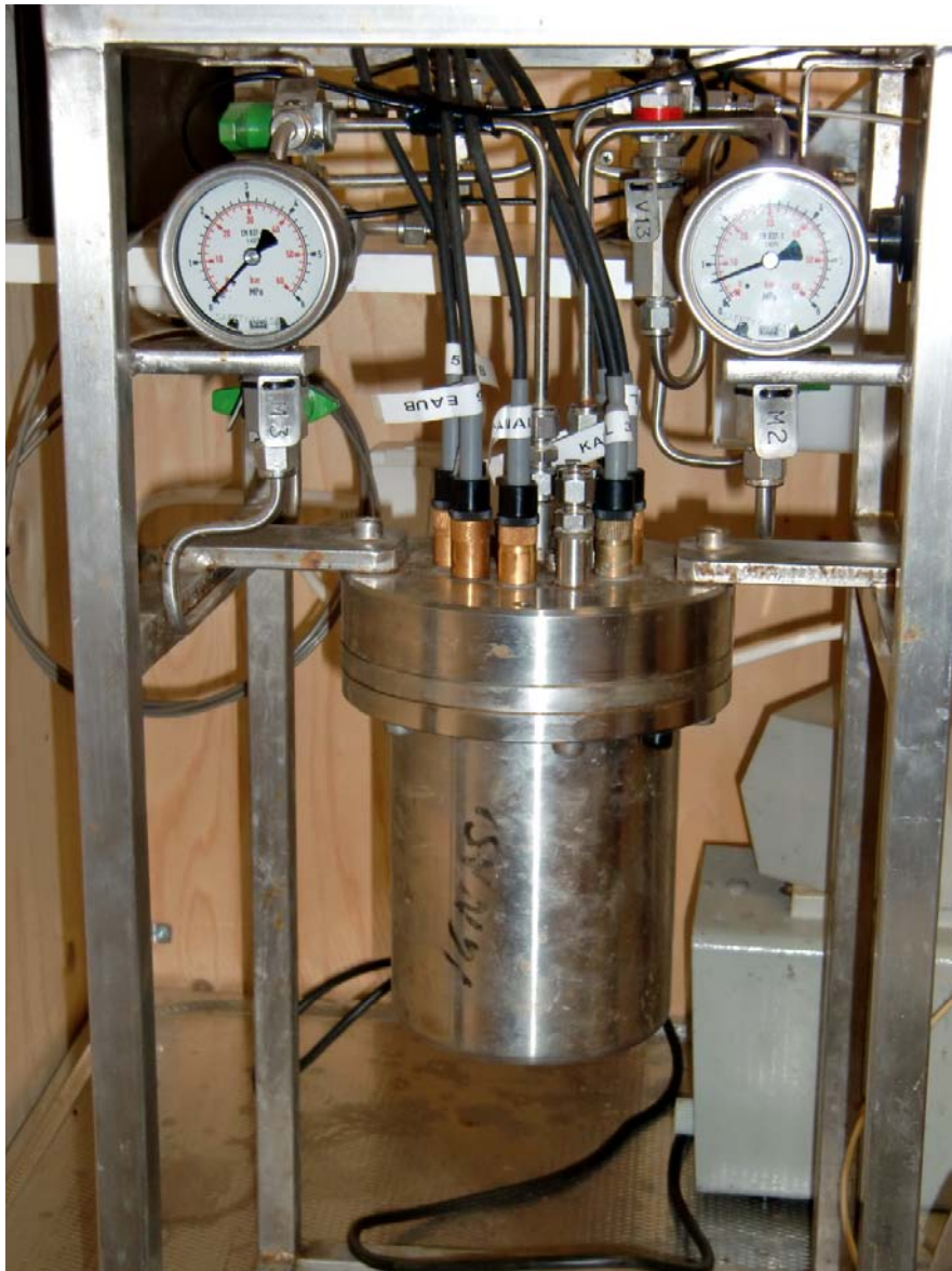
Figure 4-4. The measurement chamber, used in borehole sections KFR7A:1 and KFR08:1.
