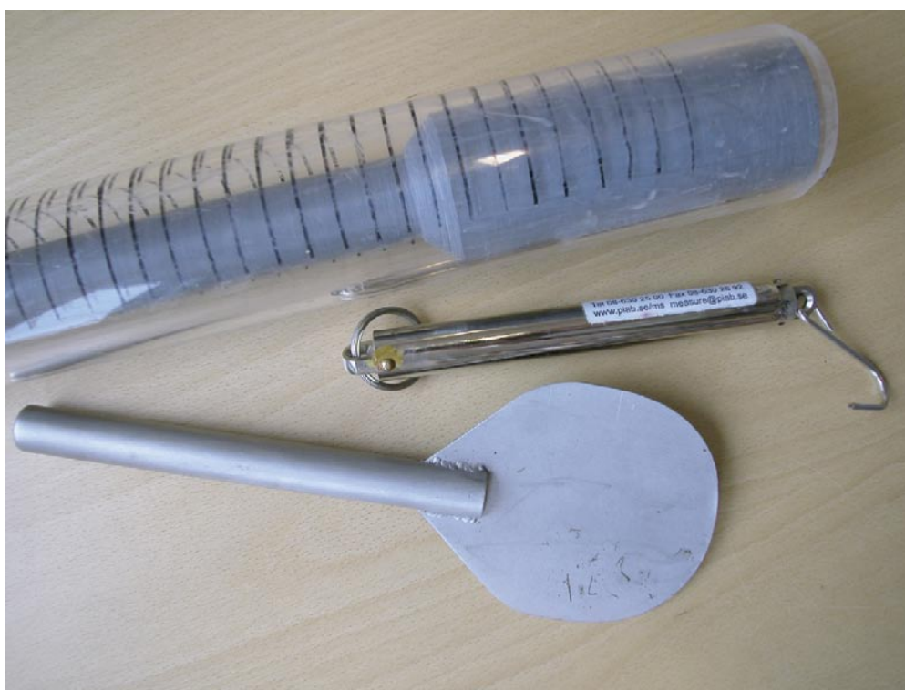
Figure 3-1. Equipment used to measure snow depth and snow weight.
