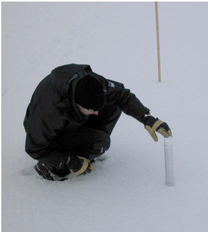
Figure 4-1. Measurement of snow depth with a plastic tube at Storskäret, AFM000071.
