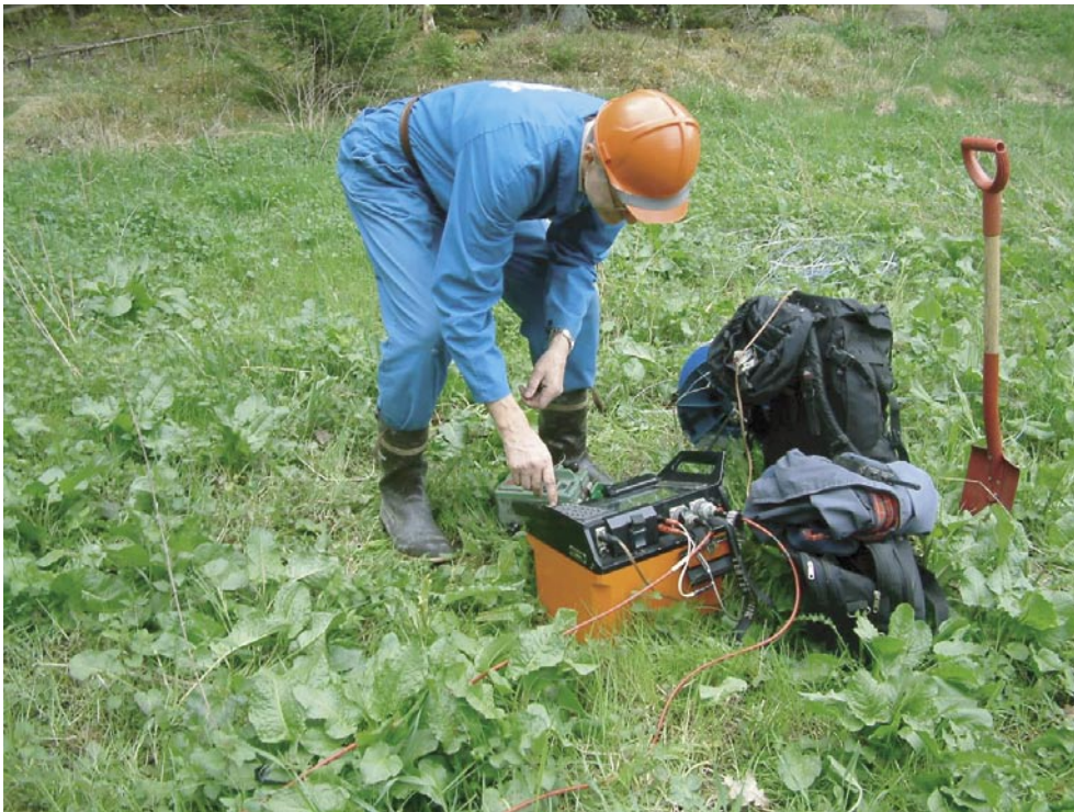
Figure 3-1. The recording instrument, ABEM Terraloc MK6.
