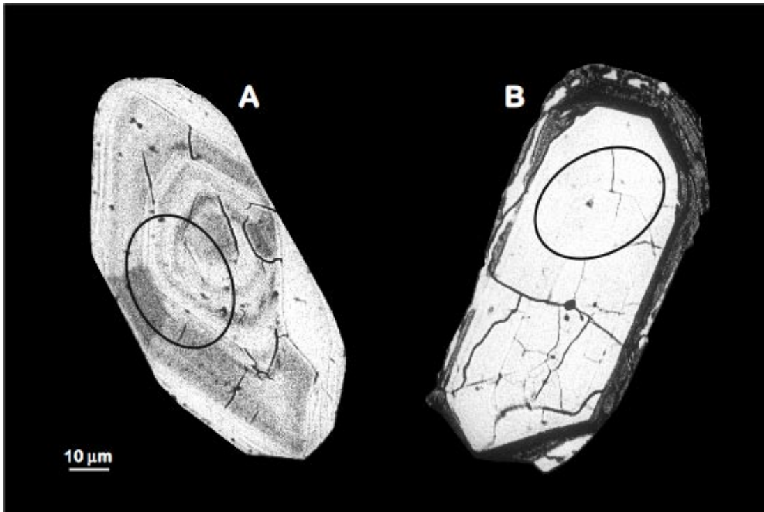
Figure 5-1. Representative BSE-images of zircons mounted for analysis by the SIMS technique. A: Zircon (analysis n1257-07a) with magmatic oscillatory zoning that has been included in an age calculation. B: Zircon (analysis n1257-06a) that lacks zoning, is BSE-bright and has been omitted from an age calculation. Ellipses mark analysed spots.
