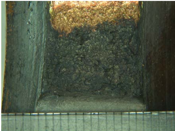
Figure 3-9. LOM image showing fracture surface for CCG215, test at 215°C.
