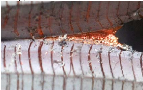
(c) 695 hrs, 150 MPa, LLD=1.92 mm
