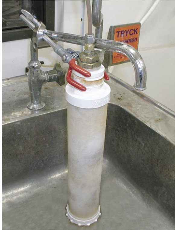
Figure 4-5. The ion exchange column mounted to the outlet of pumped groundwater from the borehole section.
