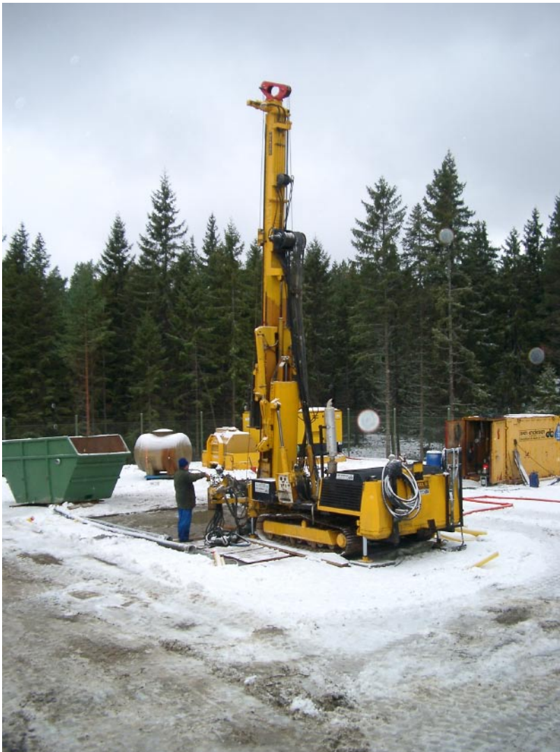
Figure 3-1. The Puntel MX 1000 drilling machine in operation at KFM02A.
