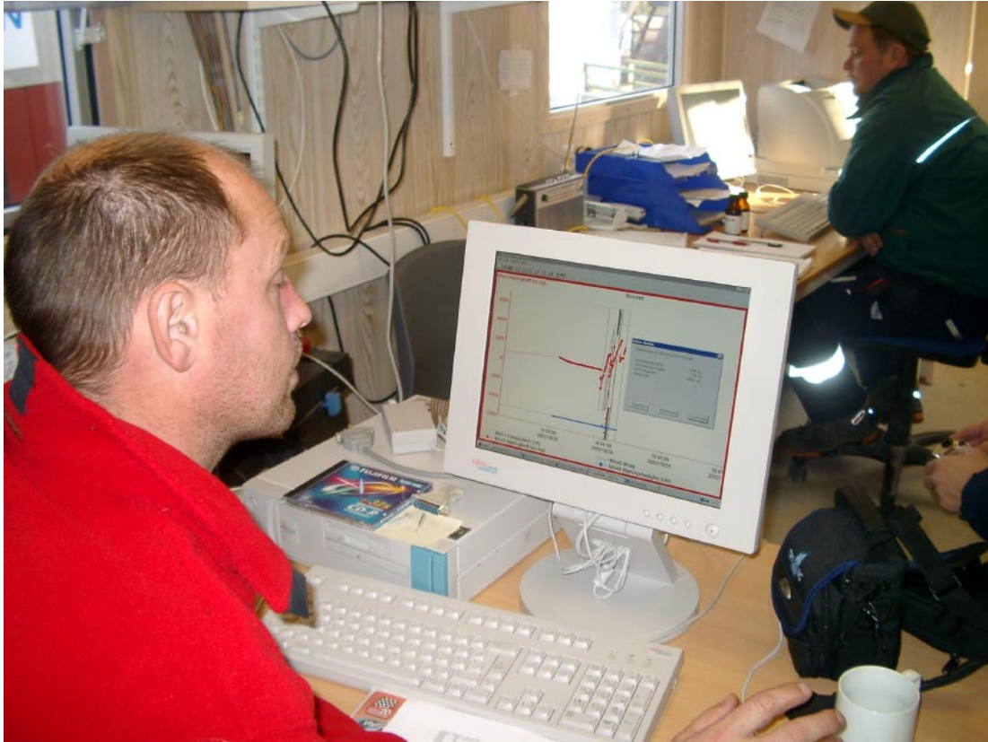
Figure 2-1. During drilling, a number of drilling related parameters are collected by a drilling monitoring system. Part of these data sets, in this report called DMS-data (Drilling Monitoring System), are transferred to the SKB database SICADA.
