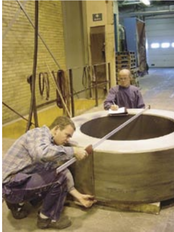
Figure 5-1. Control measurement of bentonite ring.
