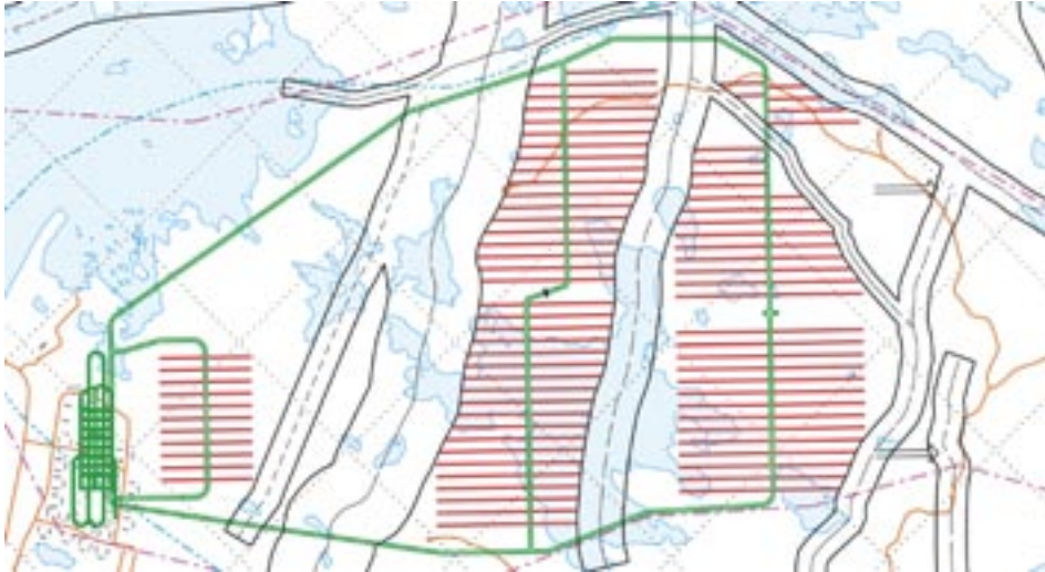
Figure 2-3. Repository layout at 400 m level in Forsmark.
