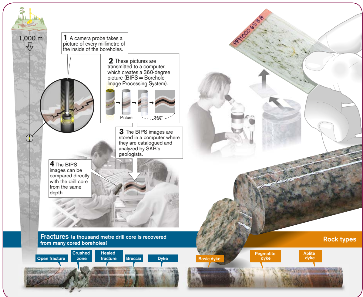
Figure 7-6. The site investigations, investigation of drill cores and boreholes.
