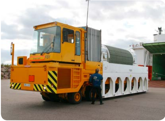
Figure 8-10. Terminal vehicle used for overland transport between the facilities (the nuclear power plants and Clab) and m/s Sigyn.
