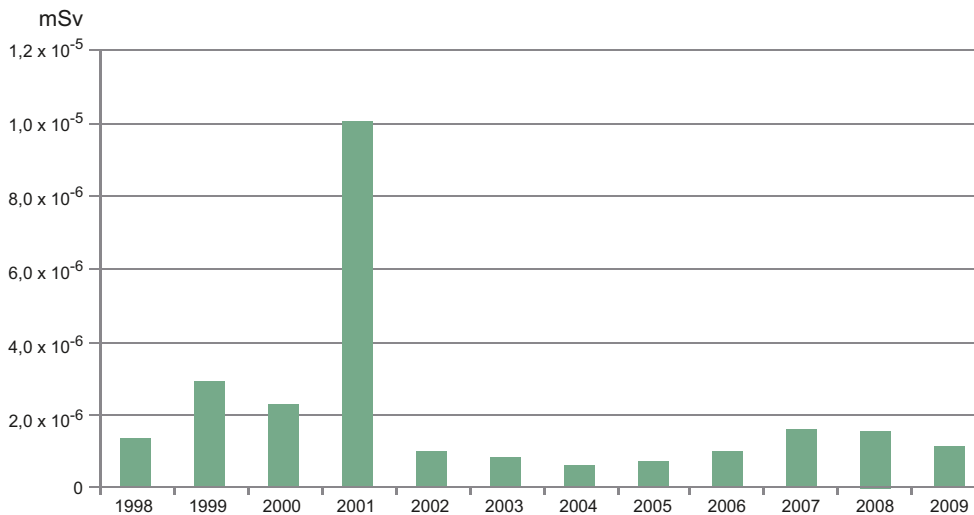
Figure 8-17. Dose to critical group from annual releases to air from Clab during the period 1998–2009.
