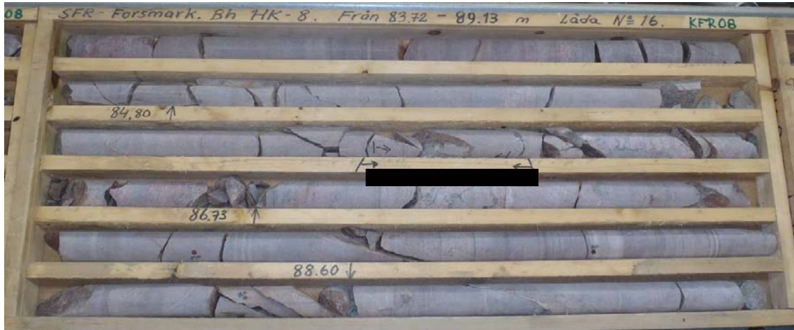
Figure A1-47. Photograph of the sampled drill core box. The sampled section is marked with a black line under the drill core.
