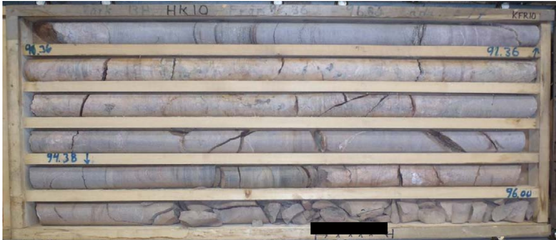
Figure A1-54. Photograph of the sampled drill core box. The sampled section is marked with a black line under the drill core.
