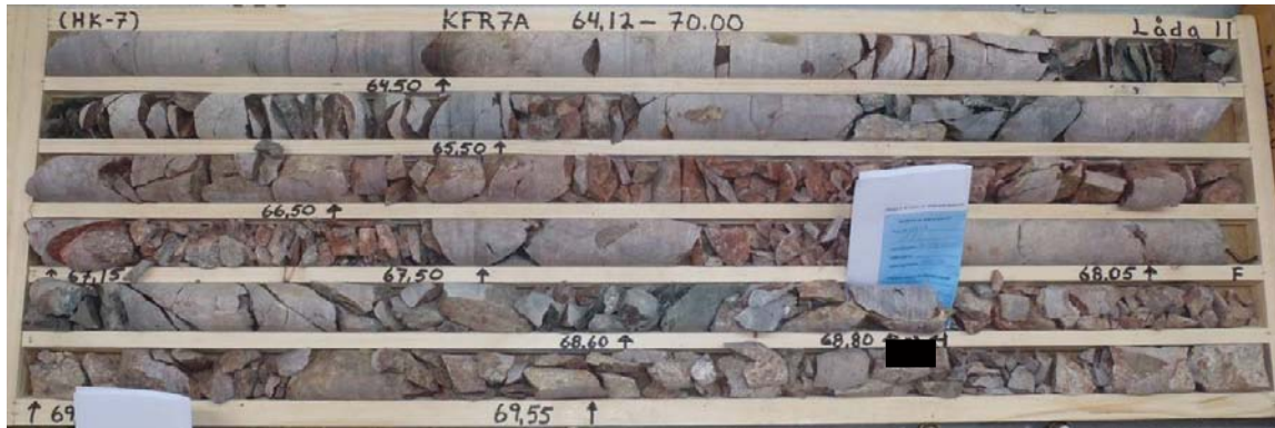
Figure A1-22. Photograph of the sampled drill core box. The sampled section is marked with a black line under the drill core
