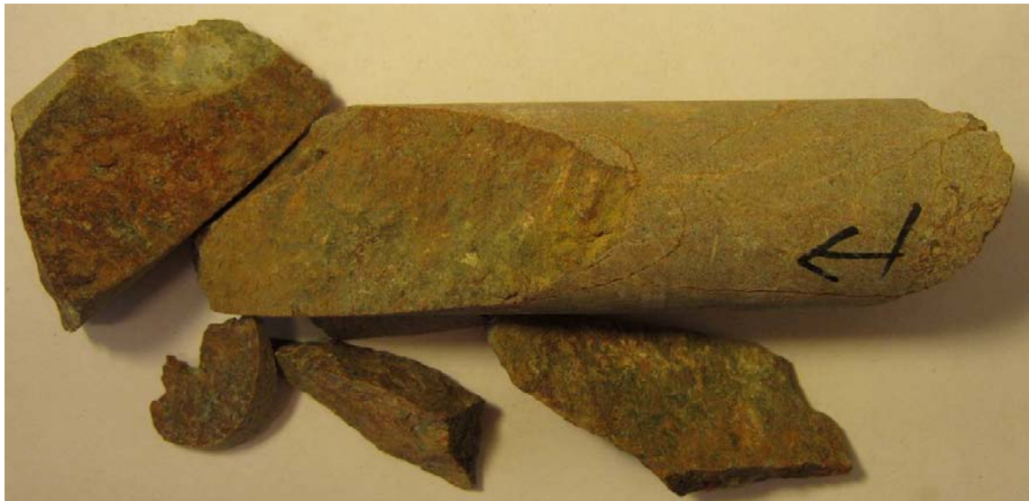
Figure A1-48. Photograph of the sampled fractures.
