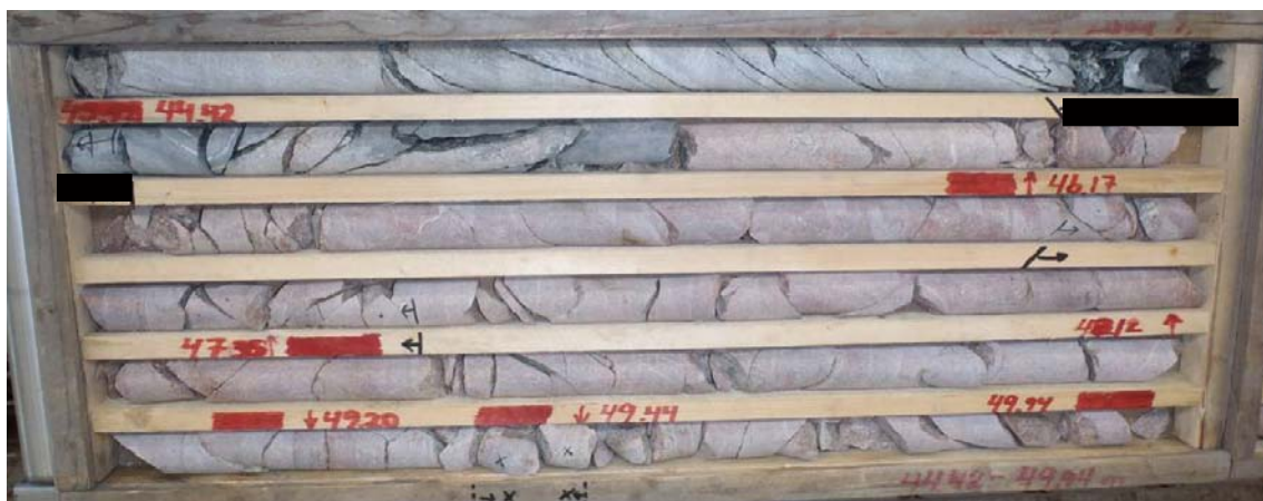
Figure A1-1. Photograph of the sampled drill core box. The sampled section is marked with a black line under the drill core.
