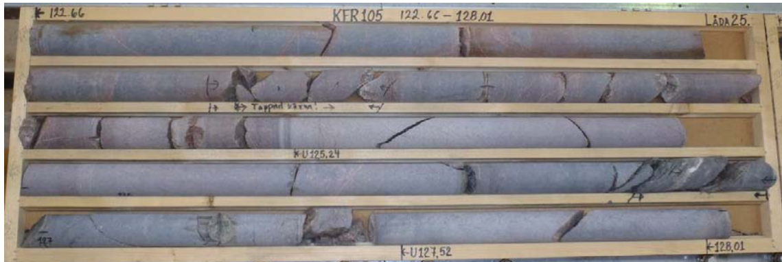
Figure 5-9. Photograph of drill core box from part of the sampled borehole section KFR105: 120.0–134.0 m.
