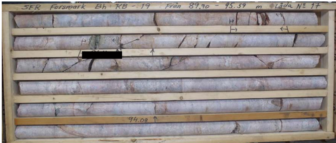
Figure A1-68. Photograph of the sampled drill core box. The sampled section is marked with a black line under the drill core.
