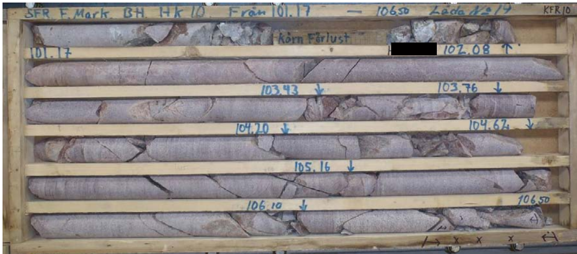
Figure A1-58. Photograph of the sampled drill core box. The sampled section is marked with a black line under the drill core.
