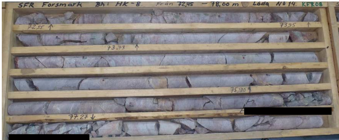
Figure A1-39. Photograph of the sampled drill core box. The sampled section is marked with a black line under the drill core.
