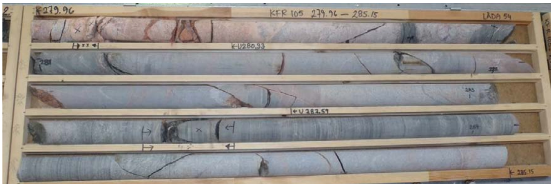
Figure 5-10. Photograph of drill core box from part of the sampled borehole section KFR105: 265.0–306.8 m.
