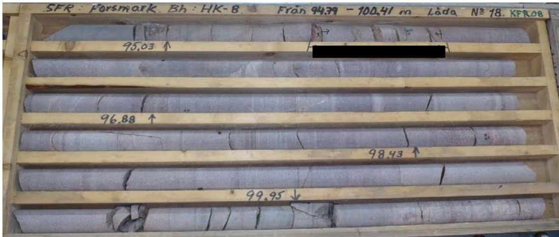
Figure A1-51. Photograph of the sampled drill core box. The sampled section is marked with a black line under the drill core.
