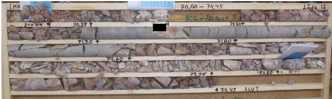
Figure A1-29. Photograph of the sampled drill core box. The sampled section is marked with a black line under the drill core.
