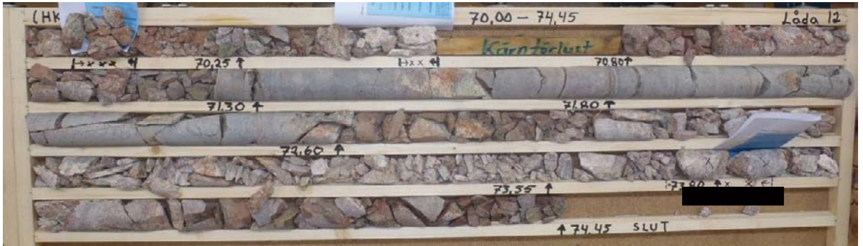
Figure A1-32. Photograph of the sampled drill core box. The sampled section is marked with a black line under the drill core.
