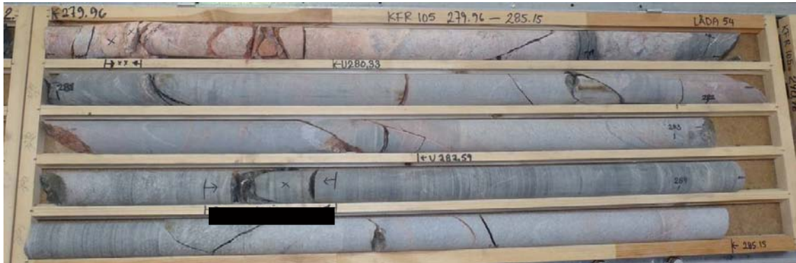
Figure A1-95. Photograph of the sampled drill core box. The sampled section is marked with a black line under the drill core.
