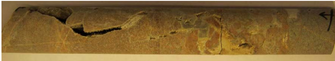
Figure A1-44. Photograph of the sampled fractures.
