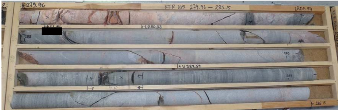
Figure A1-92. Photograph of the sampled drill core box. The sampled section is marked with a black line under the drill core.
