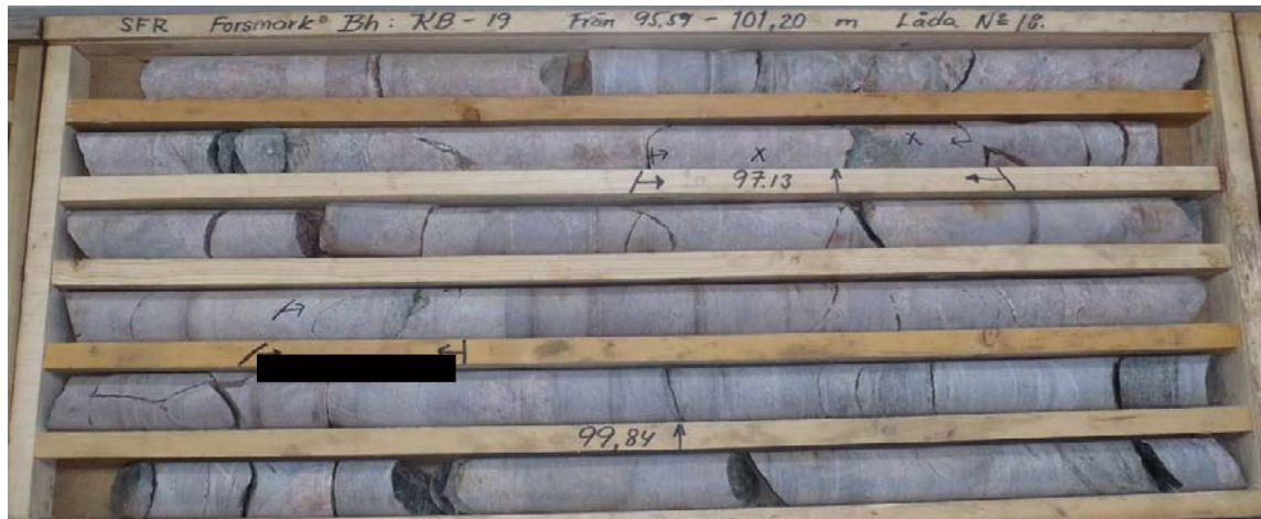
Figure A1-75. Photograph of the sampled drill core box. The sampled section is marked with a black line under the drill core.
