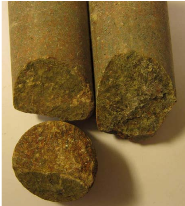
Figure A1-80. Photograph of the sampled fractures.
