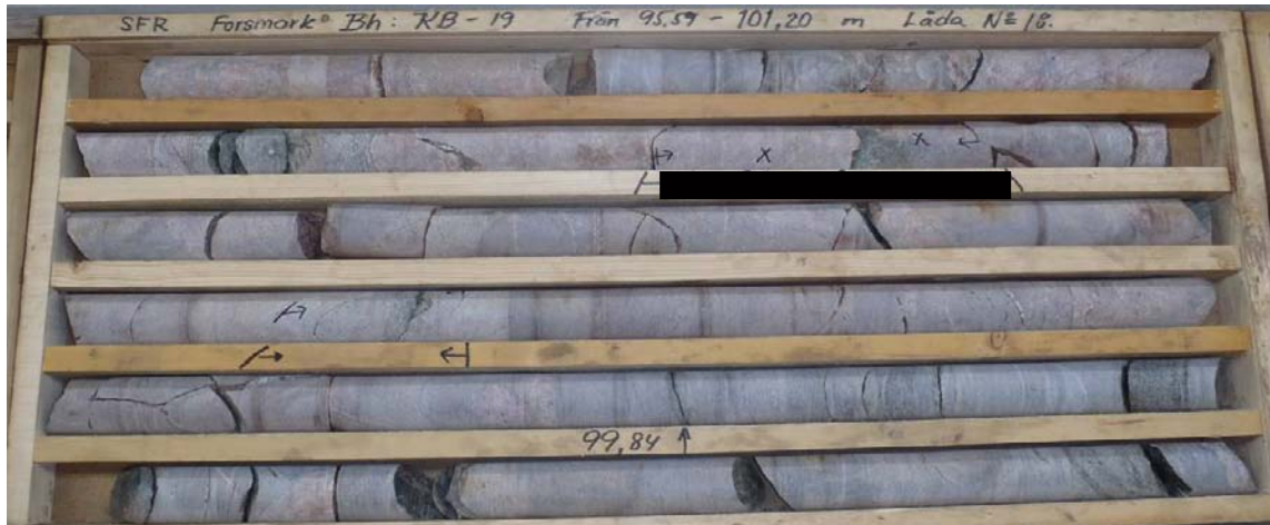
Figure A1-72. Photograph of the sampled drill core box. The sampled section is marked with a black line under the drill core.
