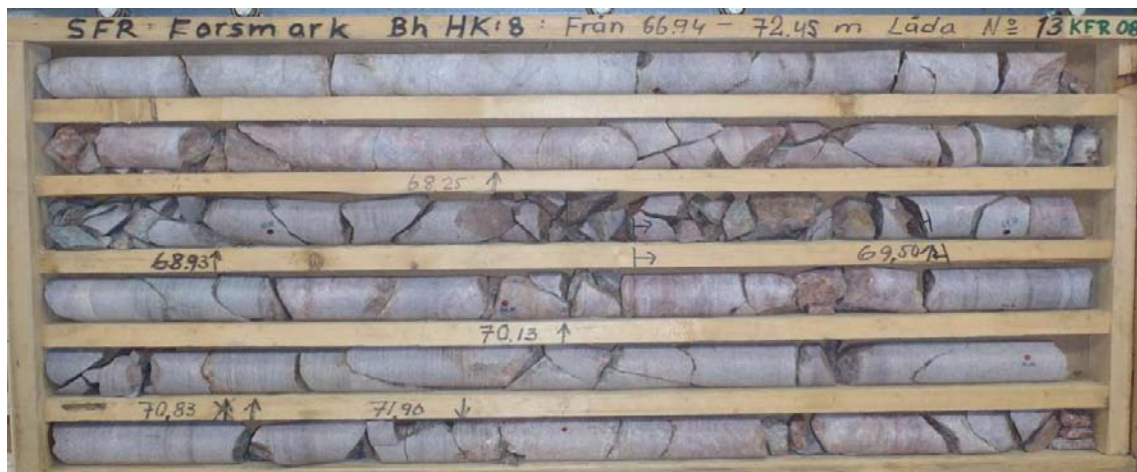
Figure 5-6. Photograph of drill core box from part of the sampled borehole section KFR08: 63.0–104.0 m.
