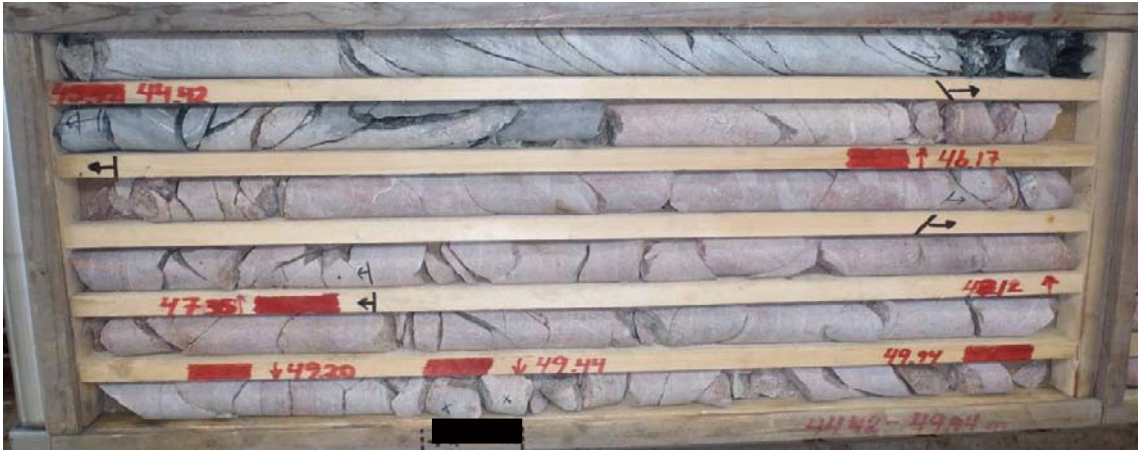
Figure A1-8. Photograph of the sampled drill core box. The sampled section is marked with a black line under the drill core.
