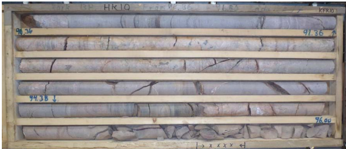
Figure 5-7. Photograph of drill core box from part of the sampled borehole section KFR10: 87.0–107.3 m.
