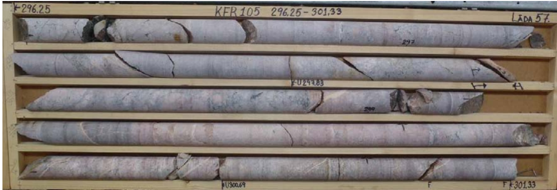
Figure A1-98. Photograph of the sampled drill core box. The sampled section is marked with a black line under the drill core.
