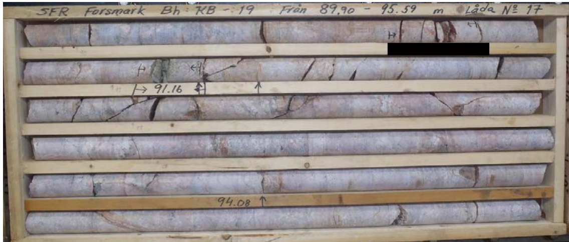
Figure A1-64. Photograph of the sampled drill core box. The sampled section is marked with a black line under the drill core.
