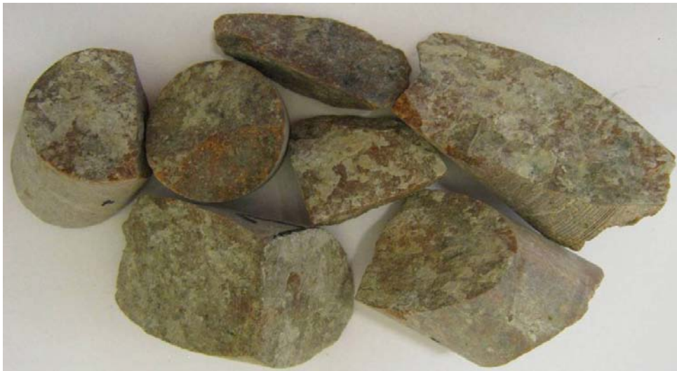
Figure A1-5. Photograph of the sampled fractures.
