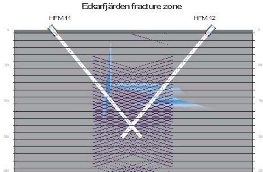
Figure 3-8. Schematic and simplified representation of boreholes HFM11 and HFM12, the Eckarfjärden deformation zone and estimated approximate locations of water yielding zones.
