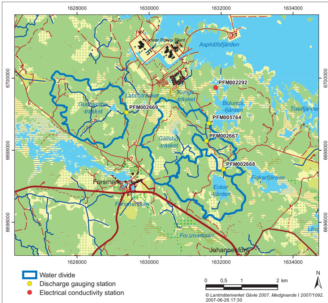
Figure 3-4. Location of the four discharge gauging stations and the electrical conductivity monitoring station (PFM002292) in Forsmark.
