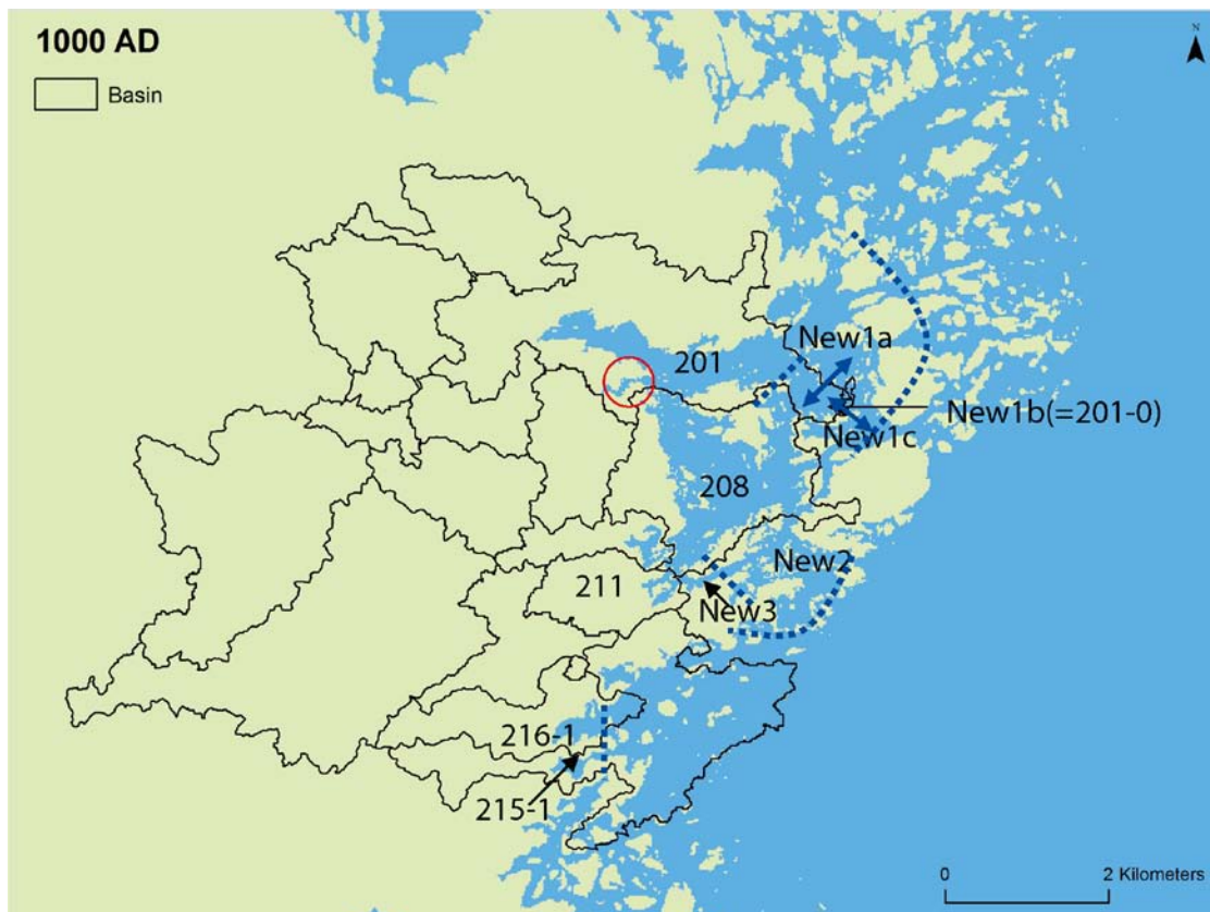
Figure A-5a. Delimitation of the coastal basins with the shoreline of the year 1000 AD. Three new basins needed to be added. SB New1 has several strait connections to BO 201 and 208 and its elongated character is rendered by presenting (but not computing) it as three SBs. New1a through New1c. For practical computing reasons the SB New1b which consists of the outer part of BO 201 (coincidental with 201-0) has thus been treated as conjoined with the other two fjord branches of SB New1. The arising small embayment indicated by a red circle has been omitted because it is not associated with any exit points.
