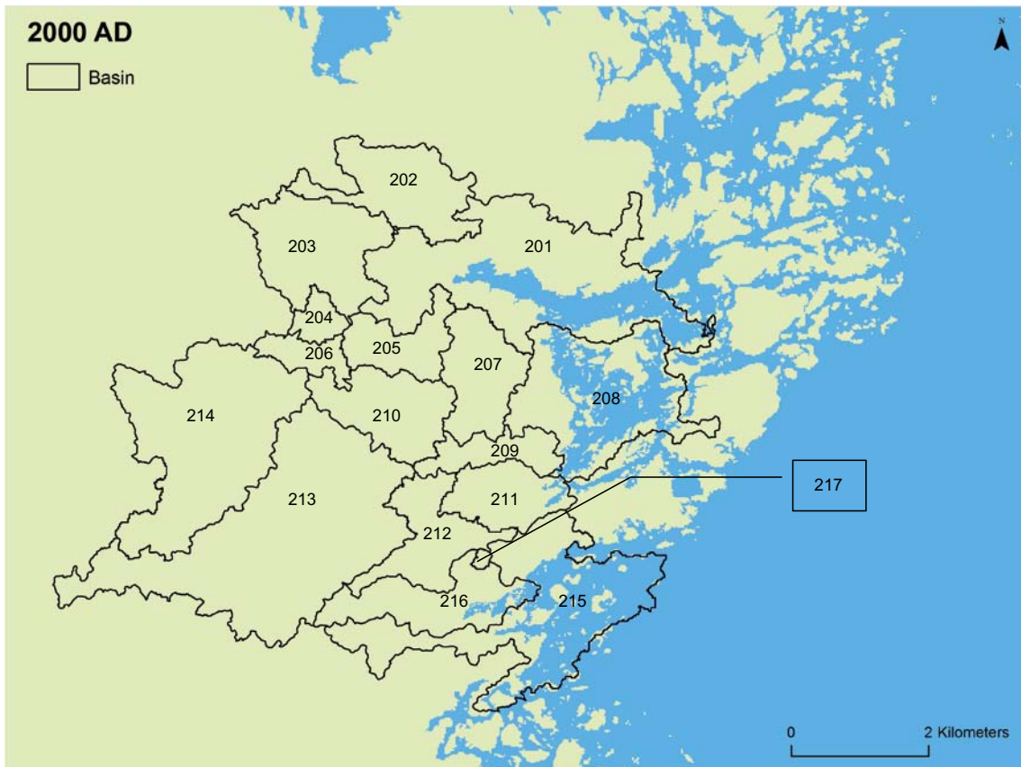
Figure 1-1a. Subdivision into biosphere object (BO) basins enumerated 201 through 216 against the background of the contemporary coastal shoreline (2000AD) when the sea level is 1m above the yearly mean water level (MW). The minute BO 217 was defined on an early stage of the study but was subsequently conjoined with BO 216.
