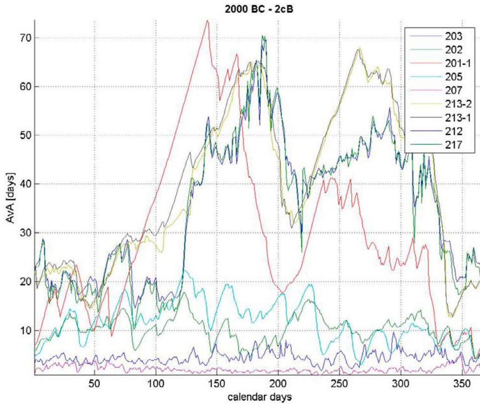
Figure B-2. Graphical rendering of the AvA-computation for 2000 BC. All involved SBs attain quasi-stationary levels. The seasonal variance is accentuated for the subsequently conjoined basins of the BOs 202 and 203.
