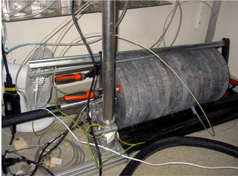
Figure 2-7. Lead shield with PEEK tubing and parts of the HPGe-detector used for on-line radioactivity concentration measurements. The fan was installed to avoid condensation on the detector's heat exchanger.
