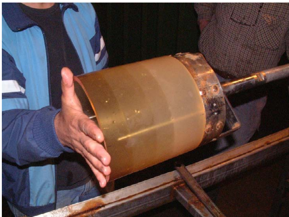
Figure A1-1. Polyurethane cylinder (mounted on lead-in equipment).
