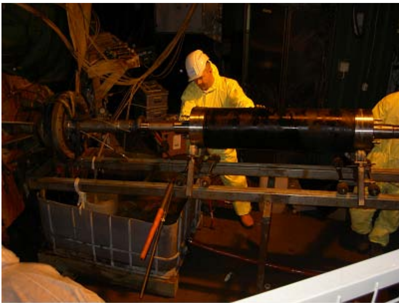
Figure 3-4. Dismantling of borehole equipment showing water collection container below the borehole collar where water was sampled and monitored for \gamma -radiation. The hydraulic packer is being dismantled.
