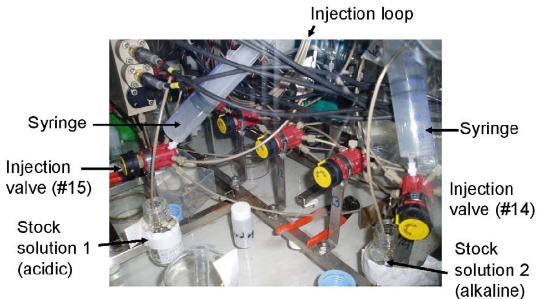
Figure A2-2. Injection valves photograph with tubes to stock solution bottles, syringes and one injection loop visible behind the left syringe. The photo is from a pre-test. In the LTDE-SD injection, 20 ml plastic vials were used for the stock solutions and the vials were placed in lead shields.
