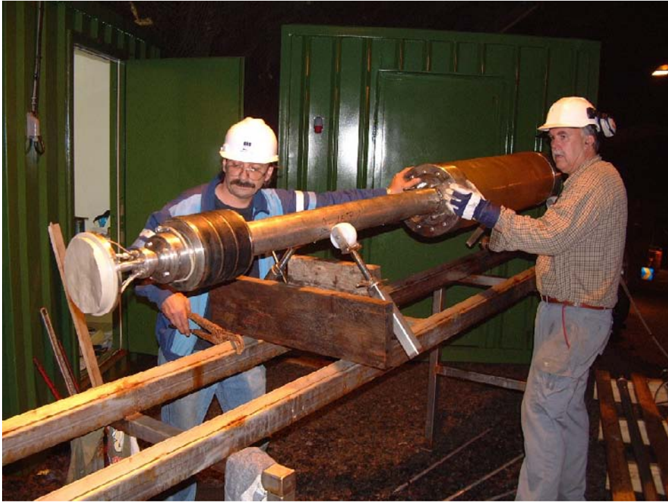
Figure A1-5. Mounted PEEK lid, mechanical and hydraulic 300 mm packers.
