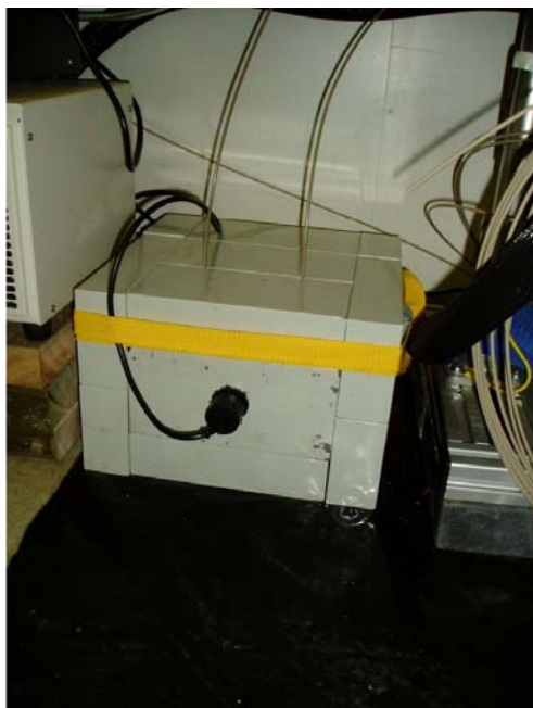
Figure 2-8. Lead shield and back part of the GM-probe used for on-line dose rate monitoring.
