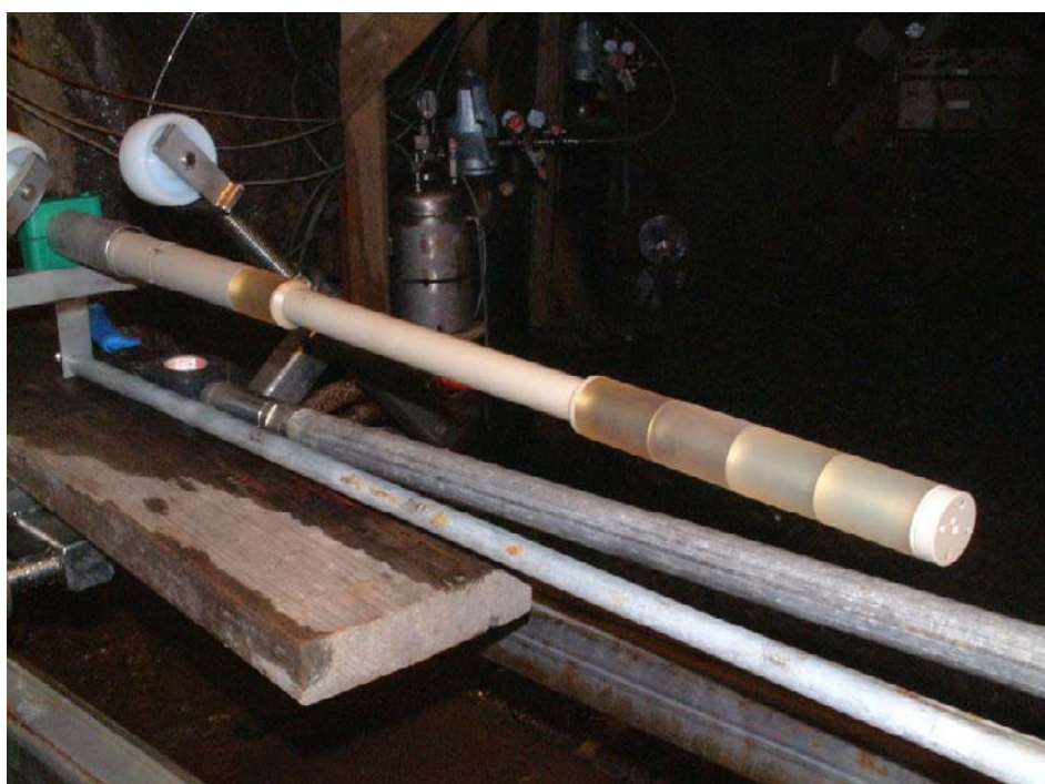
Figure A1-2. 36 mm borehole packer and dummy.
