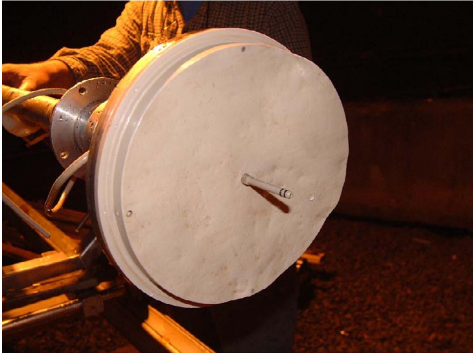
Figure A1-3. PEEK lid with connection to 36 mm borehole equipment.
