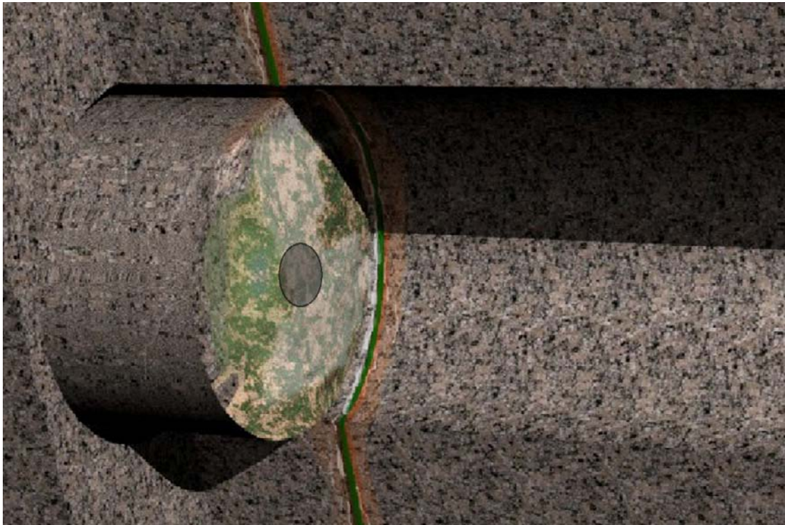
Figure 1-3. Illustration of the ~14cm long and 177 mm diameter core stub in Ävrö granodiorite exposing a natural fracture surface in borehole KA3065A03. The fracture surface is partly covered by relative thin layers of calcite (white) and chlorite (green) /Nilsson et al. 2010/. The 36 mm borehole is indicated in the centre of the stub. Illustration from /Winberg et al. 2003/.
