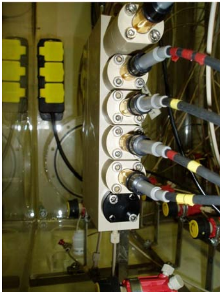
Figure 2-9. Electrochemical flow cell used for on-line measurements of pH and E_h .
