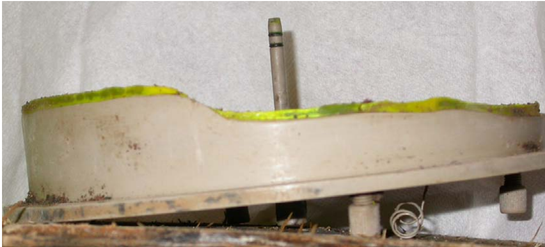
Figure 2-7. The post-experimentally injected epoxy surface covering the PEEK-disc that accidentally loosened from the fracture surface.
