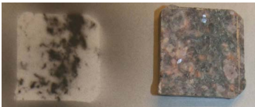
Figure 3-2. Autoradiograph of slice D7.1, cf. Figure 2-6. The blackening is interpreted to correspond primarily to the dark minerals and a single microfracture. The base of the slice is approximately 16 mm.
