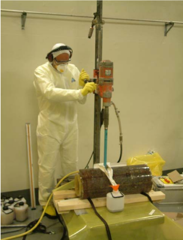
Figure 2-4. Drilling of a D core sample.
