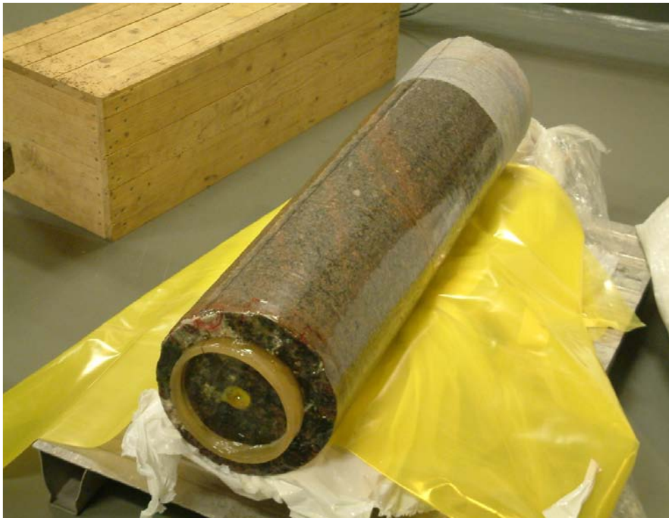
Figure 2-2. Epoxy resin coating on the 278 mm diameter core, shielding the rock in order to avoid leakage or contamination of tracers. In front is the fracture surface, where the 177 mm diameter stub is, sealed off by the PU rubber. The 36 mm diameter extension borehole can be seen in the middle. For a view of the scheme for drilling of core samples, see Figure 2-6, which shows a projection from another angle.
