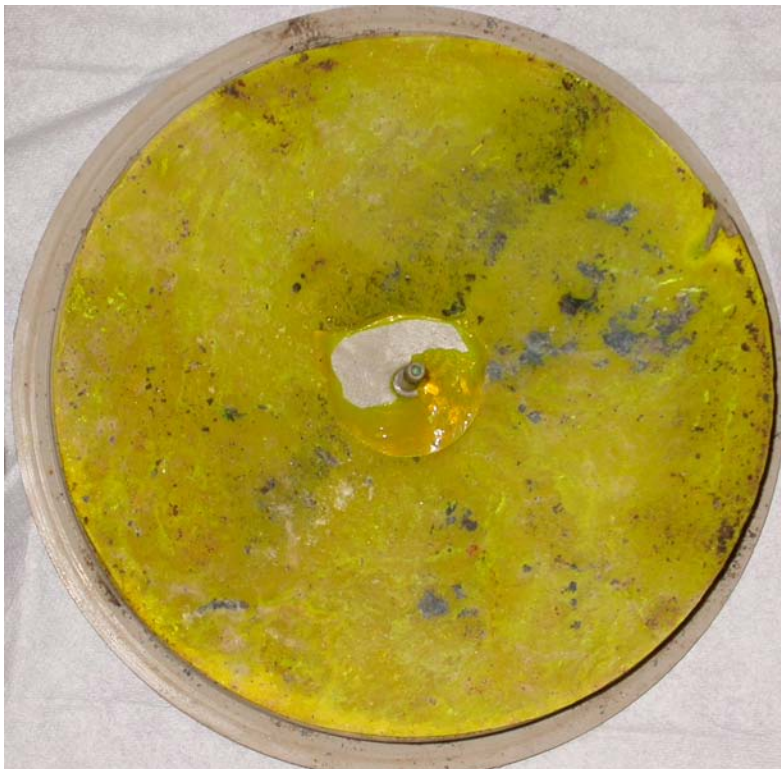
Figure 2-8. Visible fracture coatings on the epoxy surface.
