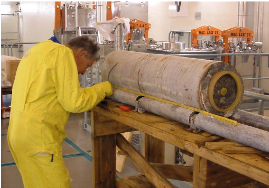
Figure A2-3. The 300 mm diameter core mapped at SKB Clab before sampling. The core stub with natural fracture is enclosed by the yellow poly urethane cylinder (to the right in the photo).
