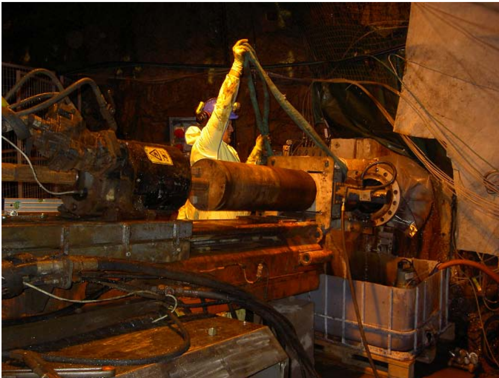
Figure 2-1. Drilling machine is prepared for 300 mm diameter over-core drilling at experimental borehole KA3065A03. Drill bit with core barrel in centre of photo. Open vessel for collecting drilling fluid beneath borehole collar.
