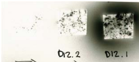
Film autoradiograph of rock slice D12.1 to D12.3 at 1 day exposure time.
