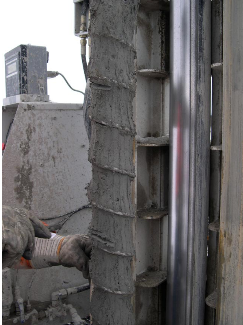
Figure 4-2. The cores were cleaned using a knife and described and sampled into plastic containers. The picture shows a section of clayey till at Storskäret (PFM002464).
