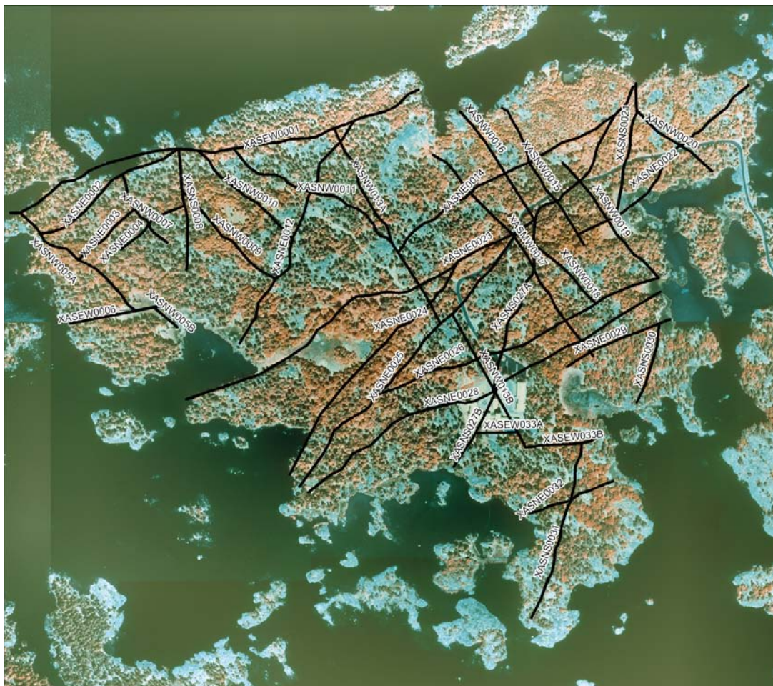
Figure 4-1. Aerial map of Äspö showing the location and id-code of the linked lineaments (black lines) presented by /Mattsson and Wahlgren 2010/.
