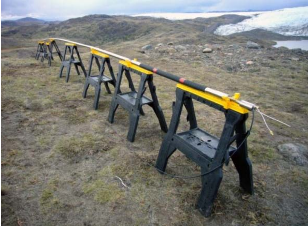
Figure 4-21. Photo of the borehole observatory showing the packer, the fluid sampling stainless steel tubes and the cable for the P/T/EC (Aqua TROLL200) sensor. The BO is connected to the deployment string, i.e. sampling and heating lines before lowered into the borehole. Total length of the BO is 12 metres. Photo by Anne Lehtinen.
