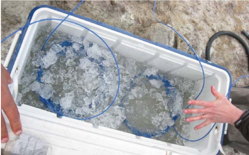
Figure 4-32. Loop of fibre optical cable is immersed into an ice-bath in order to obtain a reference temperature for the DTS-measurements. Photo by Emily Henkemans.
