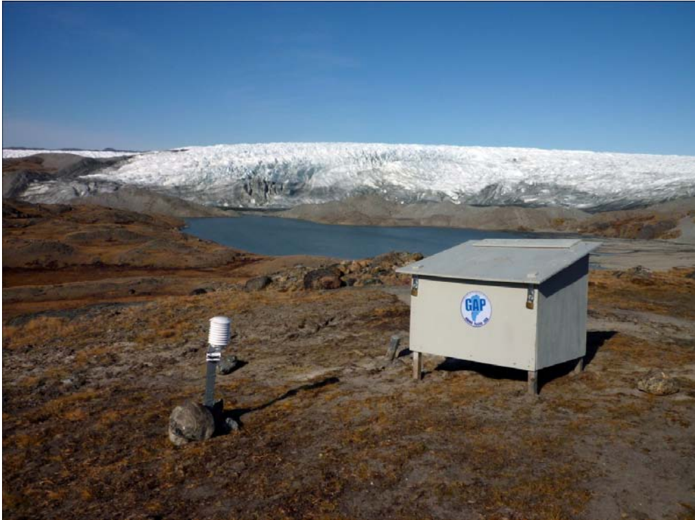
Figure 4-24. Pressure and temperature logging station beside the DH-GAP03 borehole. Photo by Lillemor Claesson Liljedahl.
