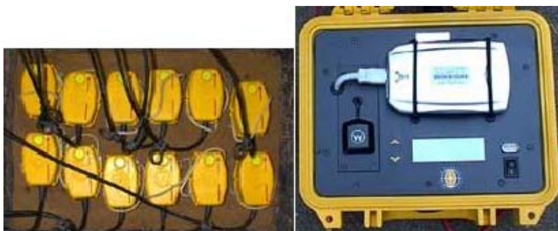
Figure 2-45. Passive seismic equipment including (Left): three-component geophones to be installed at the ice surface, connected to (Right): SAQS passive seismic data loggers.
