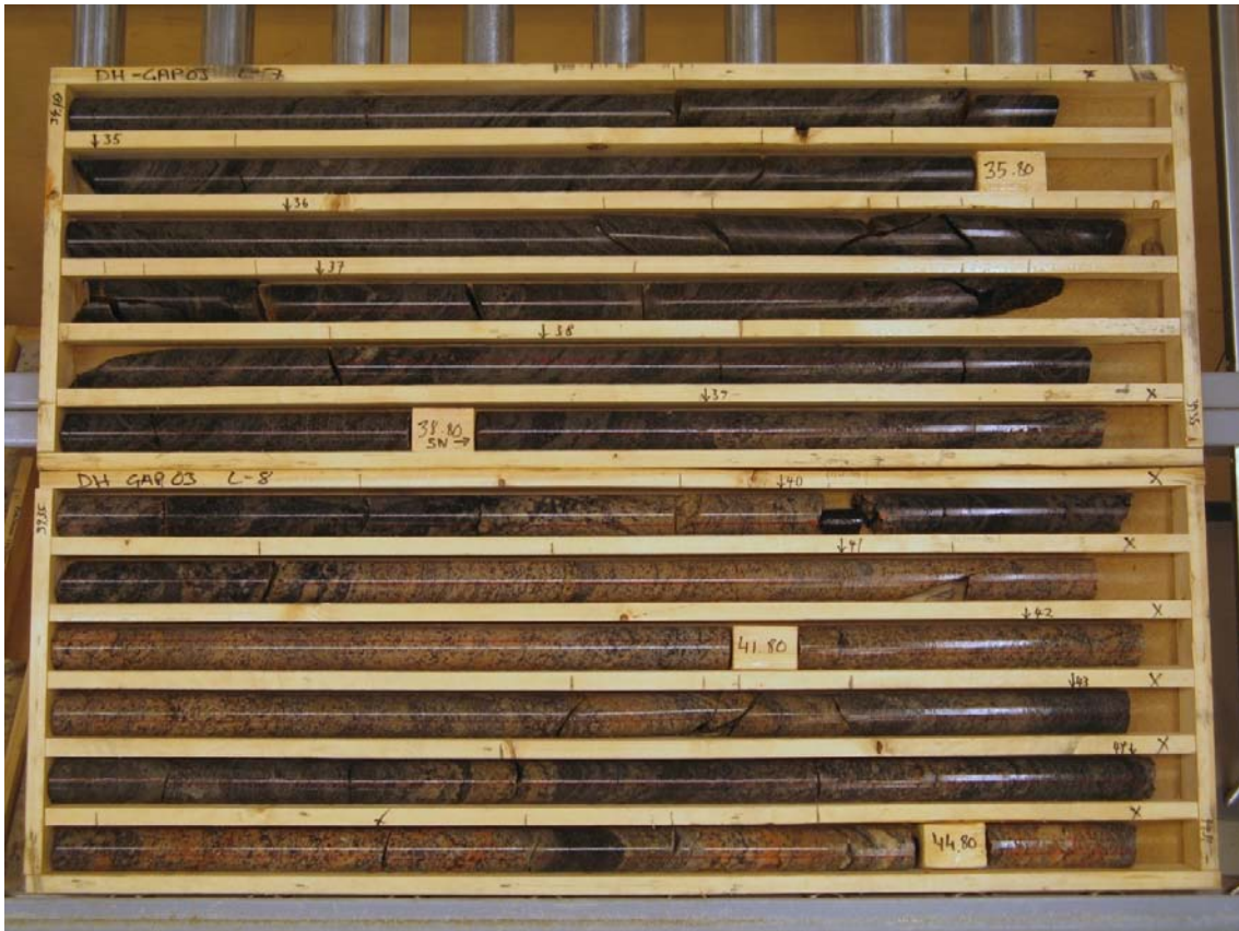
Figure 4-13. Transition from mafic and/or amphibole-rich gneisses to felsic gneisses in DH-GAP03, 34.10–44.91 m. Photo by Tuomas Pere.
