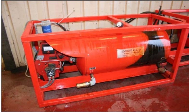
Figure 4-3. Flushing water heater. Photo by KATI OY.
