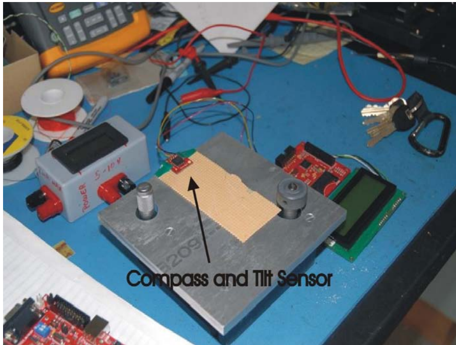
Figure 3-9. Compass and tilt (inclinometer) module under laboratory testing (the module is the 2 cm red square). This module forms the core of the ice deformation string, which will consist of 40 individual inclinometer modules. The module is being tested on a specially made micrometer tilt plate. The surrounding electronics are prototypes of the control, power and data-logging electronics, which are also developed in-house. Photo by Joel Harper.
