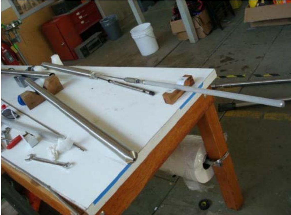
Figure 4-23. Photo showing the bull nose equipment (i.e. the Aqua TROLL 200 with P/T/EC sensors at the check valve, below which the sintered stainless steel 40 \mu\text{m} filter is connected). The conductivity sensor in the Aqua TROLL 200 is calibrated during manufacturing, and the specific conductivity reading was checked without remarks before the BO was assembled. Photo by Barry Freifeld.
