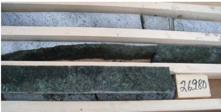
Figure 4-14. A typical “greenish” fracture surface in DH-GAP03, located at 269 m of borehole length. Photo by Jon Engström.
