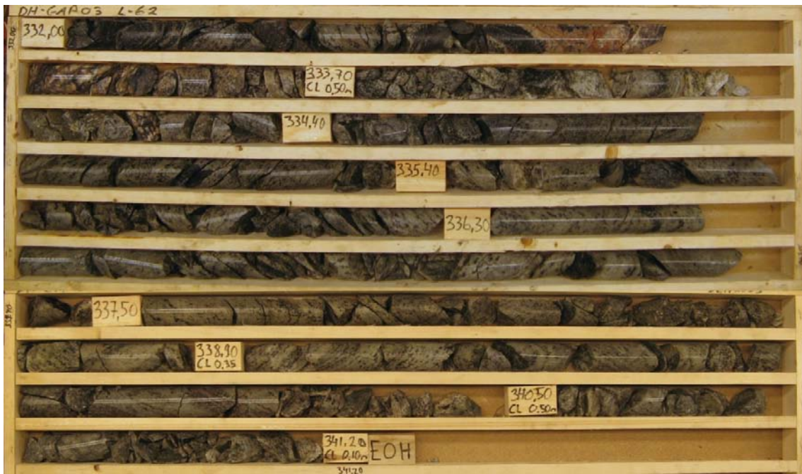
Figure 4-8. Highly fractured zone at 331.70–340.50 m, which terminated the drilling of DH-GAP03. Photo by Timo Ruskeeniemi.
