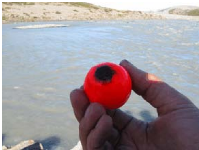
Figure 2-52. Photo of the electronic tracer. Photo by Jemma Wadham.
