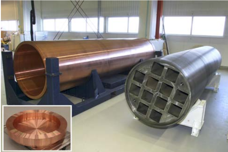
Figure 1-6. Copper canister with nodular iron insert (the inset photo shows the copper lid).
