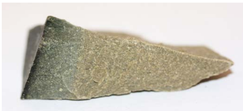
Figure 24-15. A sample from a block in the ABM test at the Äspö HRL, with a distinct reaction zone between iron and bentonite. The sample is about 4 cm long.
