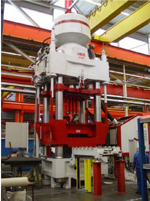
Figure 13-2. Commercial press for block fabrication.
