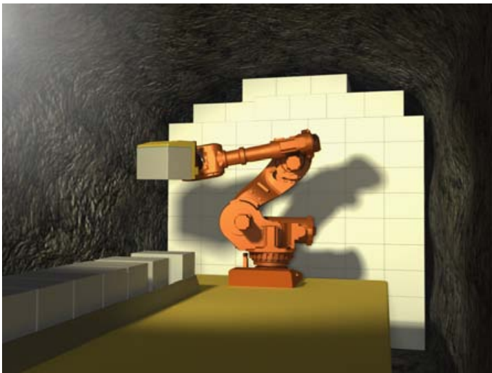
Figure 13-4. Robot for installation of backfill blocks.
