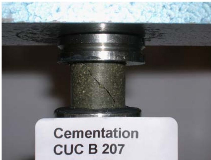
Figure 24-16. Example of a uniaxial compression test. The sample is loaded with a constant deformation rate in the axial direction to failure. Axial stress and strain are measured. From /24-28/.
