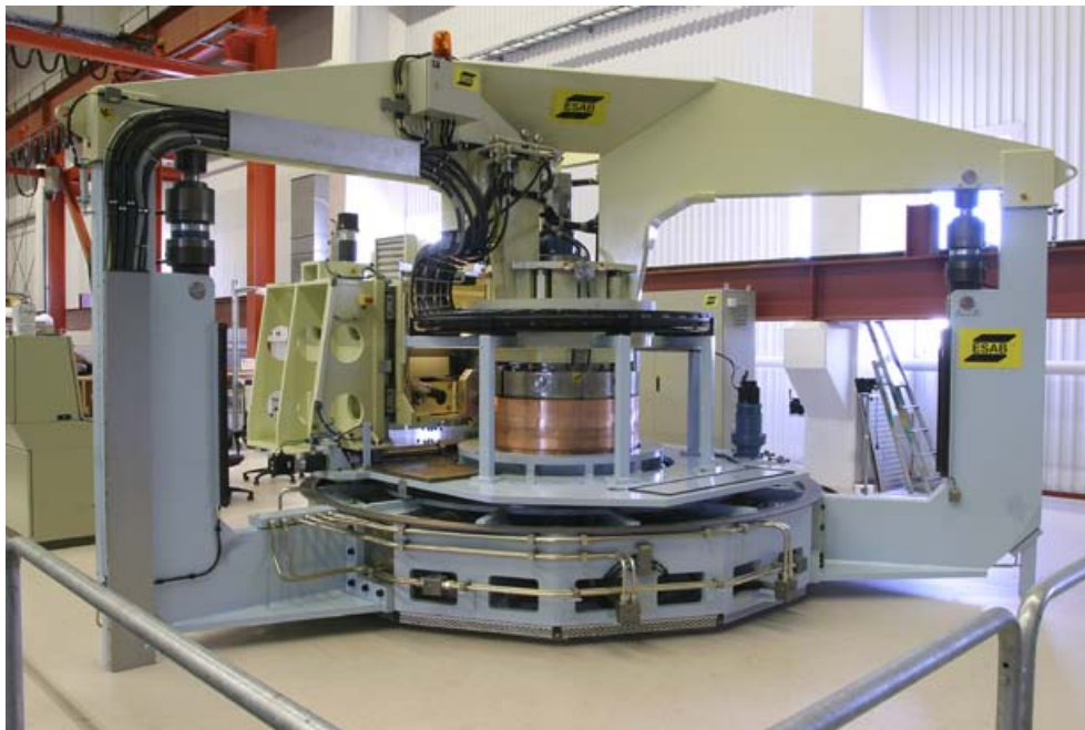
Figure 1-11. The Canister Laboratory's equipment for development of friction stir welding.
