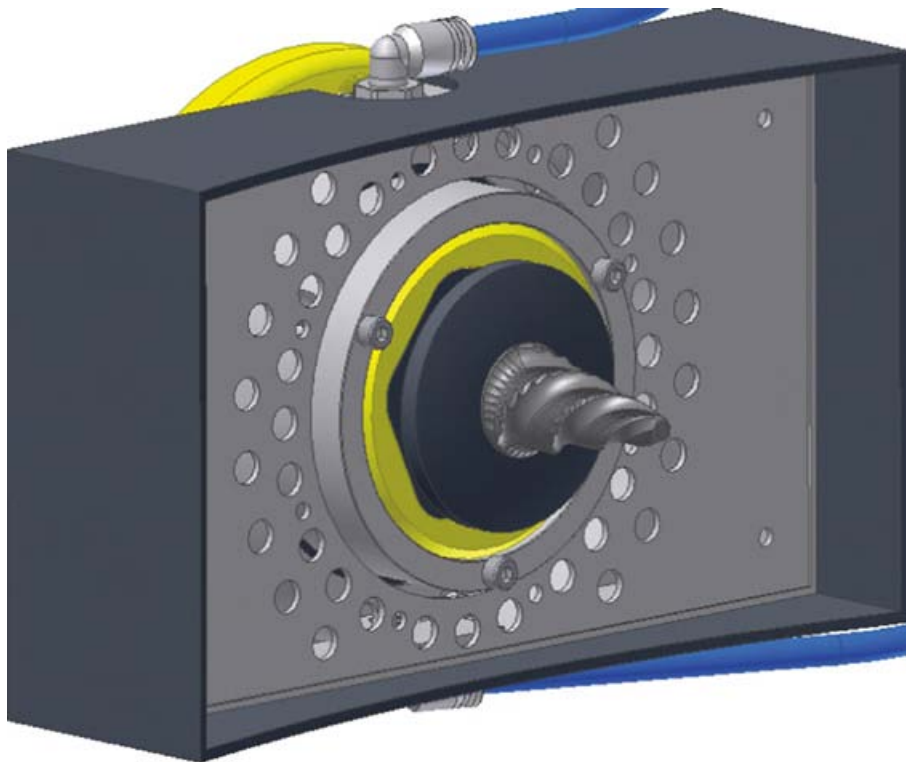
Figure 11-6. Illustration of the new shielding gas chamber.
