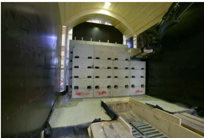
Figure 13-5. Stacking tests performed at the Bentonite Laboratory on Äspö.
