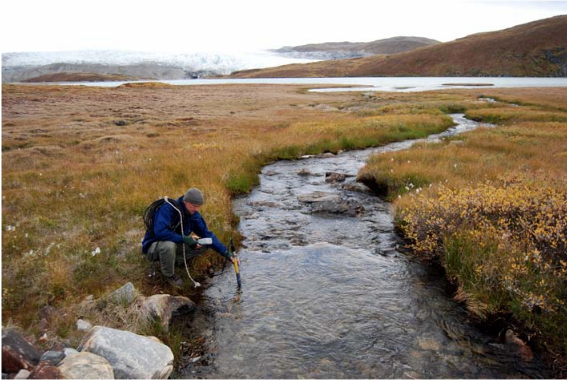
Figure 26-6. Conductivity is measured as a part of an attempt to characterize the origin of the surface water. The work was done during a field week with pilot studies in a periglacial environment near Kangerlussuaq, Greenland, in the summer of 2008.
