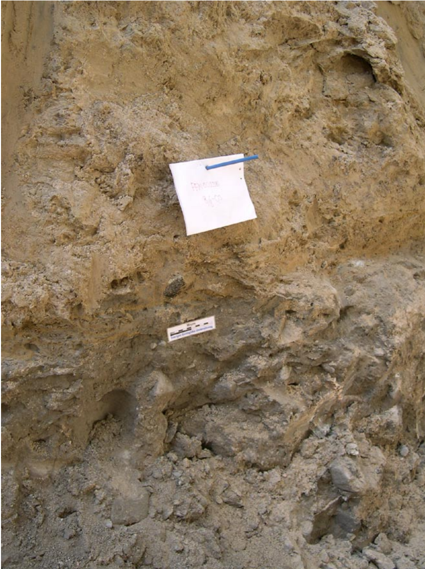
Figure 5-1. Sandy till overlaying till of clayey composition, the till beds are separated by an erosive, sharp contact (PFM002581).
