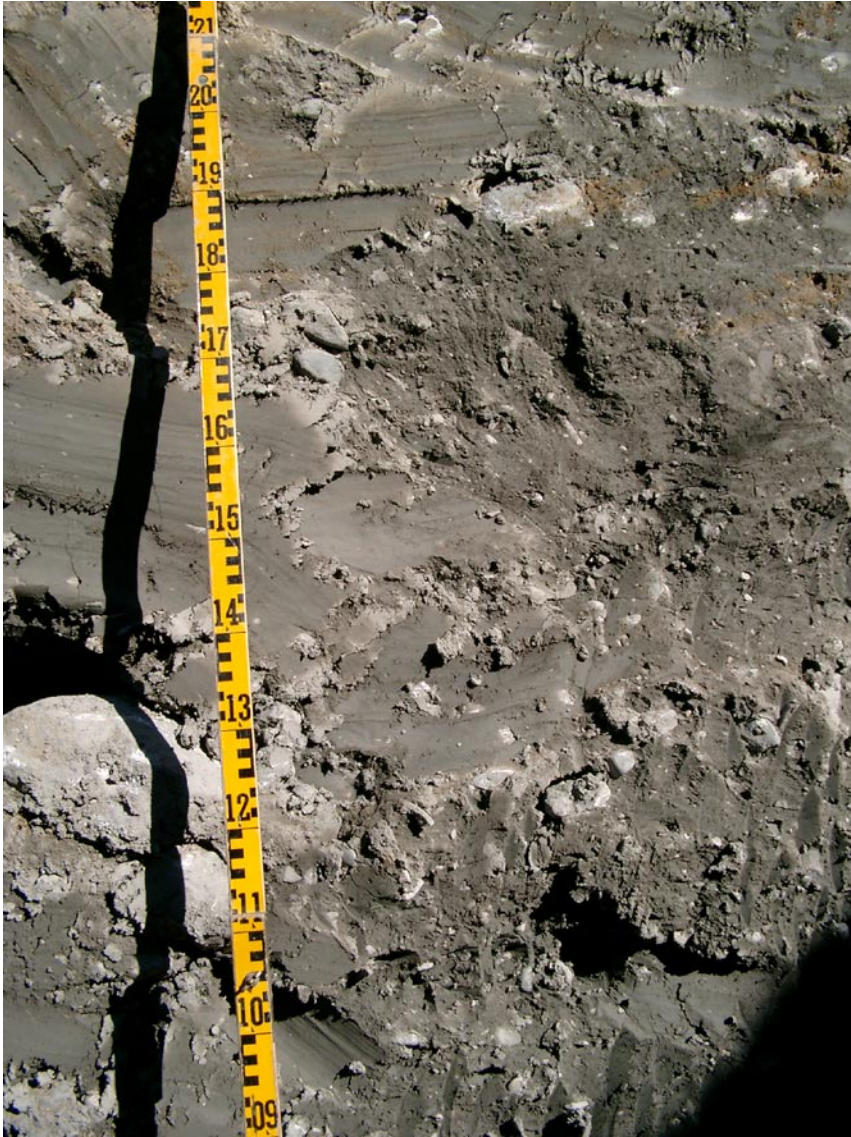
Figure 5-2. The clayey till often constitutes of compact, homogeneous boulder clay in the area around Storskäret (PFM002592).
