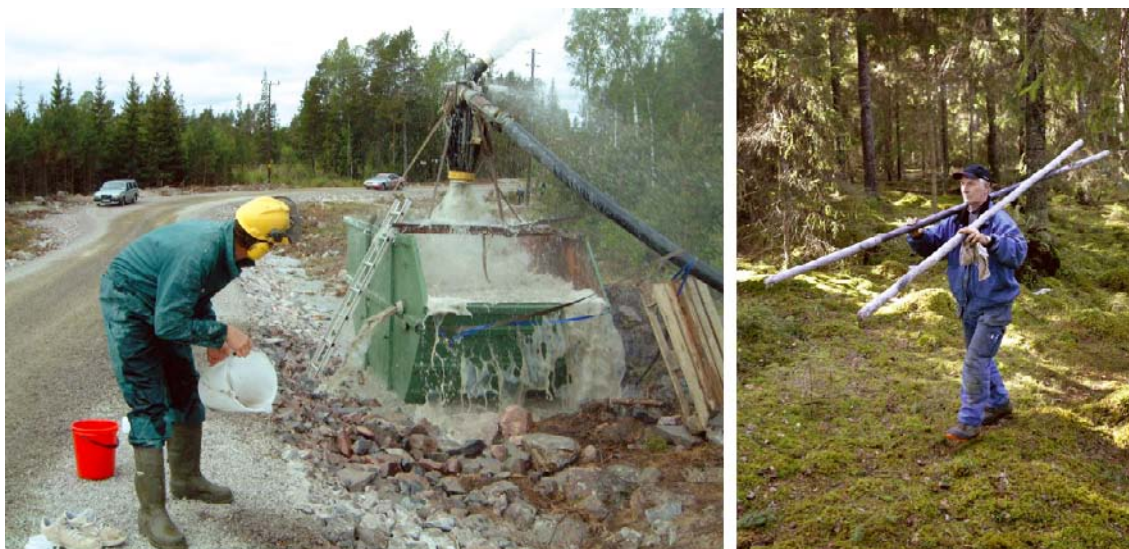
Figure 3-2. Two key features of the bedrock in the target area at Forsmark. Left: High water yields are often observed in the uppermost c. 150 m of the bedrock. Right: The large number of unbroken drill cores gathered at depth support the observation of few flowing test sections in the deeper bedrock. (Figure 10-1 in /Follin 2008/.)
