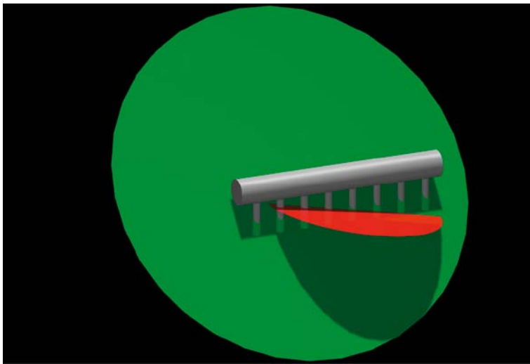
Figure 4-11. Definition of EFPC (Expanded Full Perimeter Criterion). A potentially discriminating fracture can remain undetected despite the use of the FPC in the deposition tunnel. (Figure 5-2 in /Munier 2006/.)
