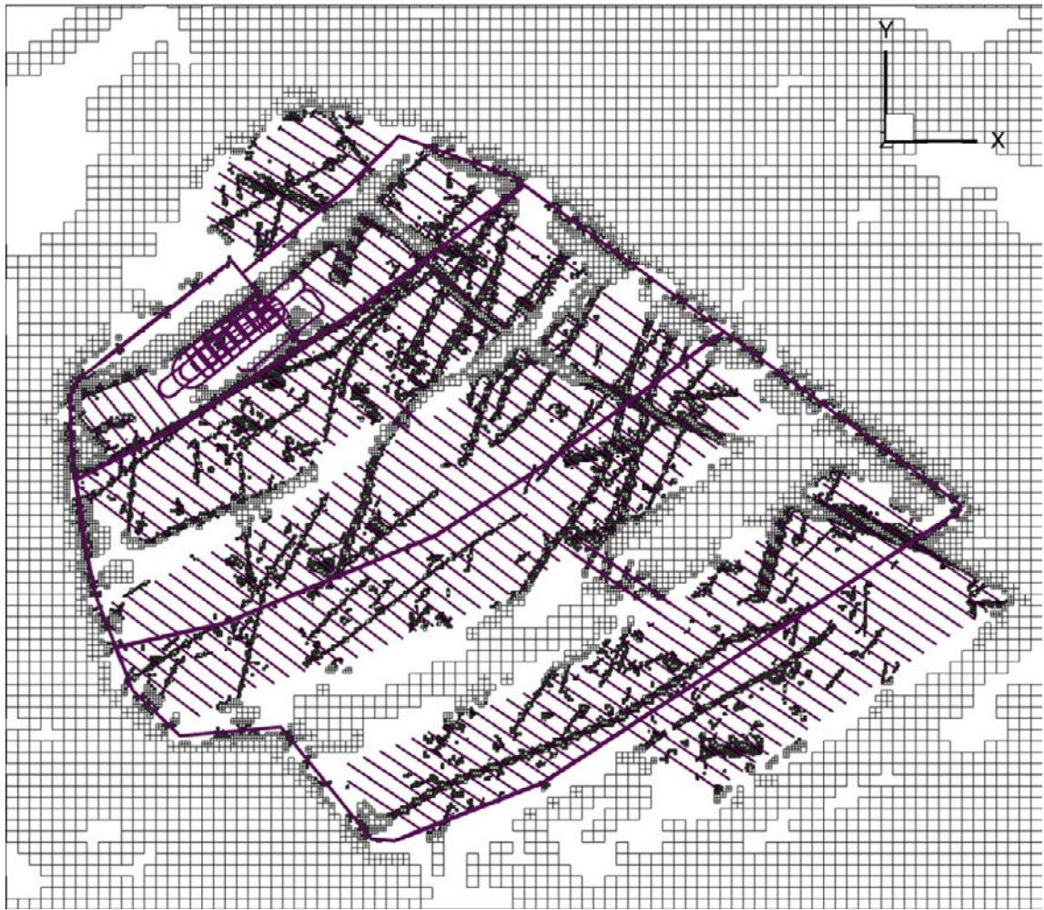
Figure E-2. Plane view of the computational grid in proximity of the repository at -472 m elevation using the EDPM approach. The discretisation around the repository is refined using an unstructured grid. The smallest grid size in this model is 0.5 m.
