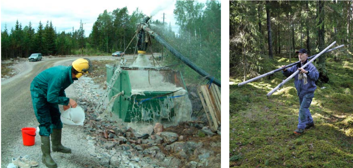
Figure 2-2. Two key features of the bedrock in the target area at Forsmark. Left: High water yields are often observed in the uppermost c 150 m of the bedrock. Right: The large number of unbroken drill cores gathered at depth support the observation of few flowing test sections in the deeper bedrock. (Source: Figure 10-1 in /Follin 2008/.)
