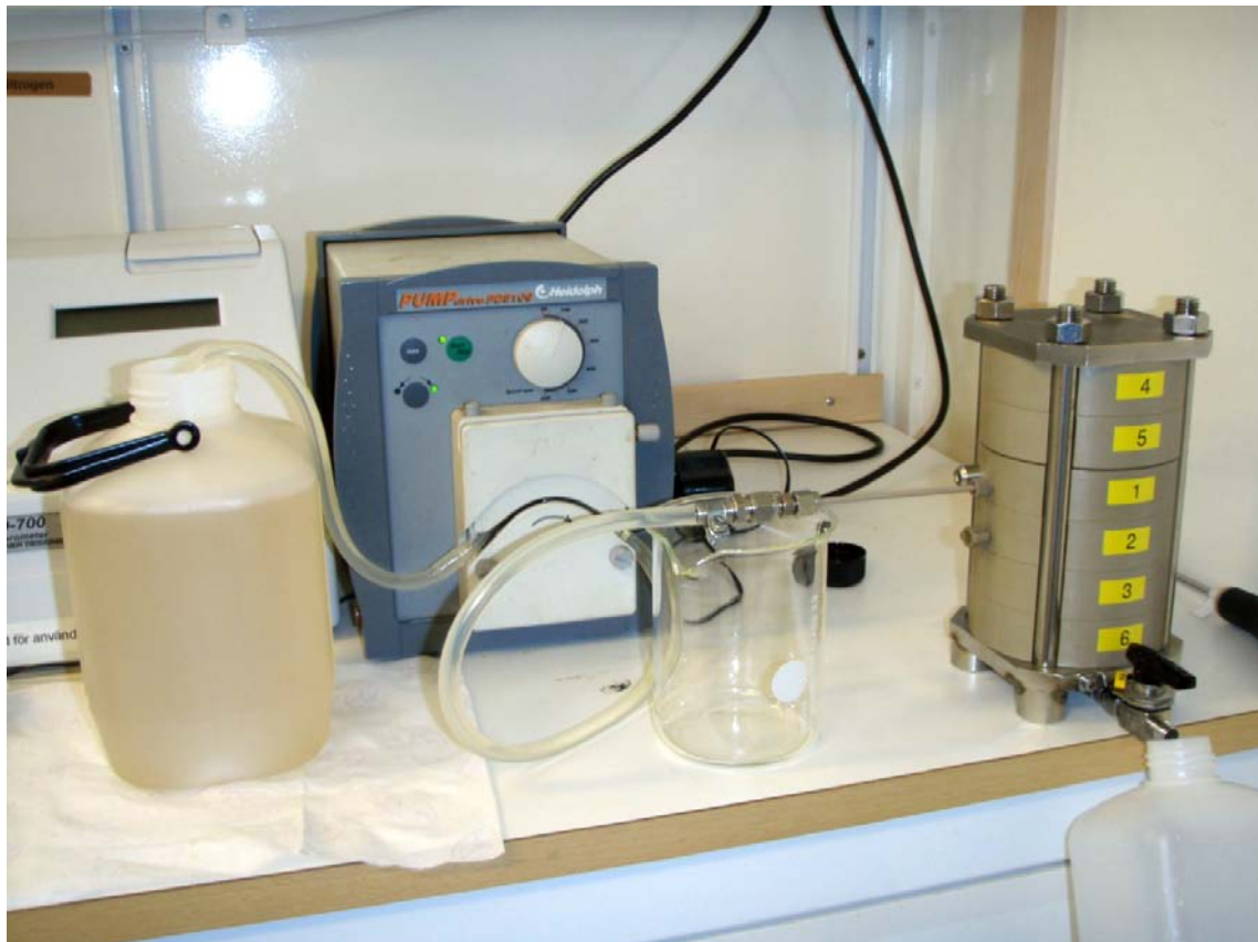
Figure 3-3. Equipment for filtering surface water through the filter unit (to the right in the picture). Test run number 2 with three membrane filters.
