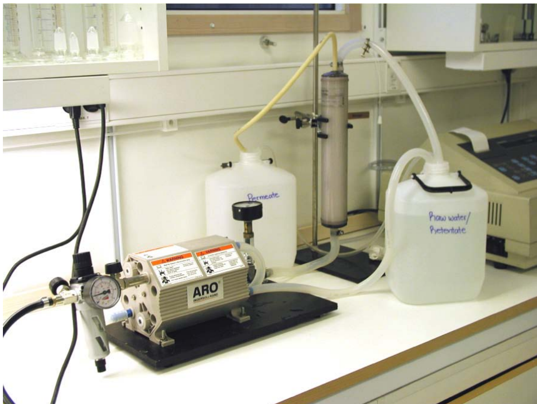
Figure 3-1. Equipment for fractionation of humic and fulvic acids.
