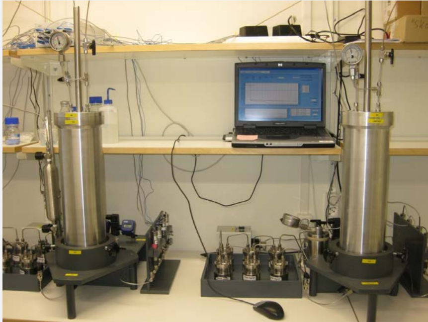
Pressure resistant micro-electrodes are used to analyse redox and pH in the circulation systems.
