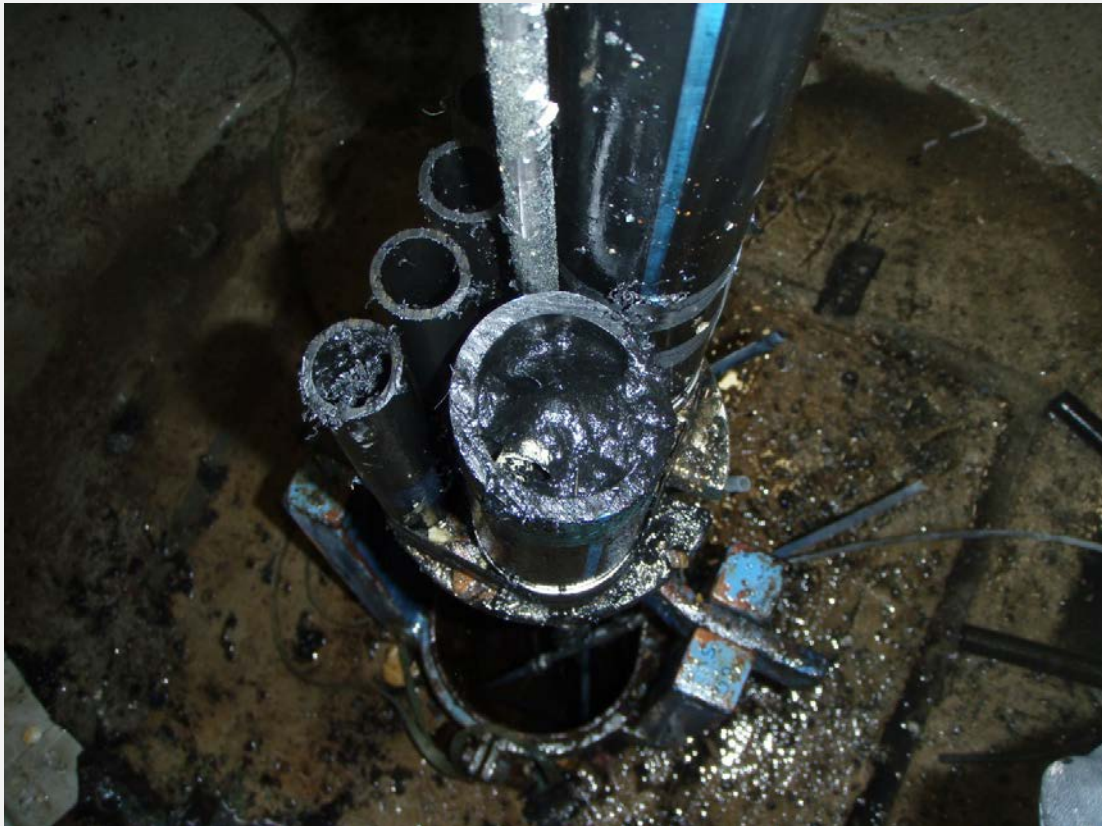
Black precipitate and a strong smell of hydrogen sulphide gas in the standpipes of borehole KAS03. The borehole equipment (iron bars, plastic tubing and rubber packers) was installed more than 20 years ago for groundwater and pressure monitoring purposes.
