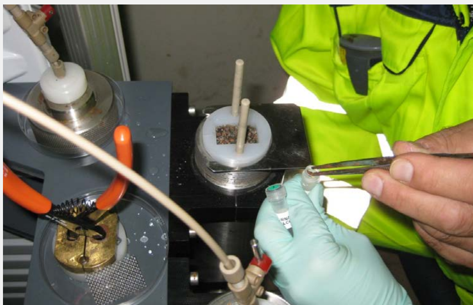
Sampling of rock pieces that have been exposed in a flow cell to circulating groundwater in one of the circulation systems on the Microbe site. Subsequently, DNA analysis reveals amount and types of microorganisms that have attached and grown on the rock pieces.
