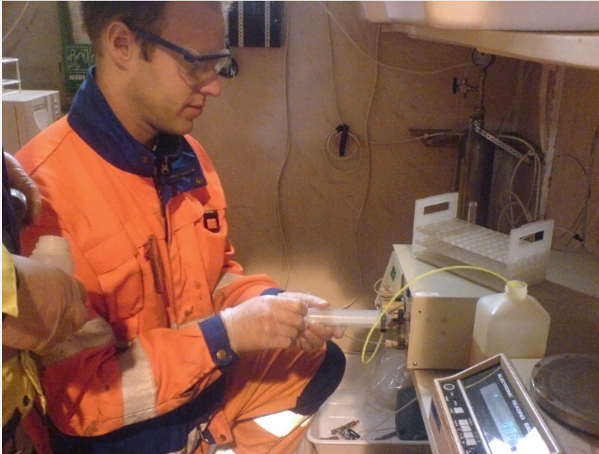
Injection of tracer in fracture.
