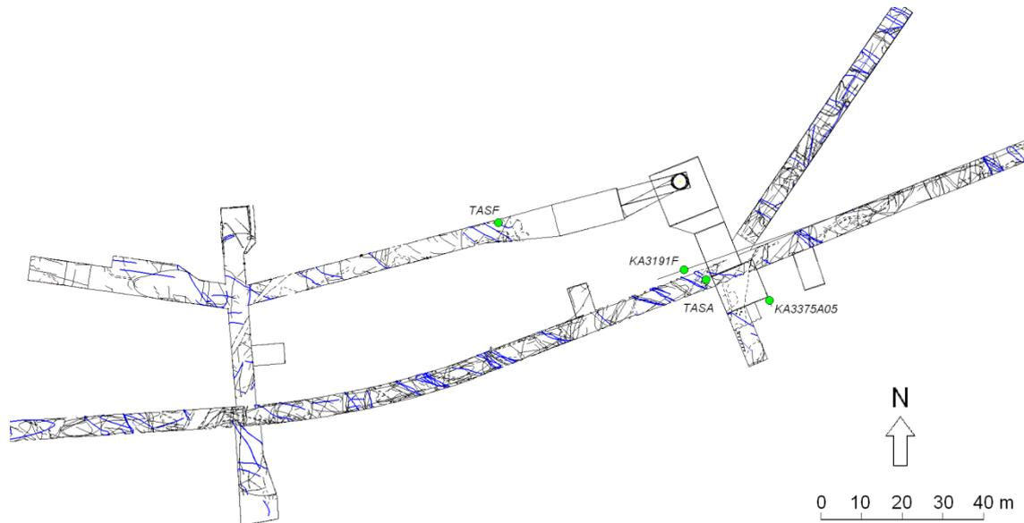
**Figure A 3.** Observation points used to model FASEW002a in tunnels and boreholes.
