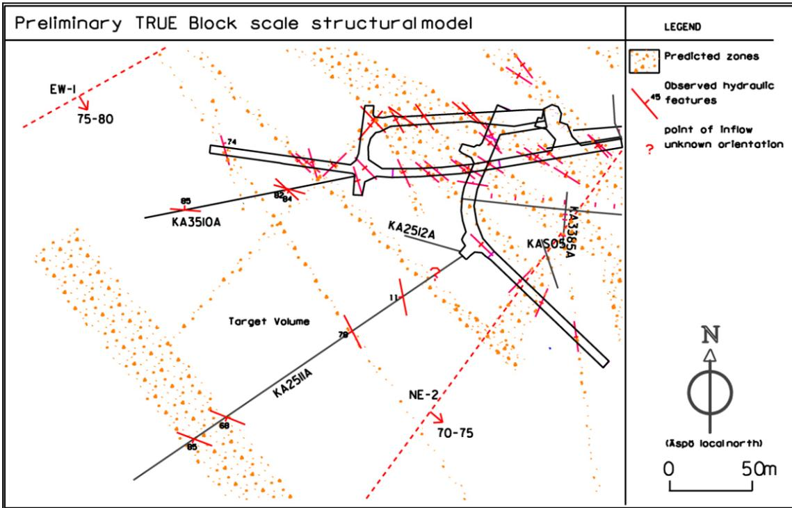
**Figure 2-2.** A preliminary structural model of the proposed experimental area for the TRUE Block Scale experiment. From /Andersson et al. 2002/.
