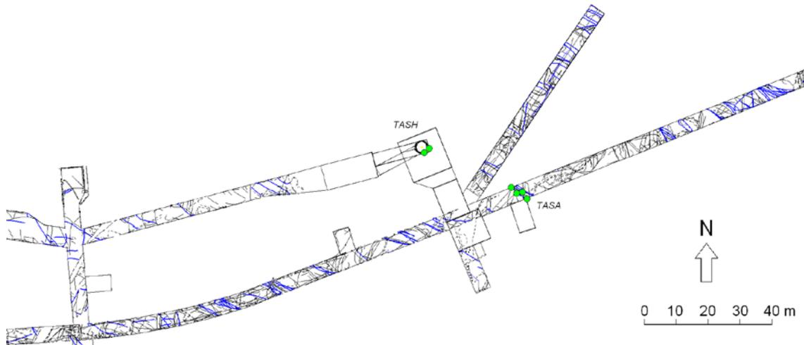
**Figure A 38.** Observation points used to model FASNW011b in tunnel and shaft.
