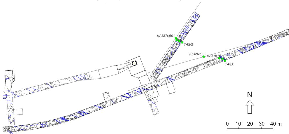
**Figure A 30.** Observation points used to model FASNW008 in tunnels and boreholes.
