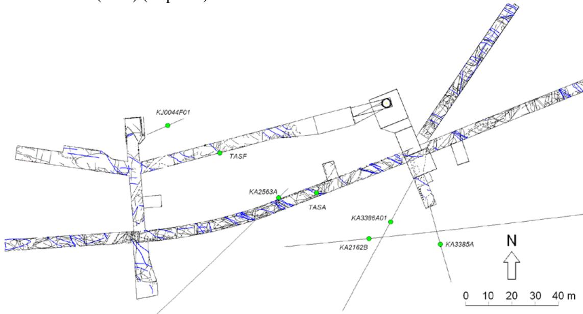
**Figure A 44.** Points used to model FASNW013 in tunnels and boreholes.
