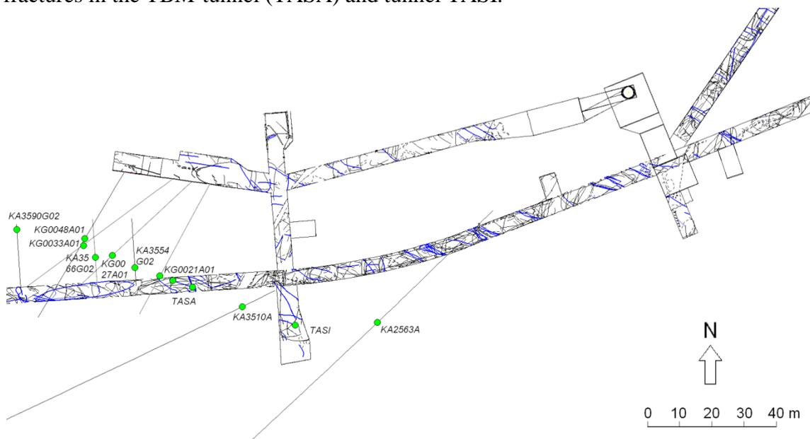
**Figure A 68.** Observation points used to model FASNW021b in tunnels and boreholes.
