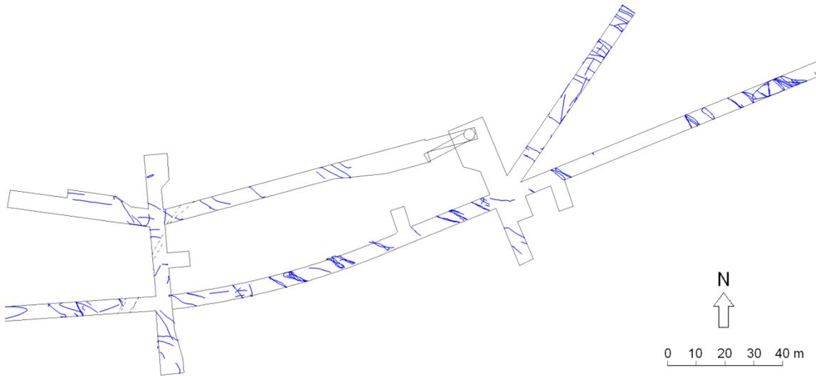
**Figure 3-2.** Tunnel mappings from the TMS system. Only water-bearing structures are shown (in blue).
