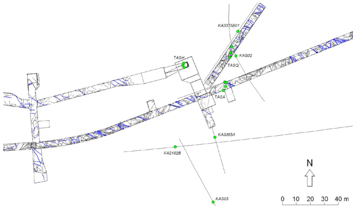
**Figure A 14.** Observation points used to model FASNS002 in tunnels and boreholes.
