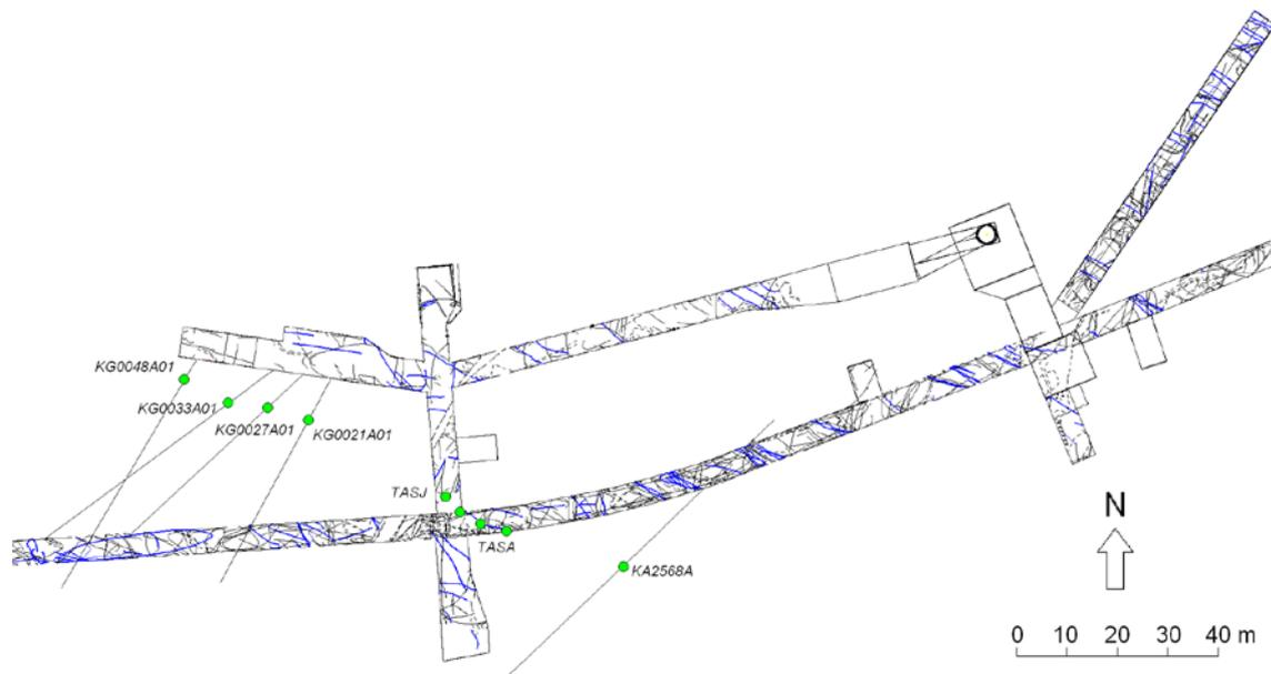
**Figure A 58.** Observation points used to model FASNW018 in tunnels and boreholes.
