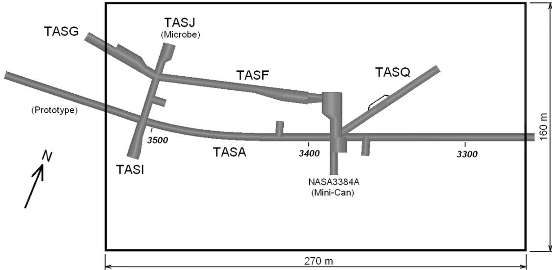
**Figure 1-2.** Top view of the model volume. Origin: Easting ( $x$ ) = 1551265, Northing ( $y$ ) = 6367676, Elevation ( $z$ ) = -500 Extent:  $dx = 270$  m,  $dy = 160$  m,  $dz = 150$  m. Y-axis bearing:  $338^\circ$  from RT90 north.
