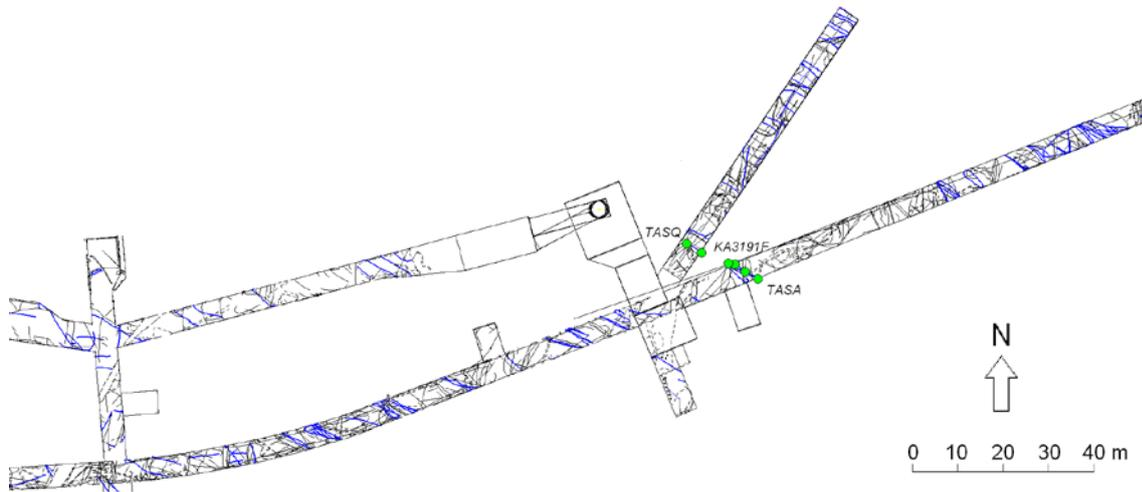
**Figure A 36.** Observation points used to model FASNW011a in tunnels and boreholes.
