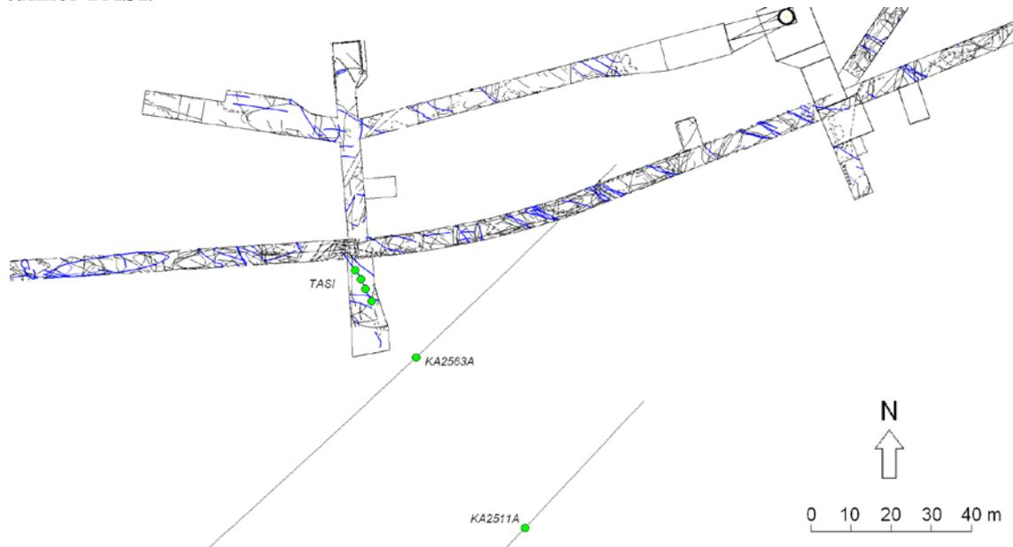
**Figure A 62.** Observation points used to model FASNW019s in the TASI tunnel and boreholes.
