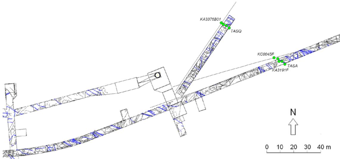
**Figure A 24.** Observation points used to model FASNW005 in tunnels and boreholes.
