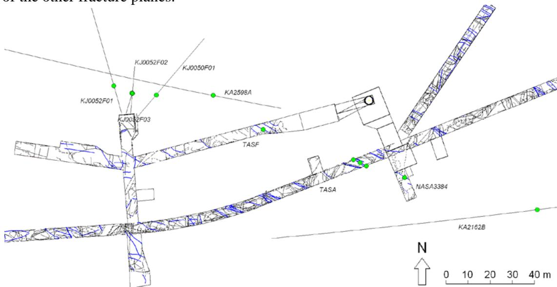
**Figure A 7.** Observation points used to model FASEW002c in tunnels and boreholes.
