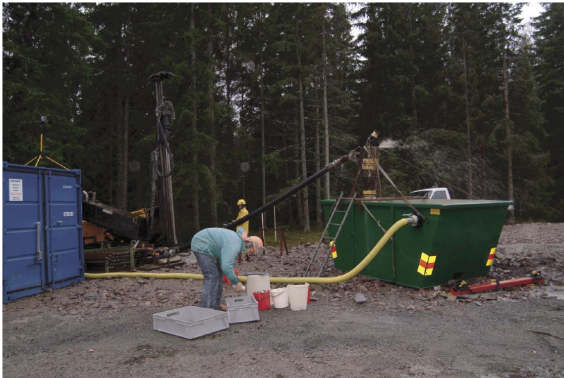
Figure 4-2. Sampling of drill cuttings from the penetrated bedrock.
