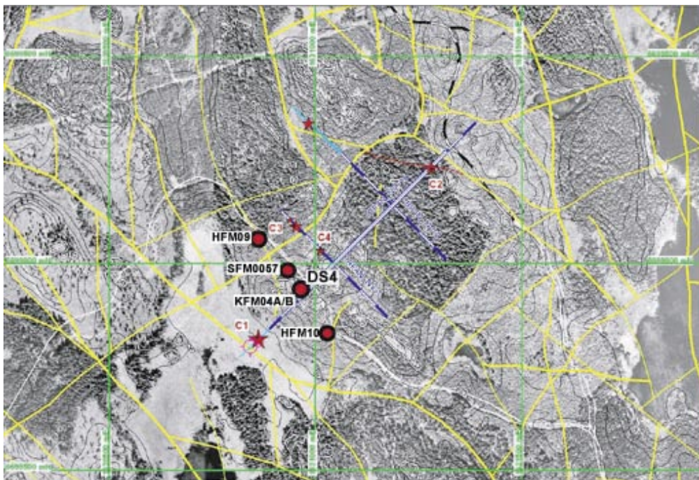
Figure 2-1. Lineaments (yellow), geophysical survey lines (blue), EM conductors (red stars) and boreholes (red dots) at drilling site DS4. Tommy Karlberg after Pitkänen and Isaksson /4/.
