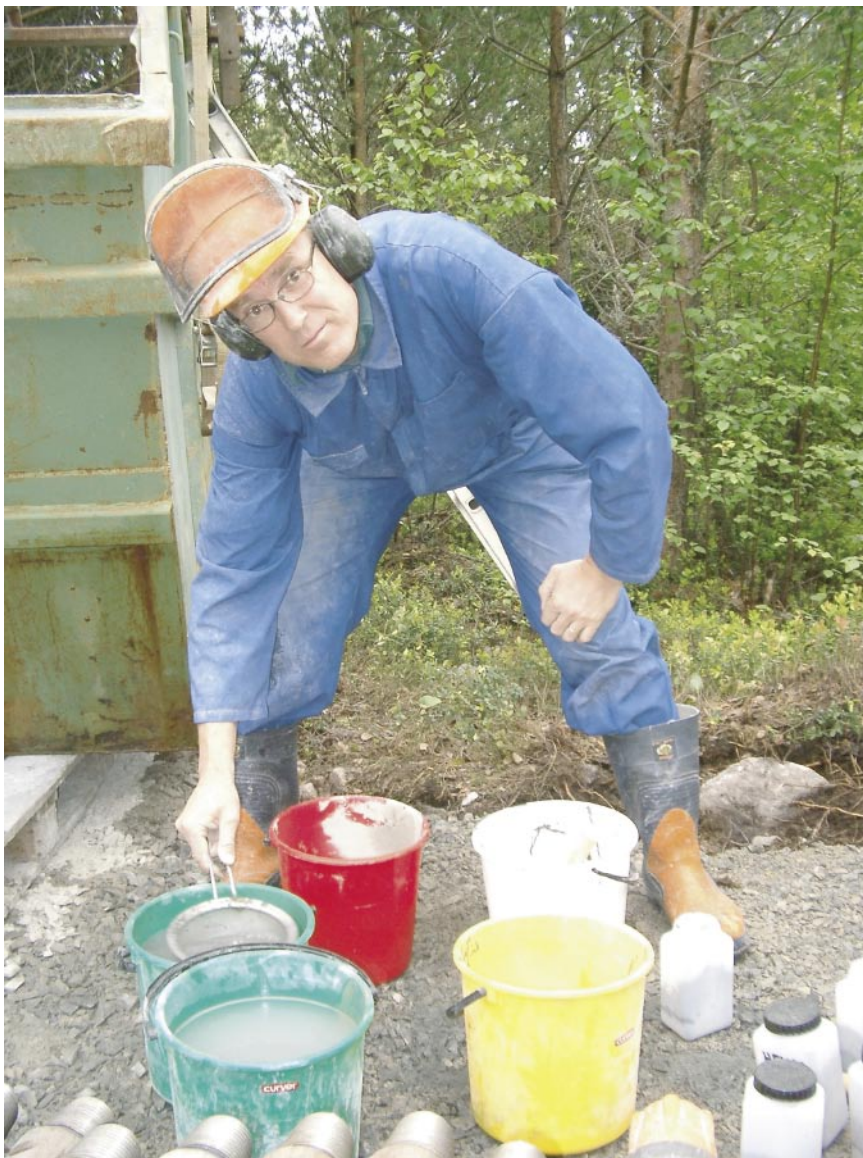
Figure 4-2. Sampling of one sample per 3 m drilling length of drill cuttings from the bedrock.
