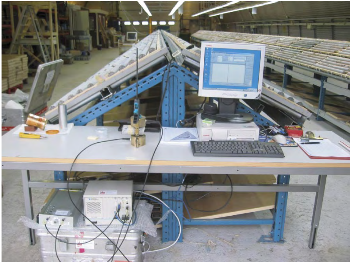
Figure 3-1. NGI's equipment set-up for measuring acoustic P-wave travel time transverse borehole core.
