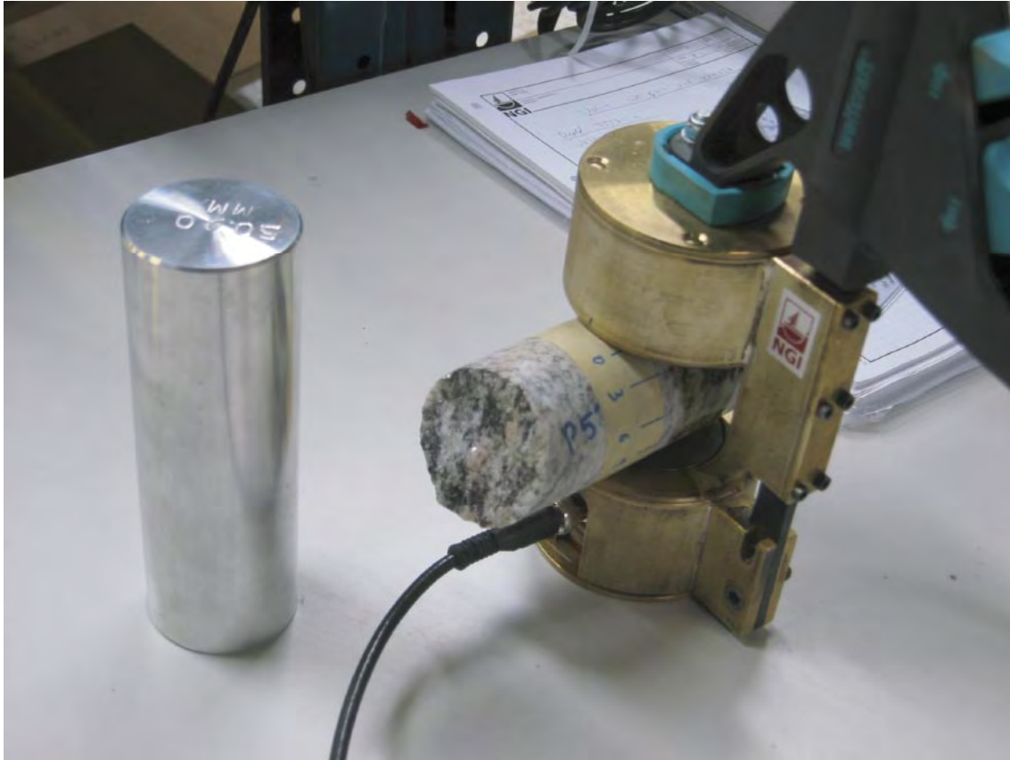
Figure 3-2. Detail of NGI's apparatus for measuring acoustic P-wave travel time transverse borehole core. The aluminium cylinder for calibration of the device is on the left.
