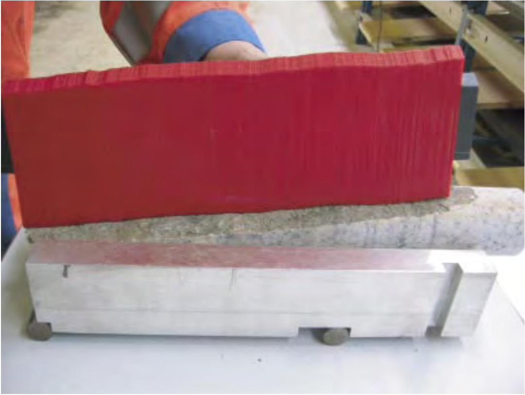
Figure 3-3. Profilometer applied on a joint surface.
