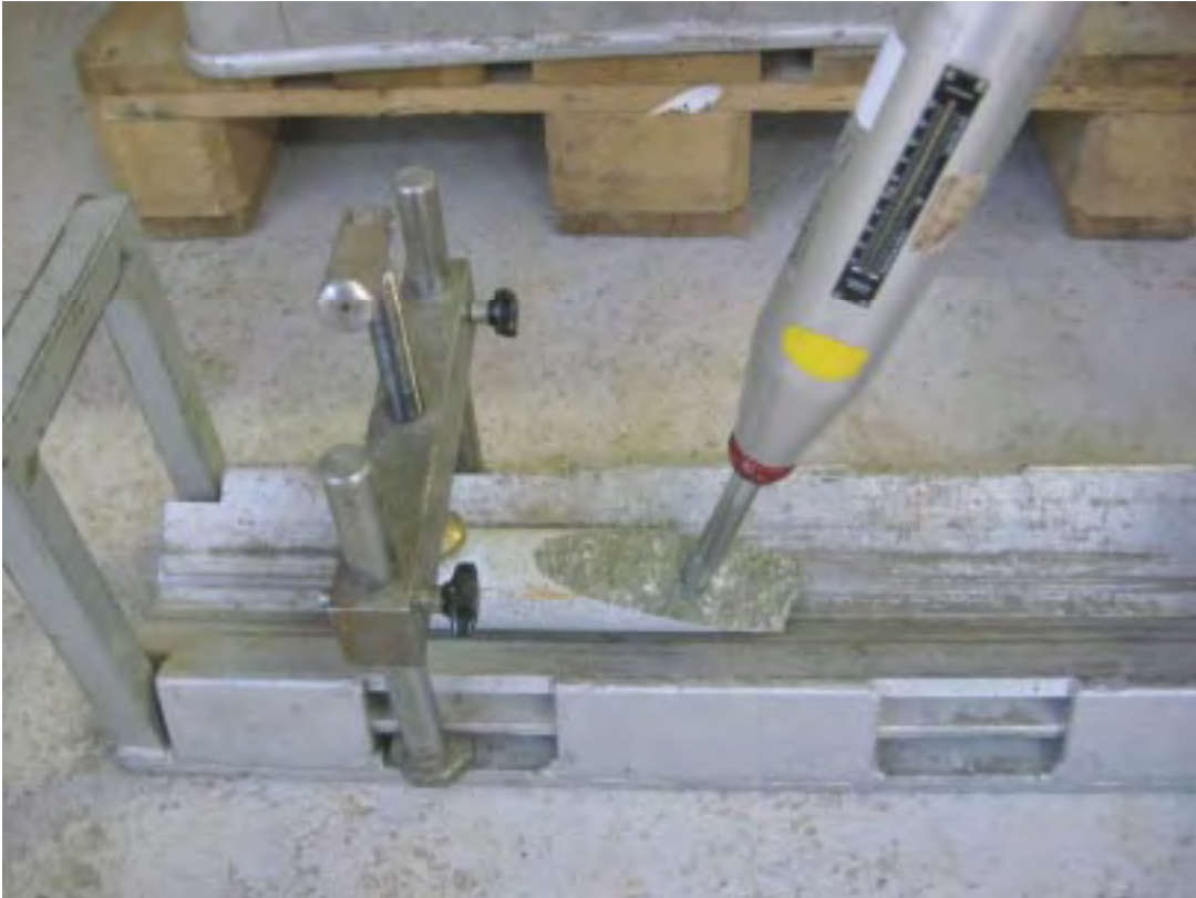
Figure 3-2. Clamp for the Schmidt hammer tests.
