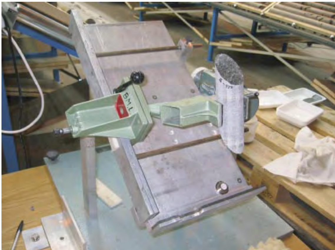
Figure 3-1. NGI's Tilt test apparatus.
