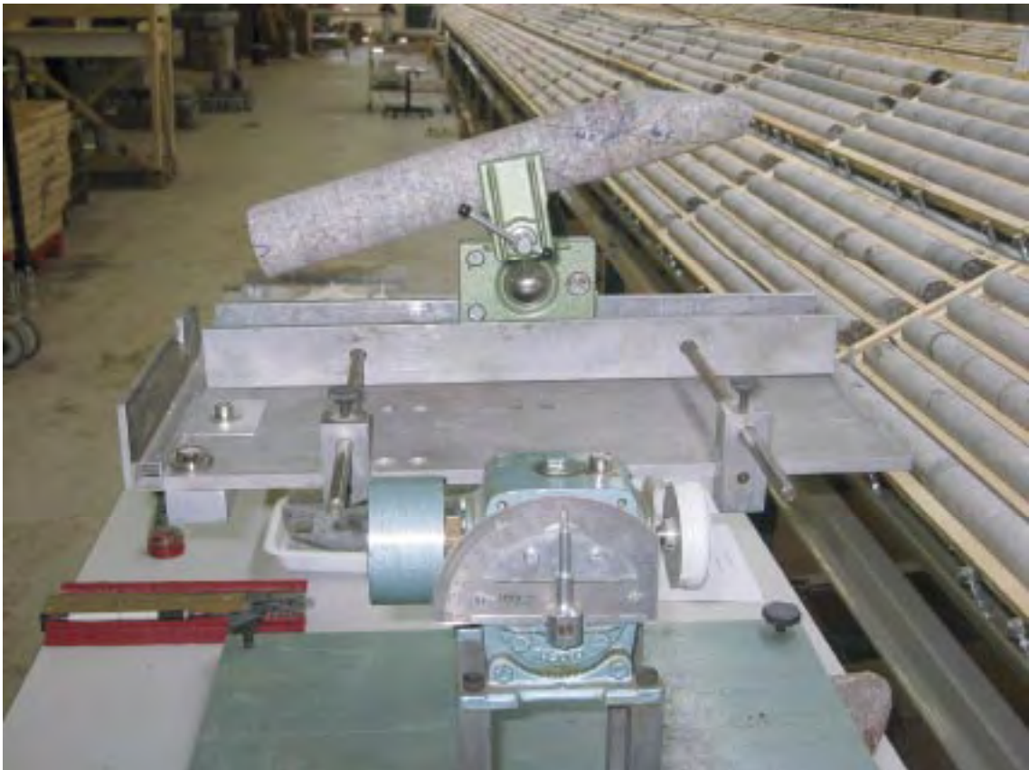
Figure 4-1. Sample for tilt testing in the tilt apparatus.
