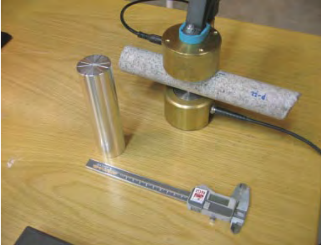
Figure 3-2. Detail of NGI's apparatus for measuring acoustic P-wave travel time transverse borehole core. The aluminium cylinder for calibration of the device is on the left.
