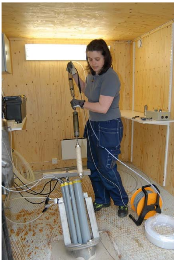
Figure 3-1. Lowering of sampling equipment in the wide diameter water stand pipe in order to pump water from the connected borehole section. From the bottom; filters, small inflatable packer and pump.
