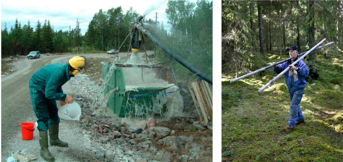
Figure 2-2. Two key features of the bedrock in the target area at Forsmark. Left: High water yields are often observed in the uppermost c. 150 m of the bedrock. Right: The large number of unbroken drill cores gathered at depth support the observation of few flowing test sections in the deeper bedrock. (Figure 10-1 in /Follin 2008/.)
