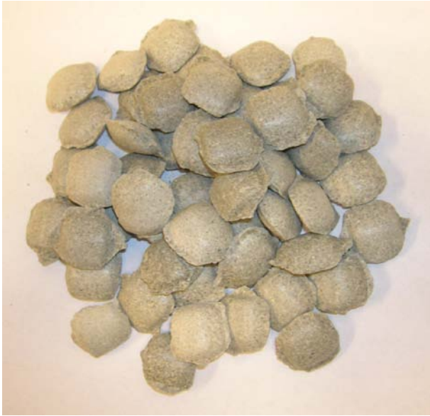
Figure 5-11. Pellets made by the briquette pressing machine used for the Prototype Repository.
