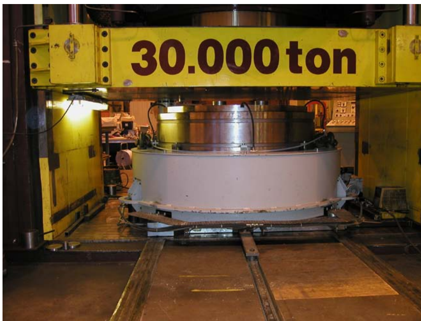
Figure 5-7. The mould used for making ring shaped blocks for the Prototype Repository.
