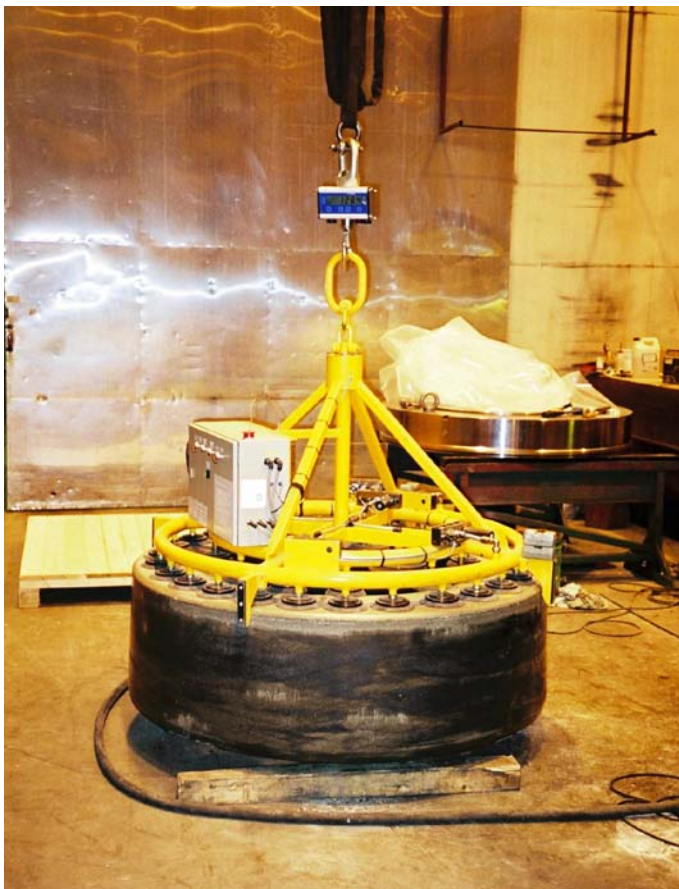
Figure 5-8. A bentonite block lifted with the vacuum oak used at the production of the blocks of the Prototype Repository. Note the weighing machine hanging in the over head crane.
